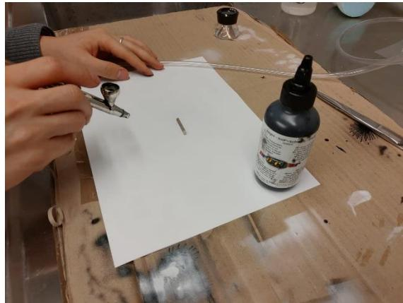
**Figure 4.6.** Deposition of the black ink on the sample with an air mini paint spray gun.
