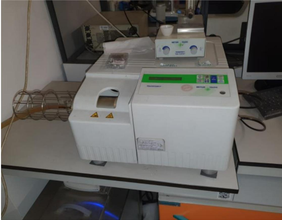
Figura 3.16: TGA Mettler Toledo
