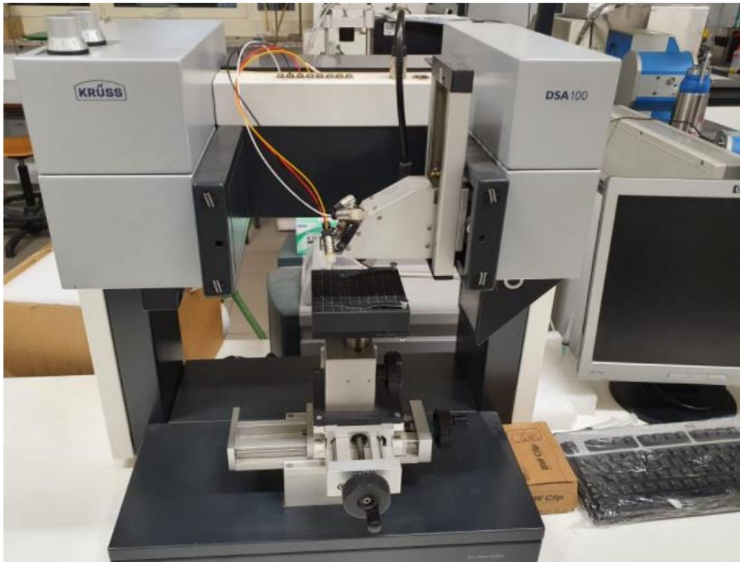
*Figura 3.20: Drop Shape Analyzer (DSA) 100 Kruss*
