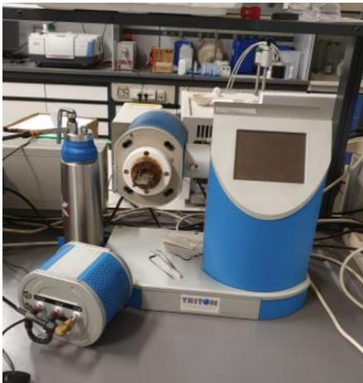
Figura 3.17: TTDMA Triton TechnologyMettler Toledo
