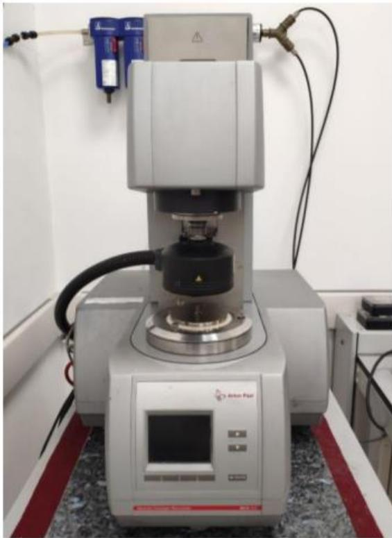
Figura 3.13: reometro Anton Paar MCR 302 <sup>47</sup>
