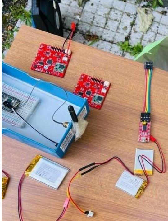
Figure 6.11: The two PCB and batteries used for the experiment.
