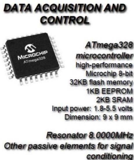
*Figure 4.6: ATmega 328 microcontroller*
