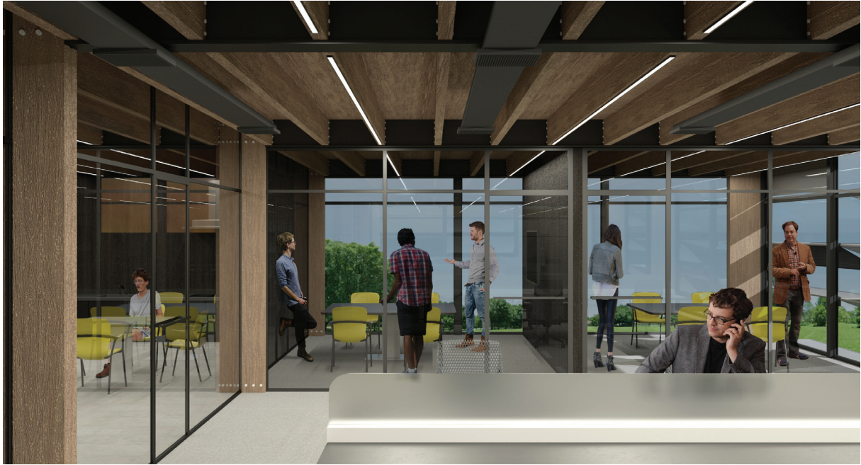
Render 03. A view from the co-working office. All the structural and mechanical elements are exposed to increase flexibility and reduce construction costs.
