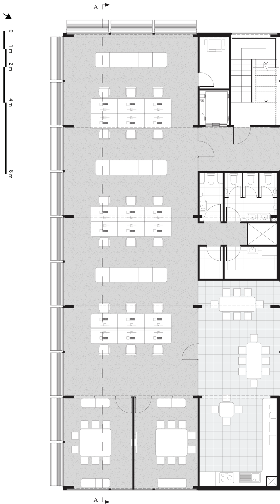
Drawing 03. First floor plan. The plan is modifiable as there are no fixed walls. All the piping systems are also exposed and located on the roof. This flexibility ensures a future-proof design.
