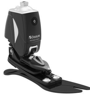
(b) PROPRIO FOOT by Ossur, adaptive microprocessor controlled ankle
