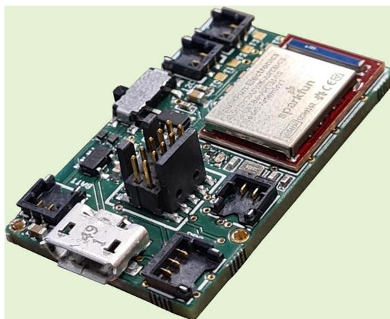
Figure 2.6: Wireless ATC acquisition device [59].
