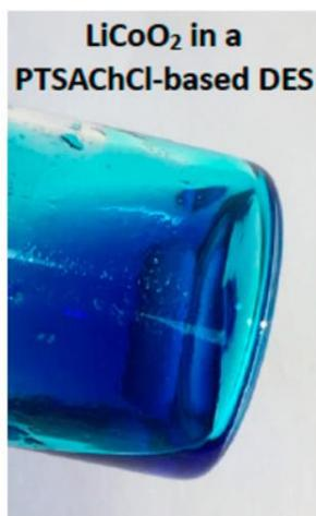
Figure 18. Solution obtained after dissolving  $\text{LiCoO}_2$  in the  $\text{PTSA}:\text{H}_2\text{O}:\text{ChCl}$  DES
