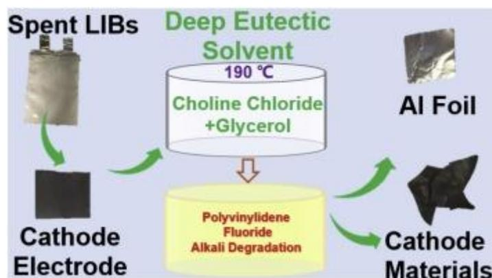
Figure 16. Schematic representation of the aluminium foil and cathode material DES-based separation process.
