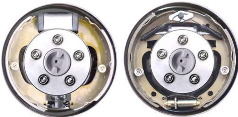
Figure 2.2: Leading/trailing shoes on left, duo-servo on right
