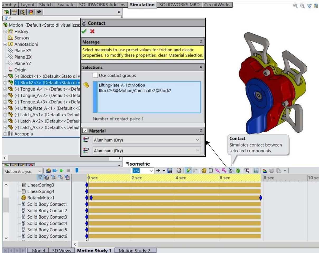
Figure 5.2.4 – Dashboard of the body contact.
