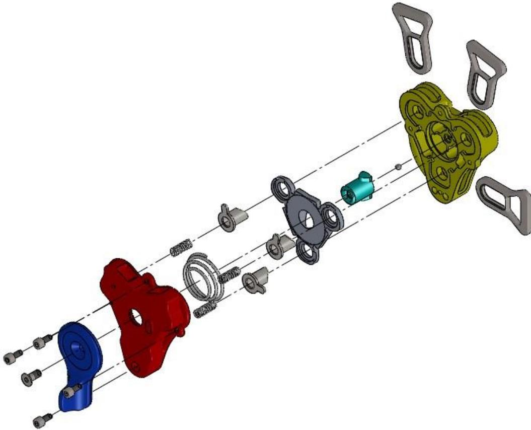
Figure 2.2.1 – Super light buckle explosion.
