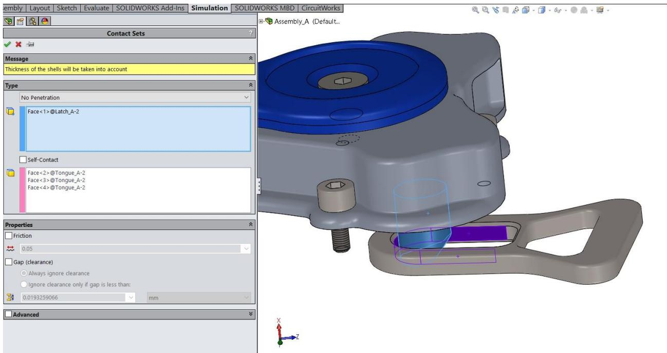
Figure 4.4.5.2.2 – Command to set the contact between two parts.
