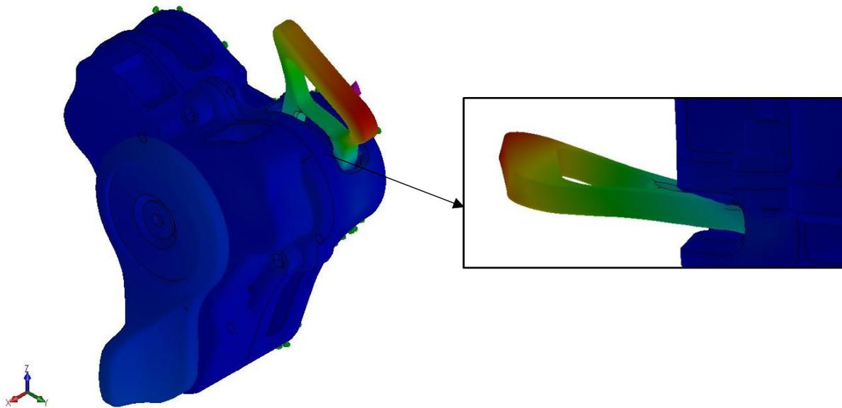
Figure 4.4.5.2.12 – Simulation adding the contact between the sphere and his housing on the lower body.
