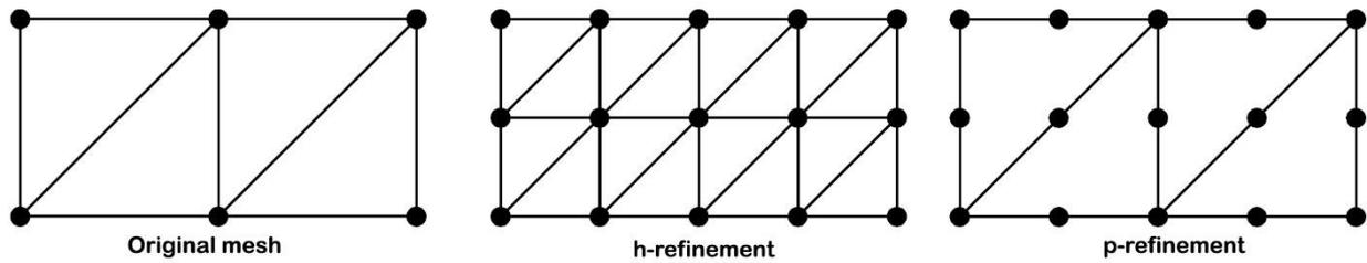
Figure 4.4.4.1.2 – h-method and p-method, shown through a simple scheme of 2D mesh elements.
