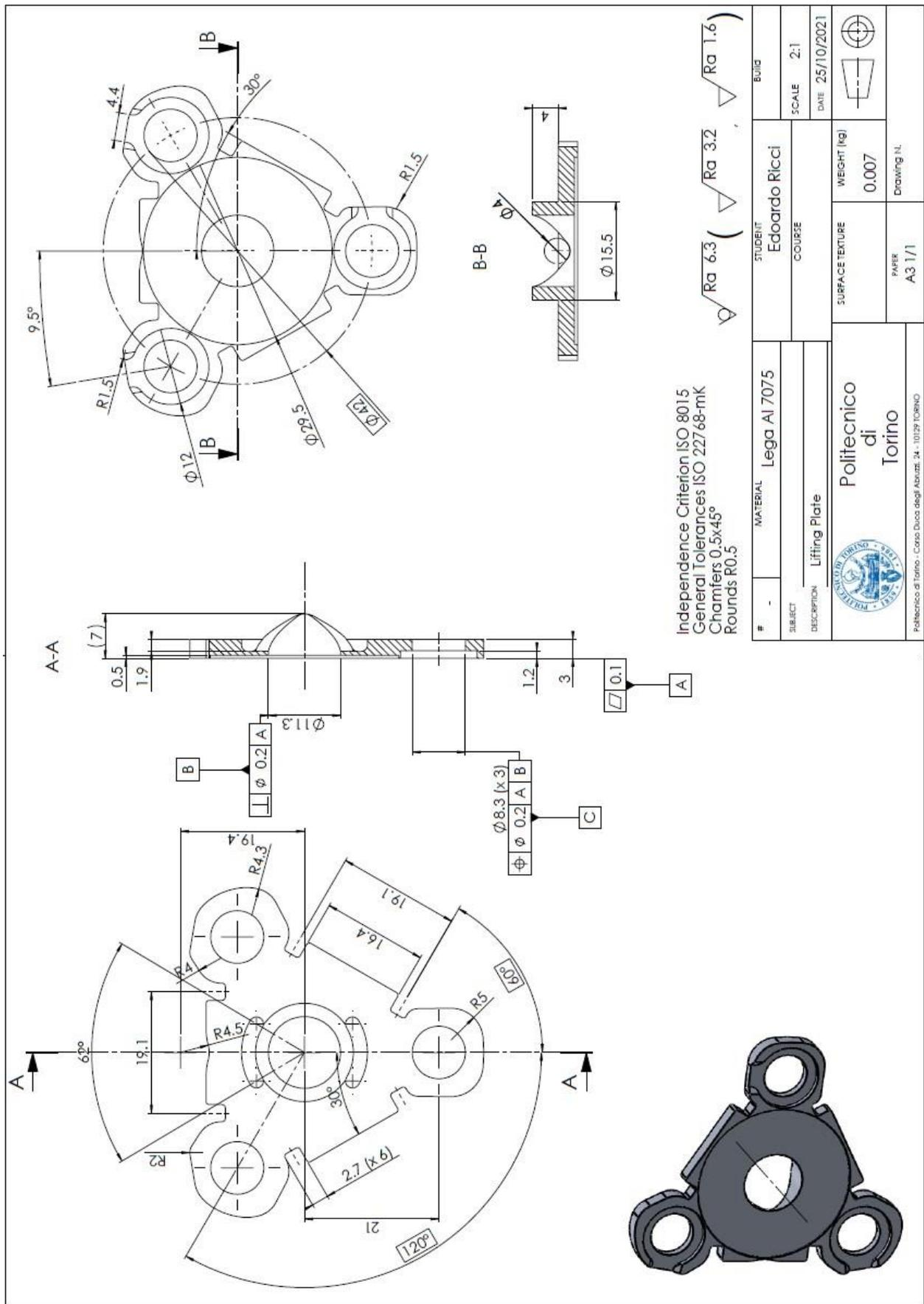
Figure A-6 – Lifting plate.
