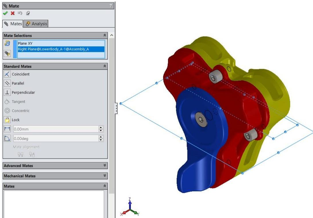
Figure 2.4.2 – Example of mate to set the reference system.
