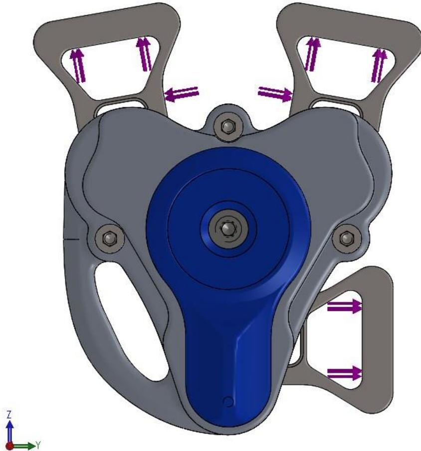
Figure 4.5.3.2 – Representation of the forces which act on the buckle.
