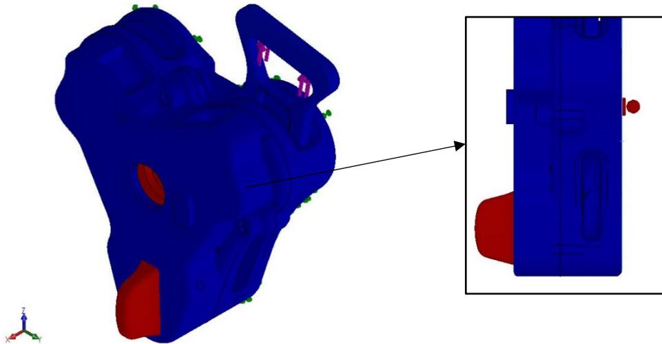
Figure 4.4.5.2.11 – Simulation adding the contact between the camshaft and the sphere.
