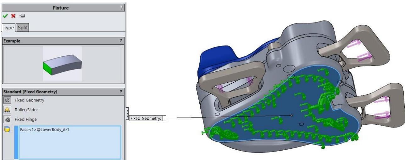
Figure 4.4.2.2 – Example of standard fixture.
