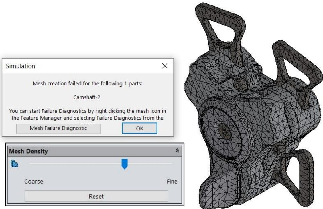
Figure 4.5.5.2 – Mesh got with a medium mesh density.
