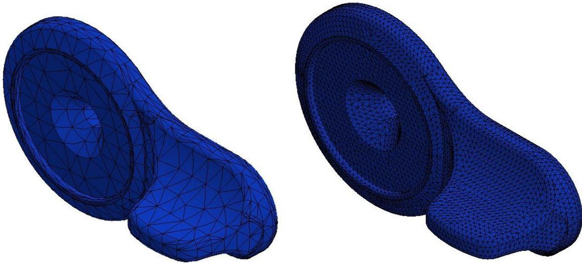
Figure 4.4.4.1.4 – Coarse density at left, fine density at right.
