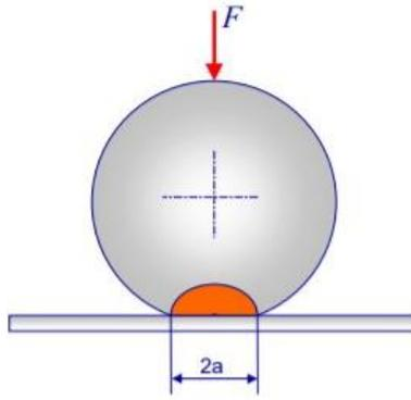
Figure 2.6.3 – Example of contact between a sphere and a plane.
