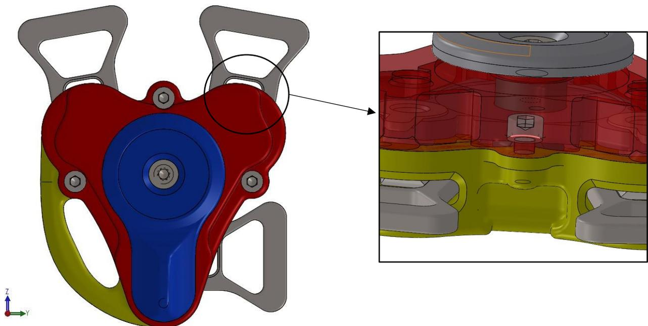
Figure 3.1.2 – Zoom of the interference between the head of the screws and the lower body.
