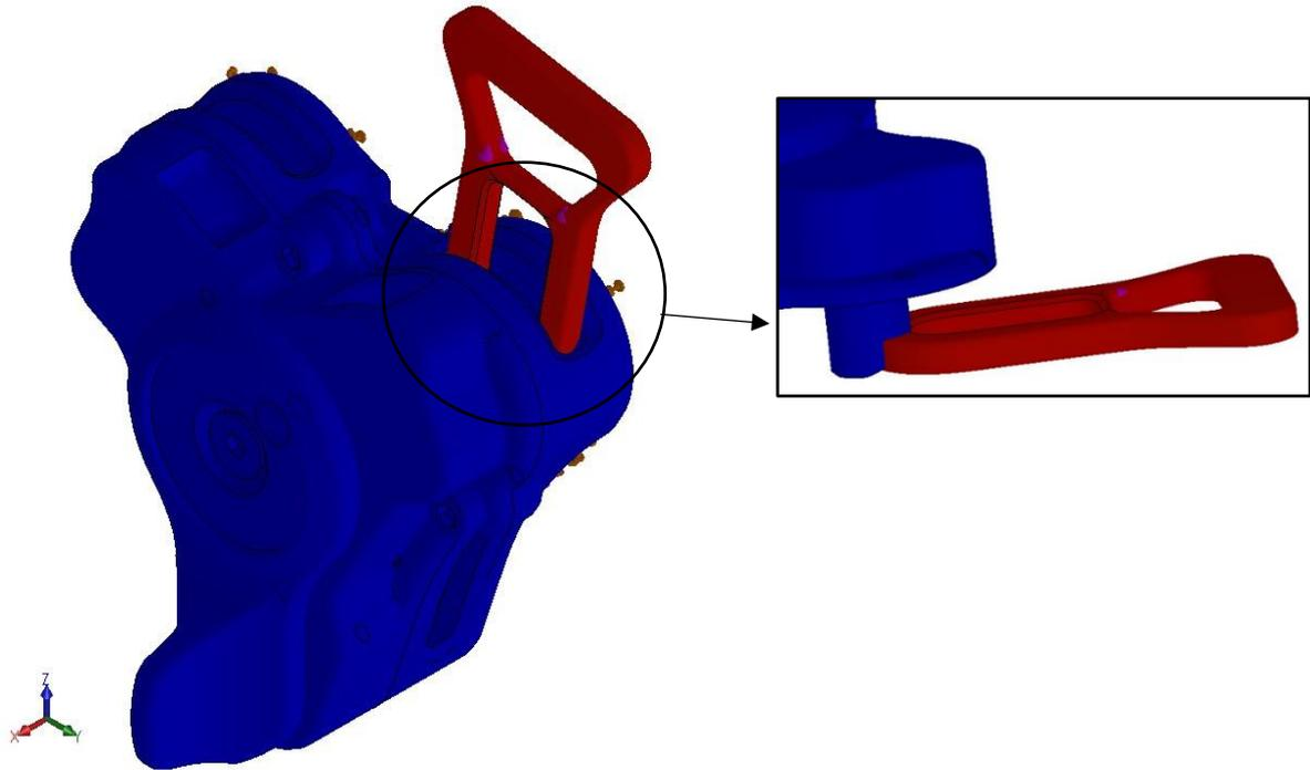
Figure 4.4.5.2.3 – Simulation without any contact set and the zoom of the interference.
