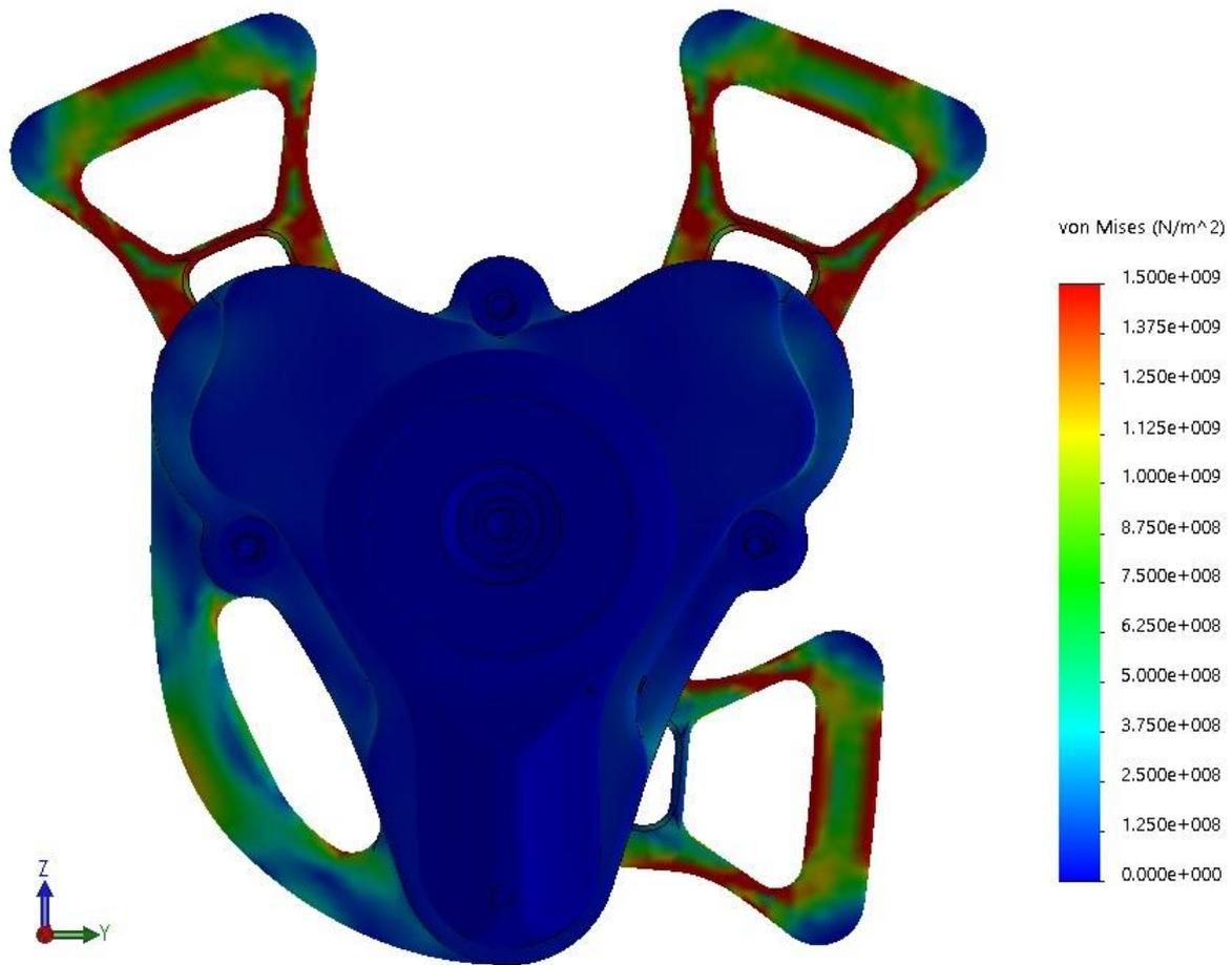
Figure 4.5.6.1 – Stress result on the super light buckle.
