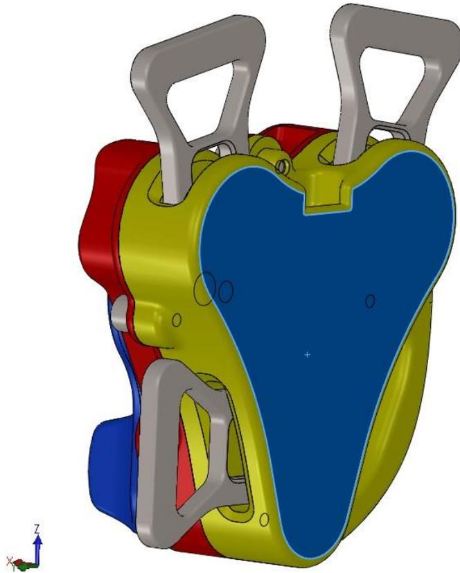
Figure 2.5.2 – Contact area between the buckle and the body of the driver.
