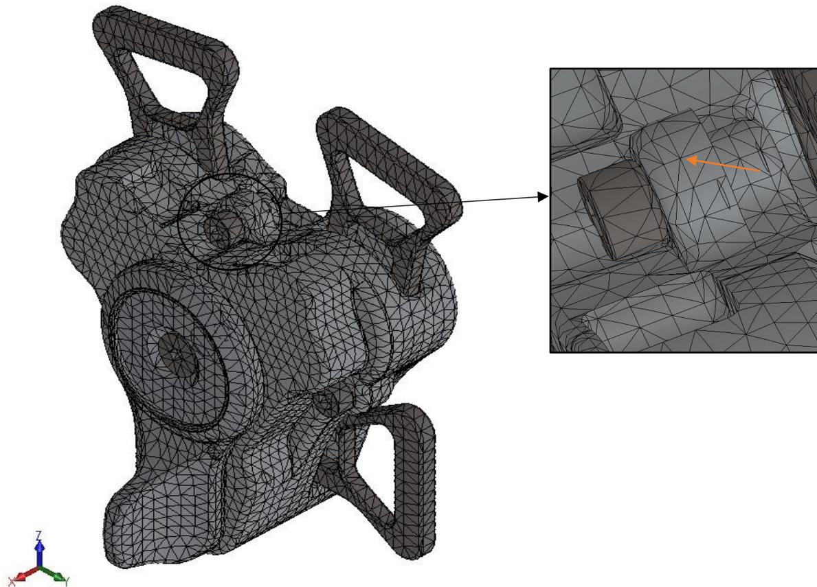
Figure 4.4.4.1.10 – Zoom of lower and upper body contact to show the meaning of compatible mesh.
