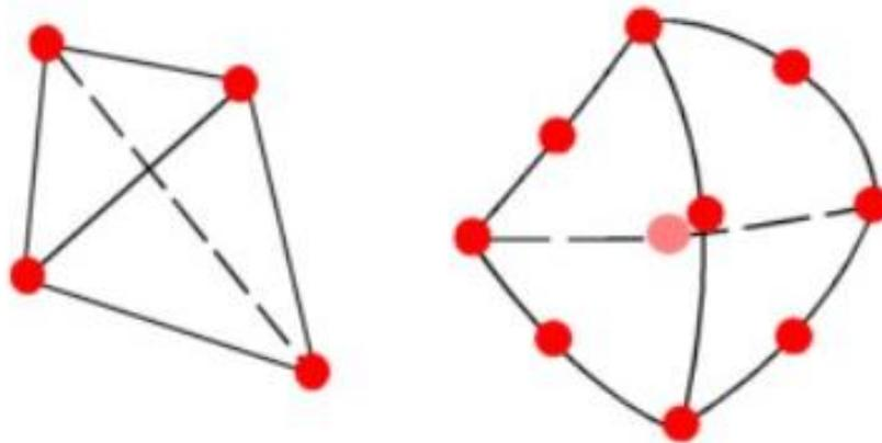
Figure 4.4.4.1.1 – Linear elements on the left, parabolic elements on the right.
