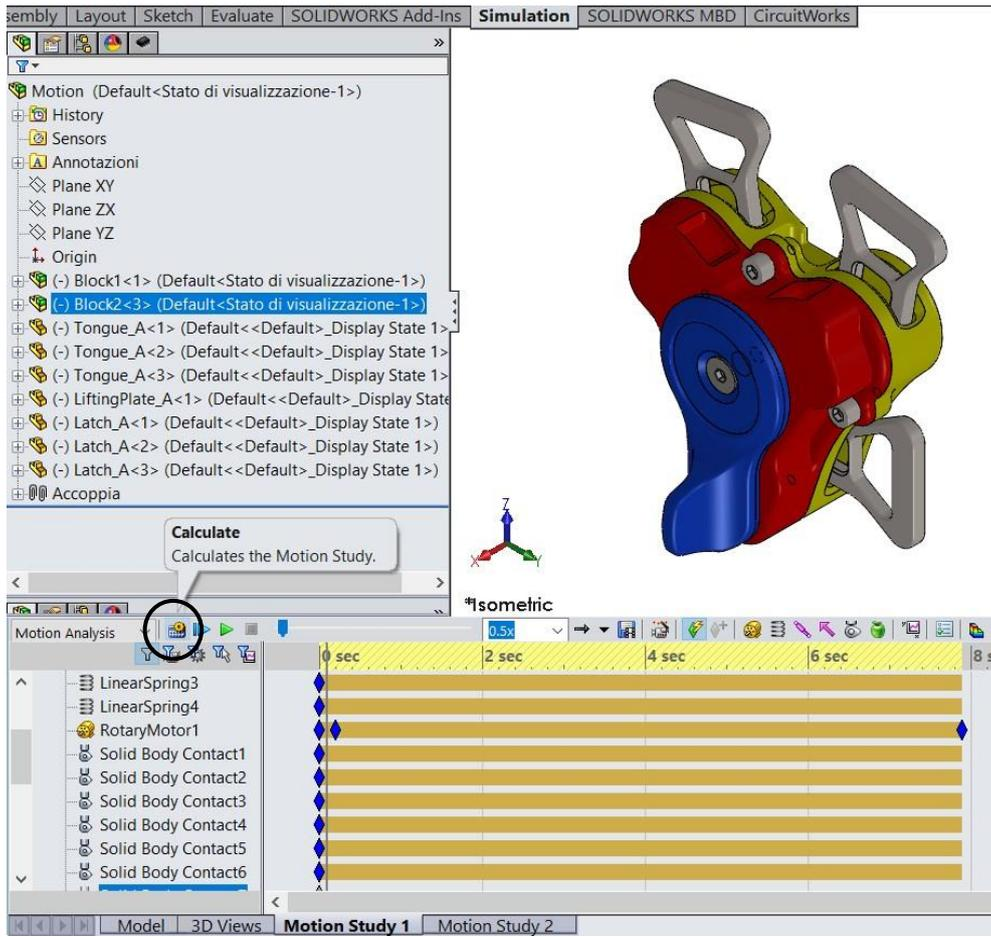
Figure 5.3.1 – Tool to calculate the Motion Analysis.
