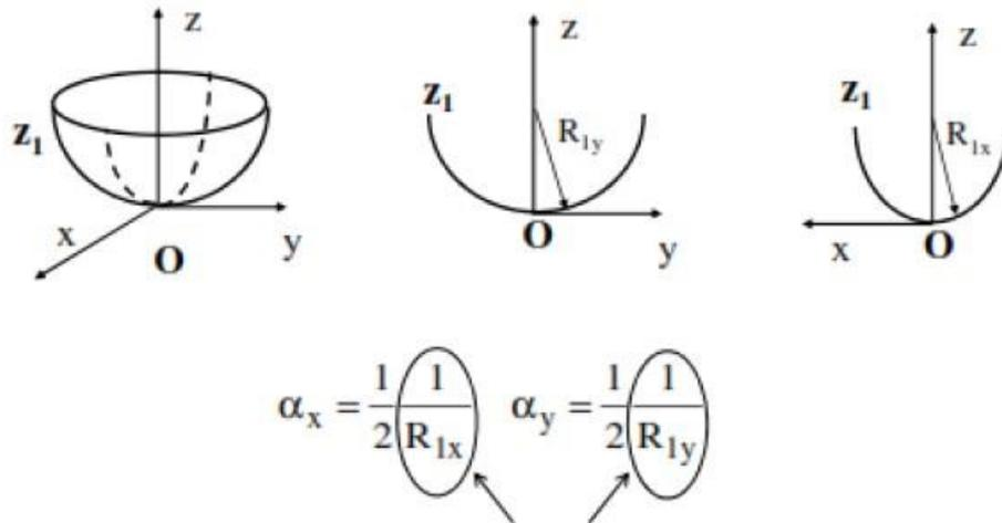
Figure 2.6.1 – Example of the principal curvatures for a generic body.
