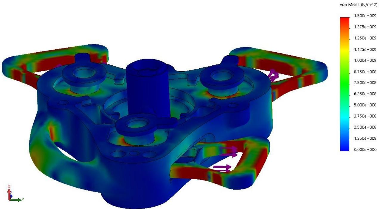
Figure 4.5.6.2 – Stress result on the super light buckle, hiding the upper body.
