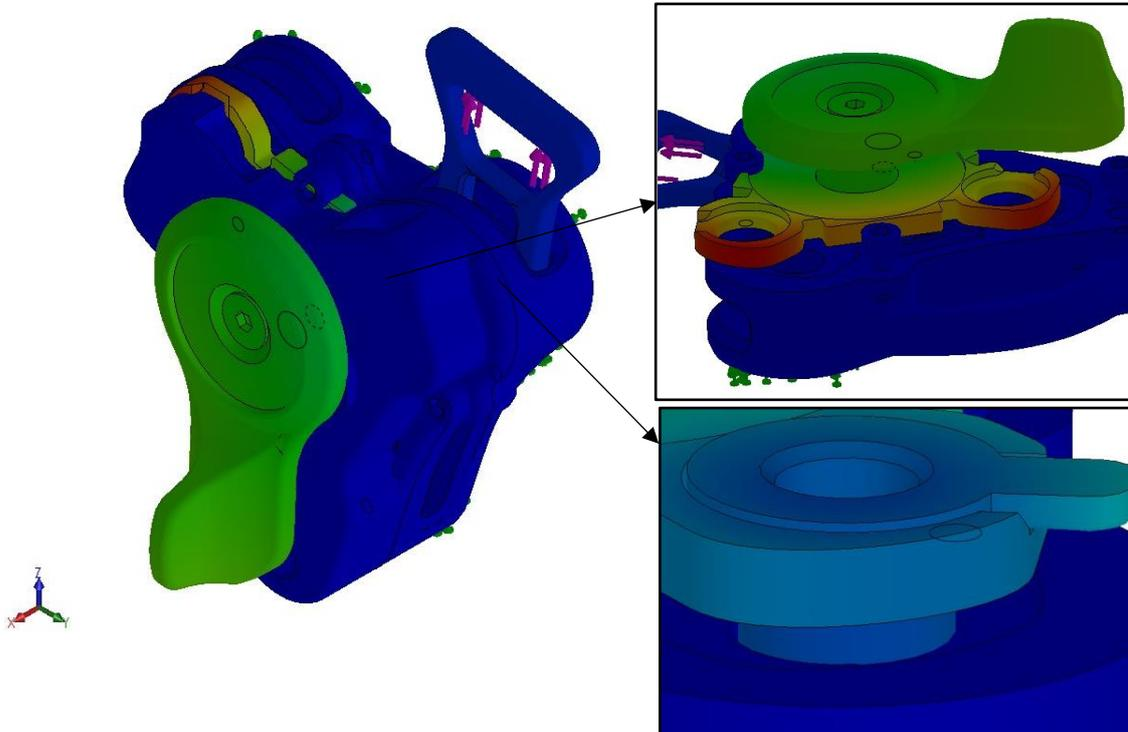
Figure 4.4.5.2.7 – Simulation adding the contact between lifting plate and lower body.
