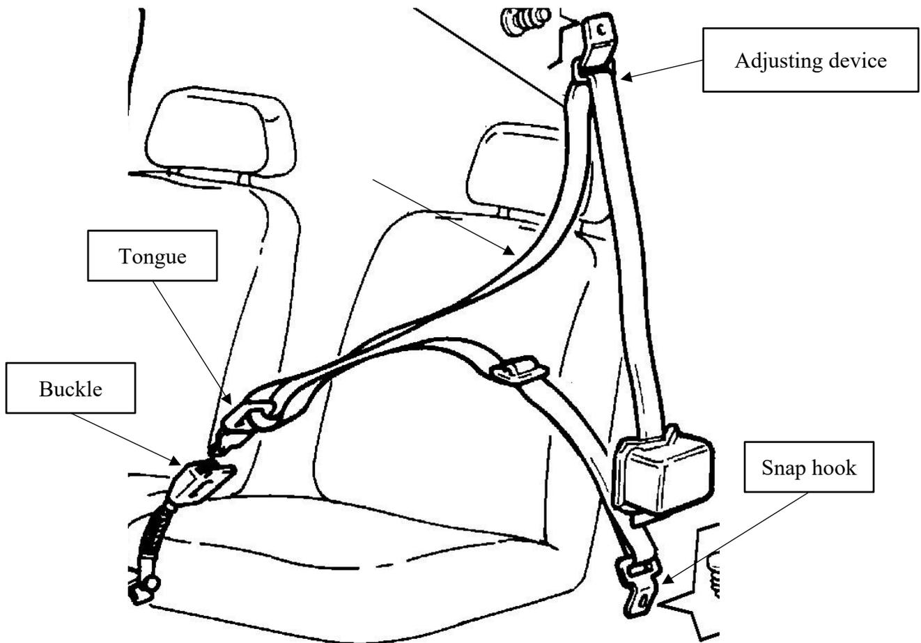
Figure 1.1 – Schematic representation of a commercial car harness.
