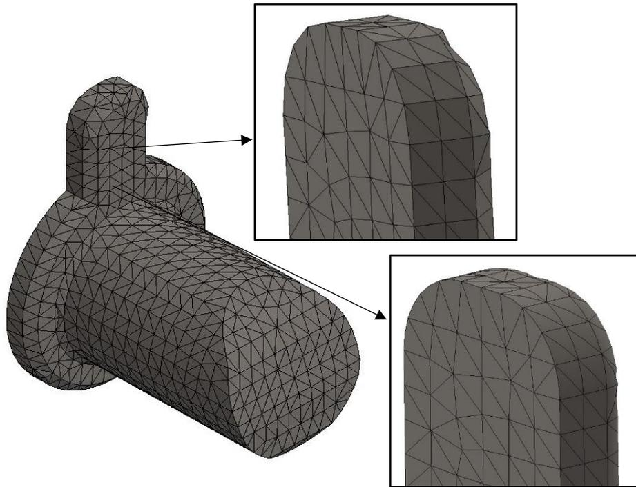
Figure 4.4.4.1.8 – Latch mesh to show the difference between Tetra4, on bottom, and Tetra4, on top.
