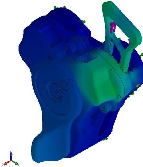
Figure 4.4.5.2.13 – Simulation adding the contact between the upper and the lower surface of the tongue and the lower body.
