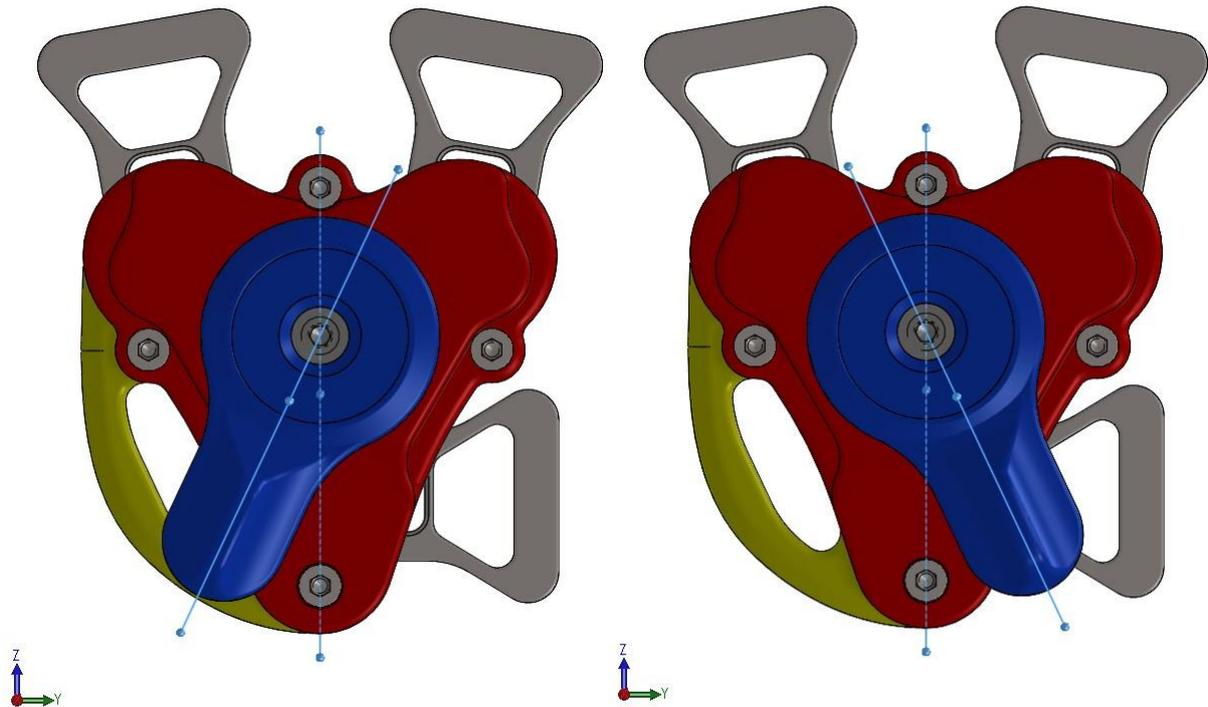
Figure 2.5.1 – Pre-release free movement, 25° each side.
