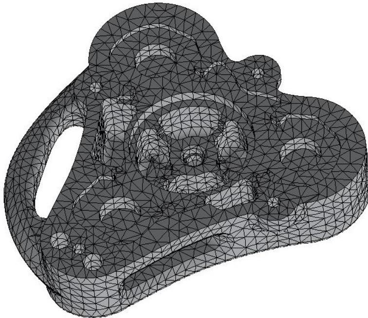
Figure 4.4.4.1 – Example of mesh, using the lower body as sample.
