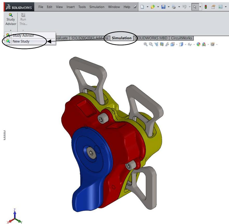
Figure 4.4.1 – Command to start a new study in Simulation.
