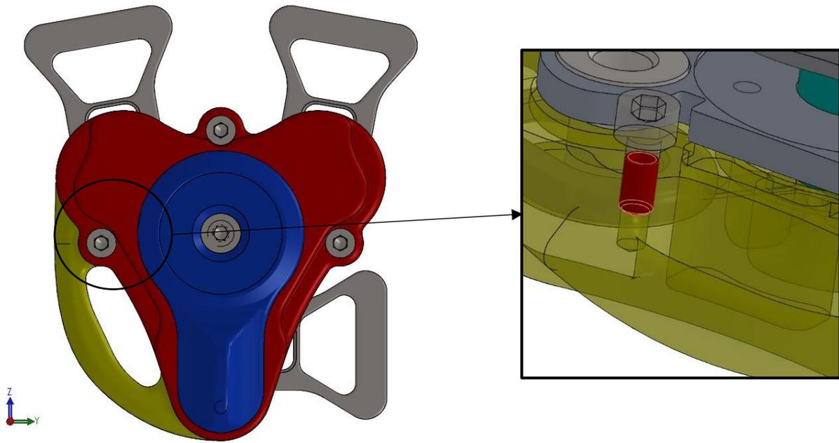
Figure 3.1.1 – Zoom of the interference between the thread of the screws and the lower body.
