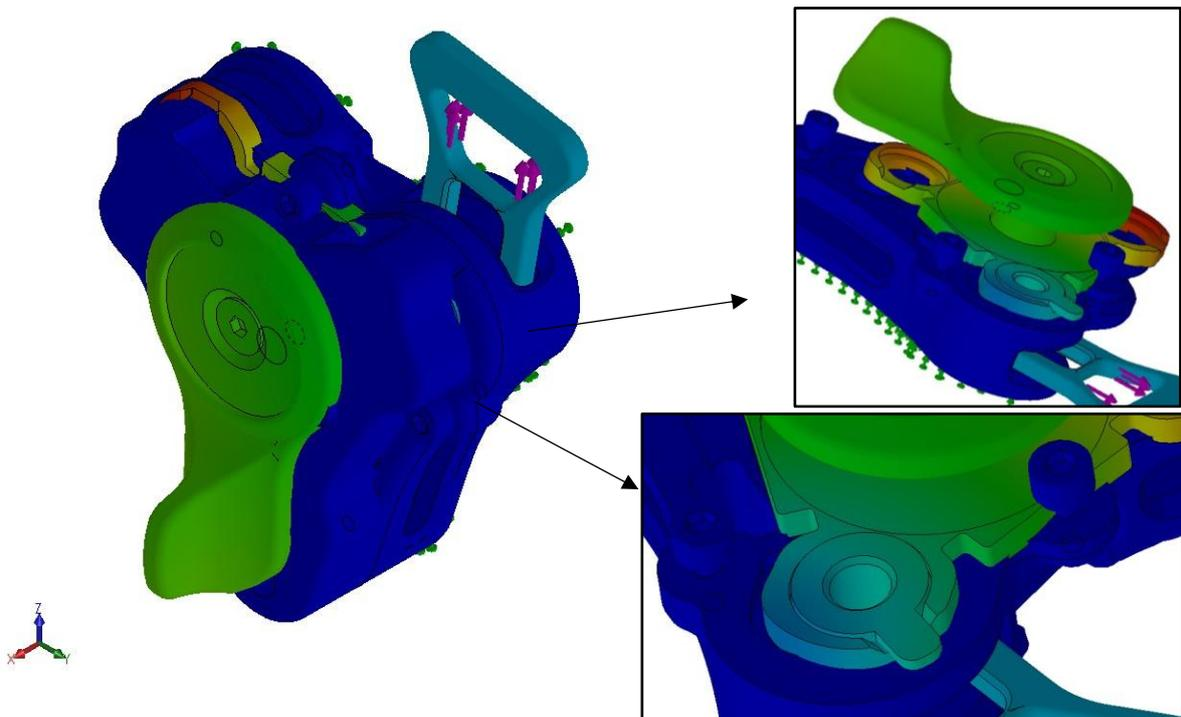
Figure 4.4.5.2.6 – Simulation adding the contact between lifting plate and camshaft.
