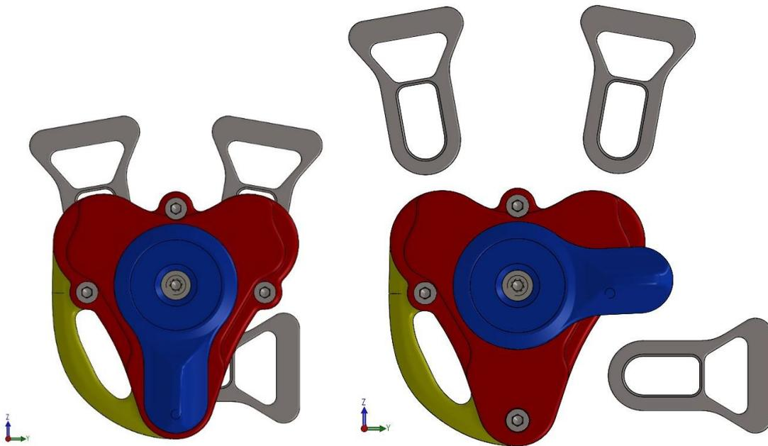
Figure 1.2.1 – Super light buckle in Solidworks: buckled position on left; unbuckled position on right.
