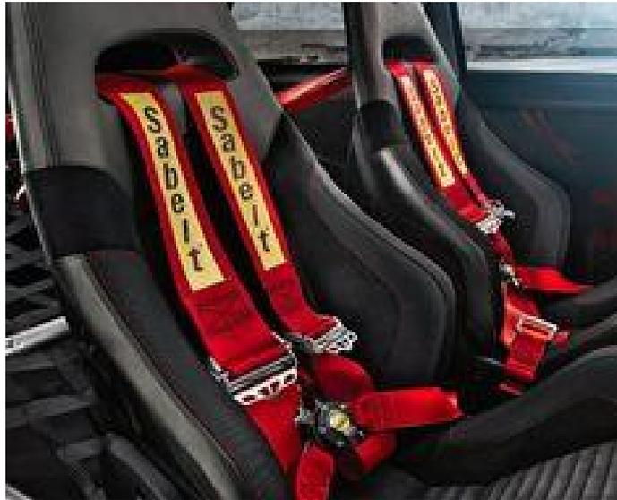
Figure 1.2 – Example of harness with 6 attachment points.
