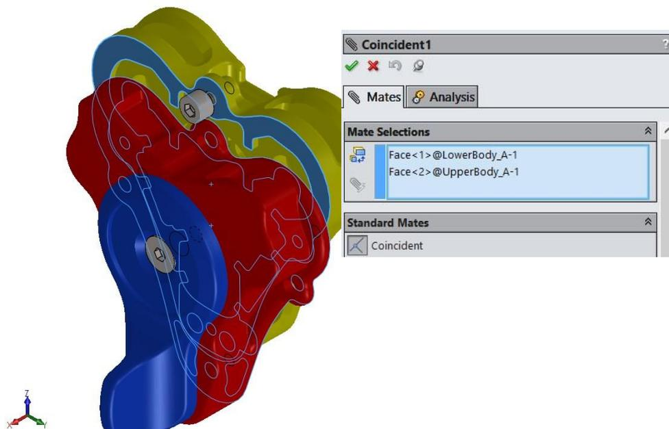
Figure 2.4.3 – First mate to lock upper body in relation to lower body.
