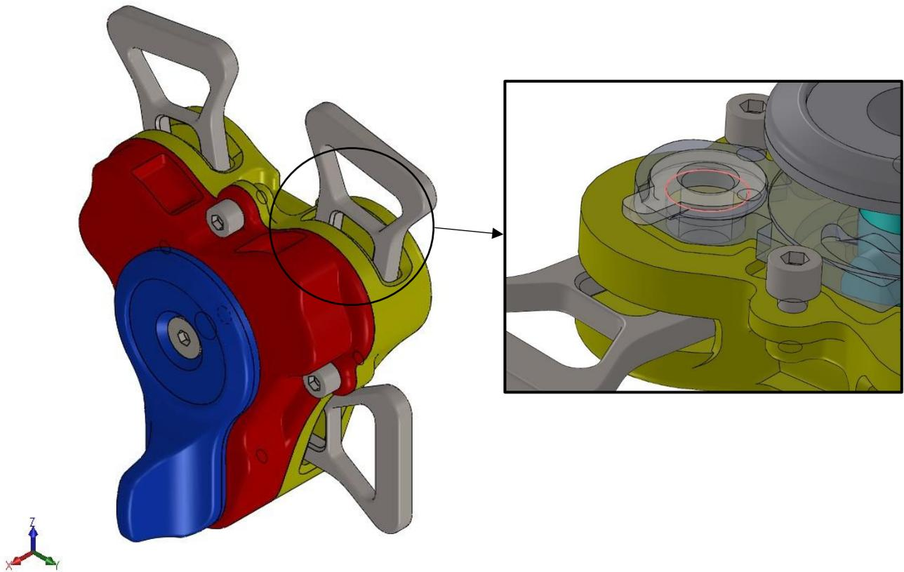
Figure 3.3.1 – Zoom of the interference between a latch and the lifting plate.
