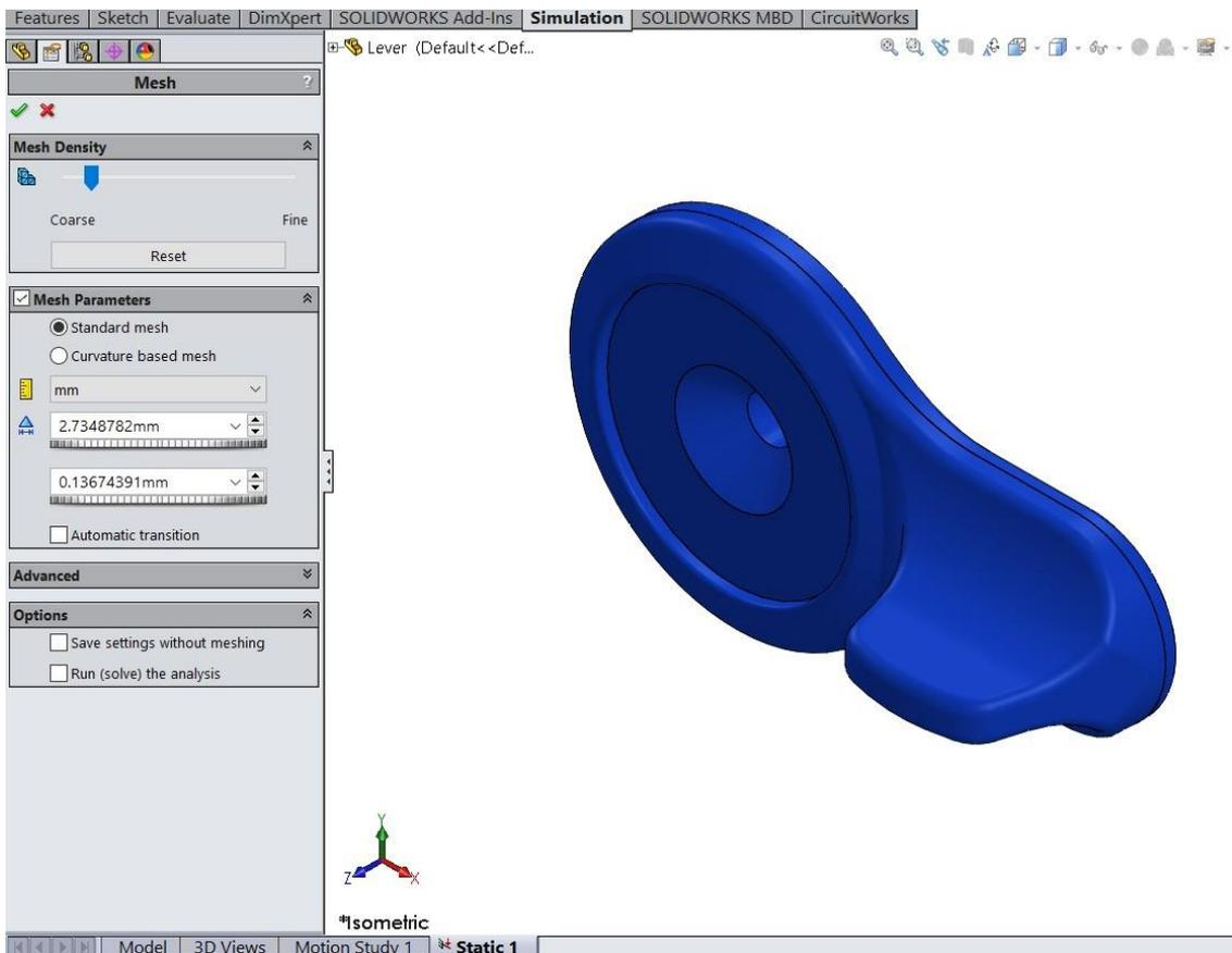
Figure 4.4.4.1.3 – Mesh density dashboard.
