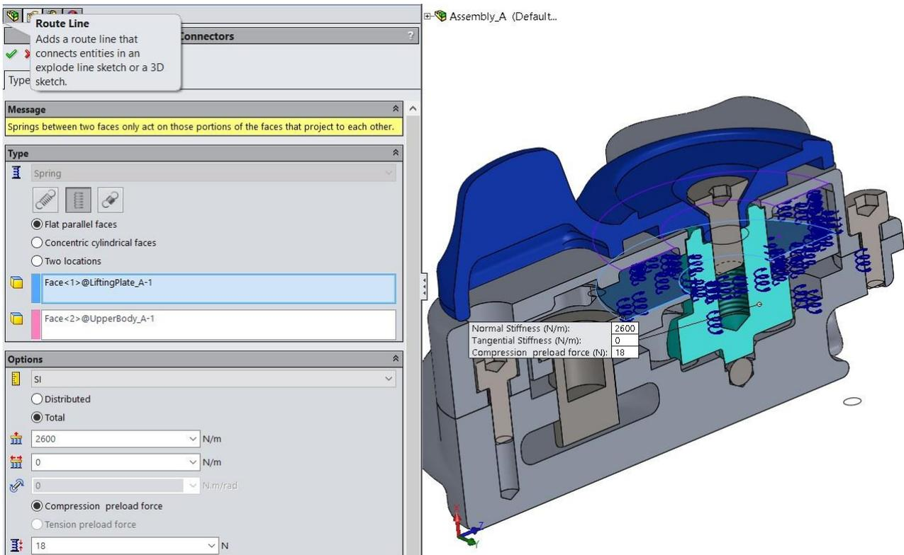
Figure 4.4.5.3.2 – Setup of the spring connector dashboard.
