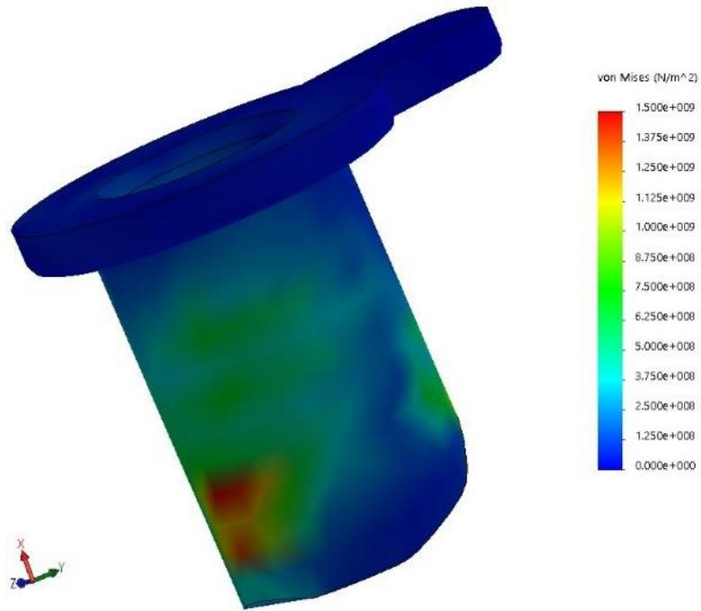
Figure 4.5.6.4 – Stress result on one latch.
