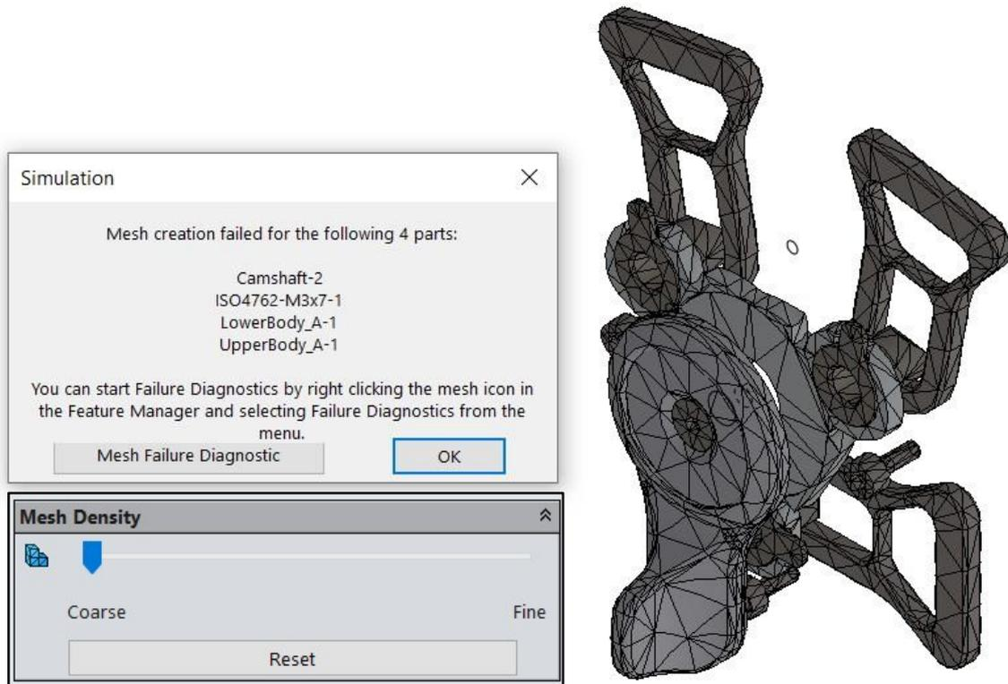
Figure 4.5.5.1 – Mesh got with a coarse mesh density.
