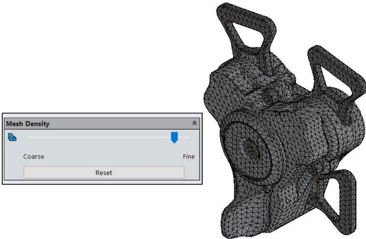
Figure 4.5.5.3 – Mesh got with a fine mesh density.
