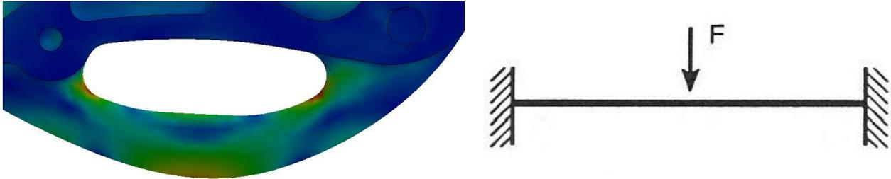
Figure 4.5.6.6 – Stress distribution on the fixed tongue on left and his hyperstatic scheme on right.
