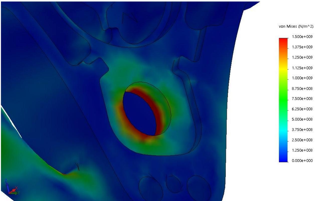
Figure 4.5.6.5 – Stress result on the lower body caused by one tongue.
