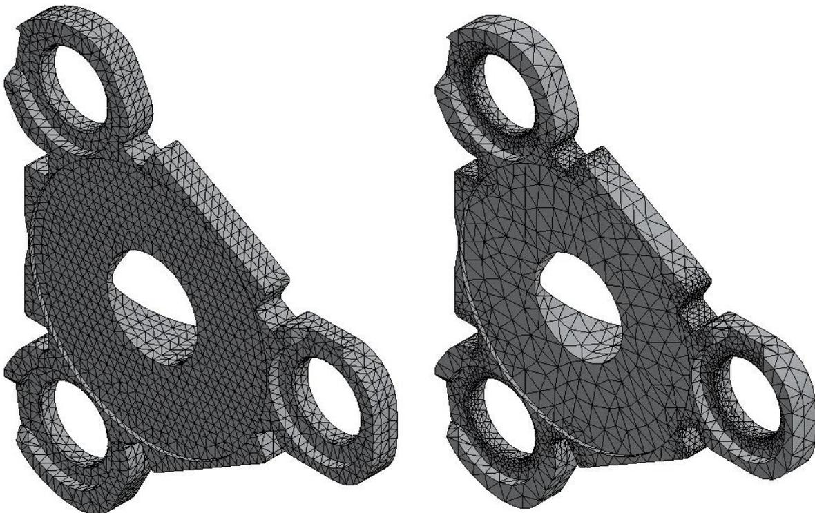
Figure 4.4.4.1.9 – Standard mesh on left, curvature-based mesh on right.
