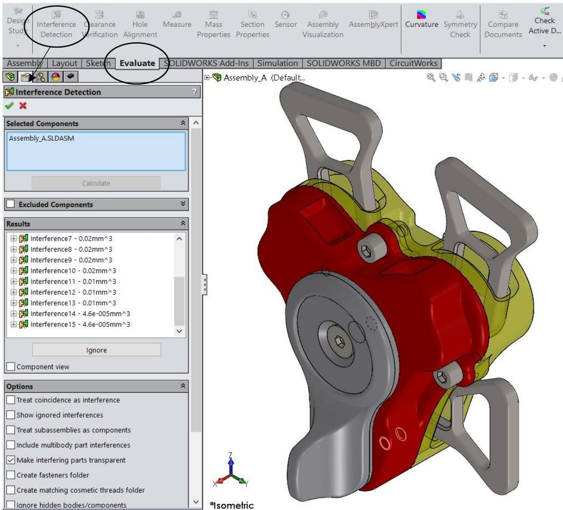
Figure 3.1 – Detection of the interferences among buckle parts from the model A in Solidworks.
