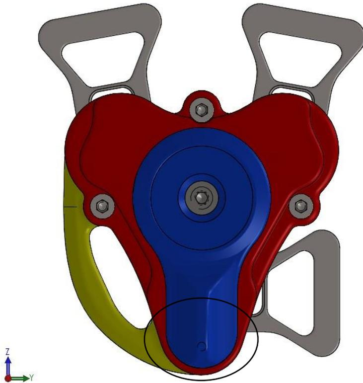
Figure 2.5.3 – Upper body covers the entire projected surface of the lever.
