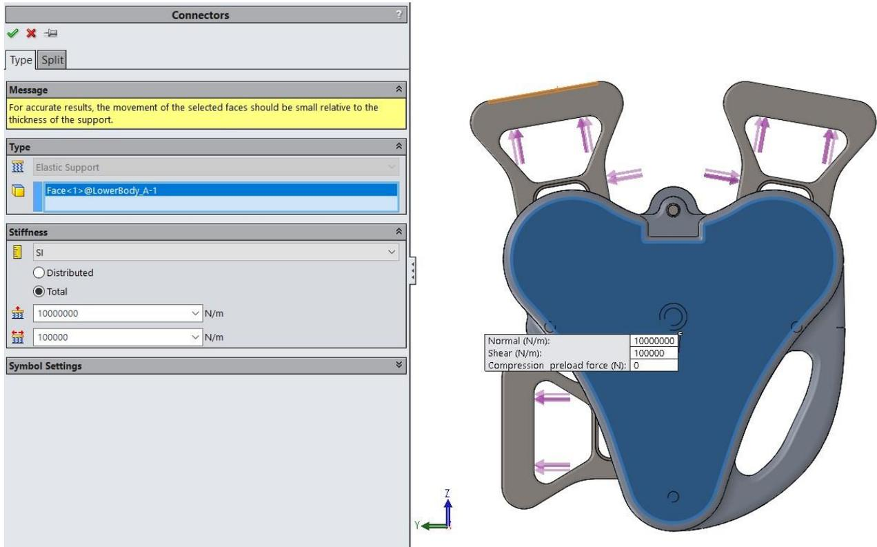
Figure 4.4.2.3 – Example of elastic support.
