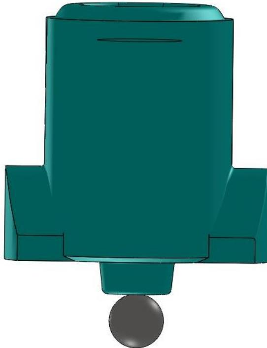
Figure 2.6.4 – Contact between the sphere and camshaft.
