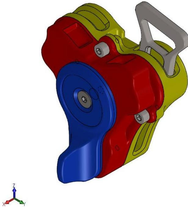
Figure 4.4.5.2.1 – Buckle without two latches and two tongues.
