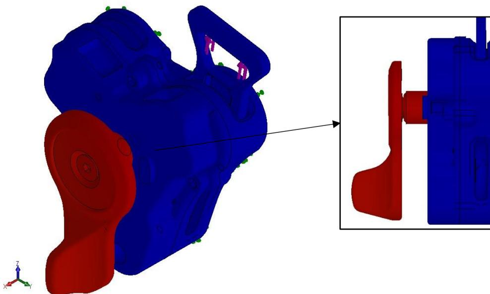
Figure 4.4.5.2.8 – Simulation adding the contact between lifting plate and lower body.
