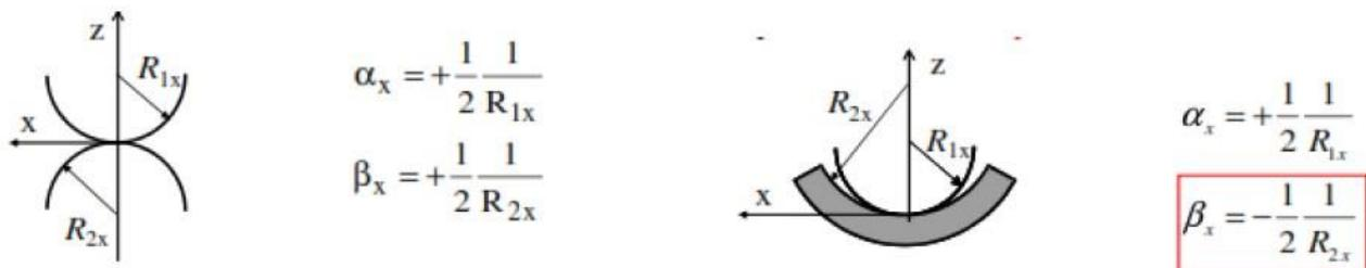
Figure 2.6.2 – Convention of sign for principal curvatures.
