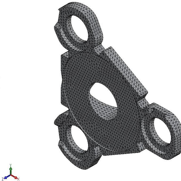
Figure 4.1.1 – Mesh of the lifting plate of the buckle.
