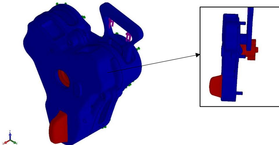
Figure 4.4.5.2.10 – Simulation adding the contact between lifting plate and internal surface of the upper body.
