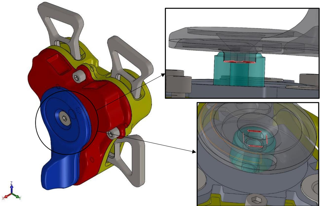
Figure 3.2.1 – Zoom of the interference between the lever and the camshaft.
