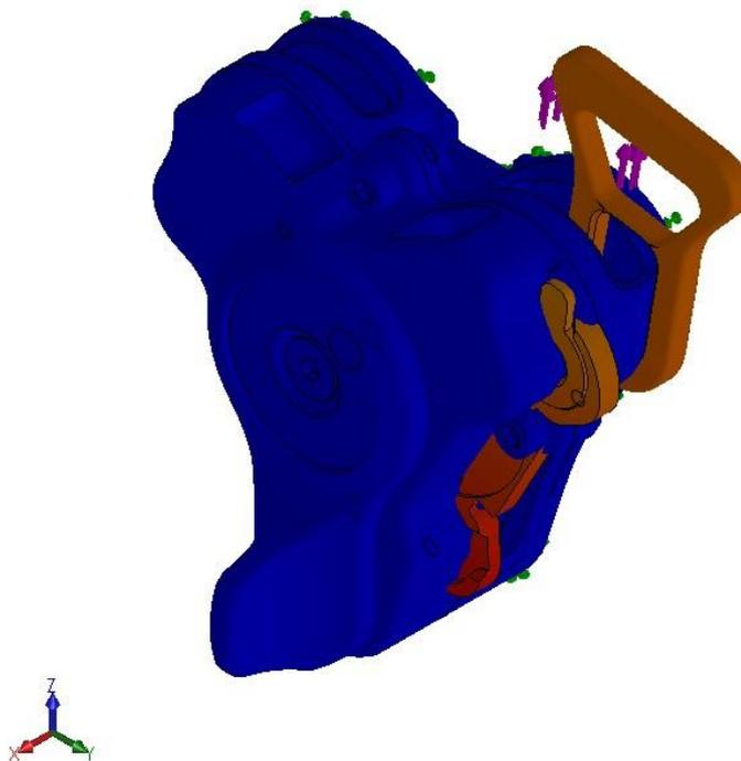
Figure 4.4.5.2.4 – Simulation with contact between tongue and latch.
