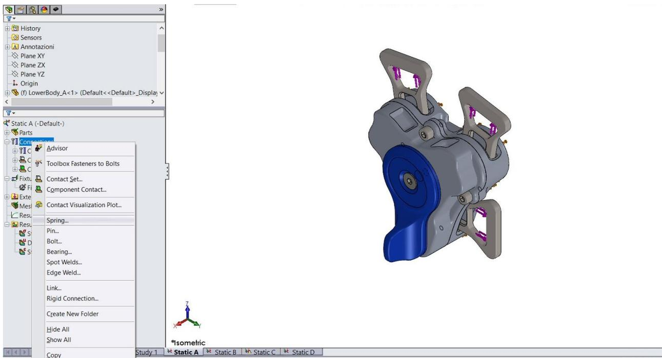
Figure 4.4.5.3.1 – How to open spring connector dashboard.
