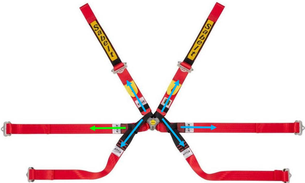
Figure 4.5.3.1 – Scheme to represent forces (blue) and fixture (green) on the buckle's tongues.
