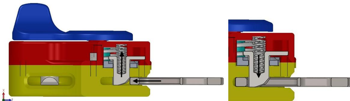
Figure 2.3.3 – Buckle section to show latch-tongue coupling.
