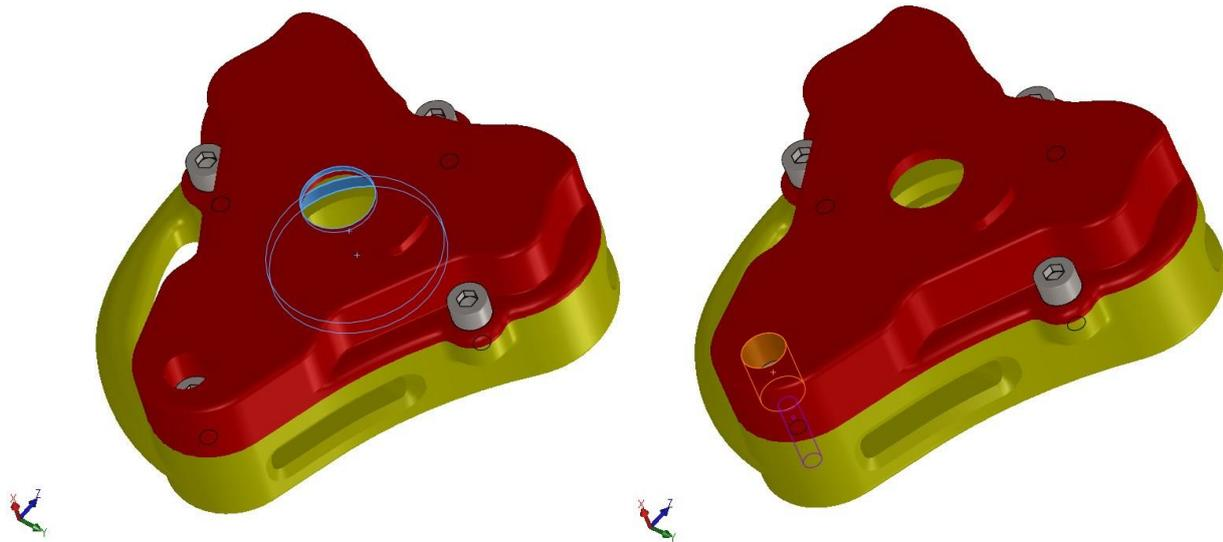
Figure 2.4.4 – Second and third mate to lock upper body in relation to lower body.
