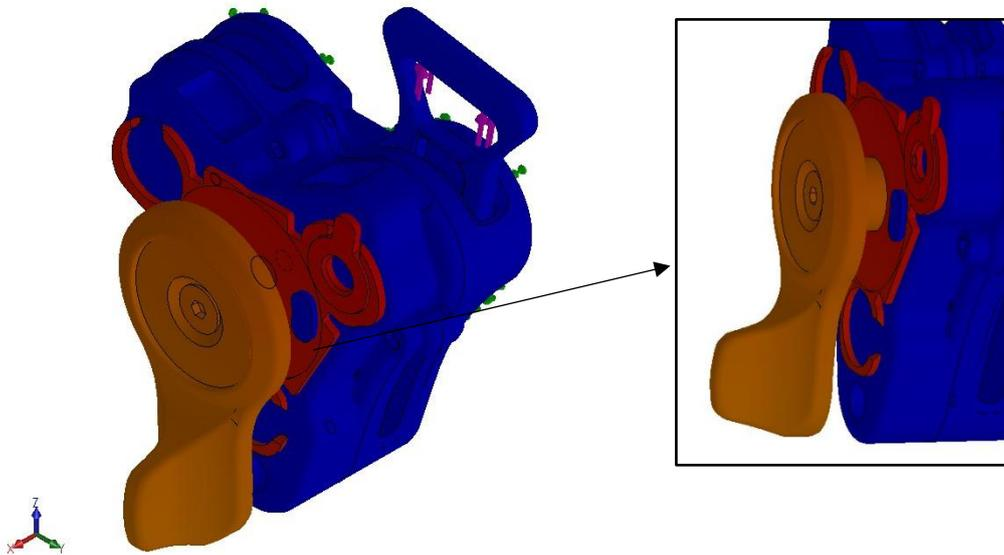
Figure 4.4.5.2.9 – Simulation adding the contact between lifting plate and camshaft.
