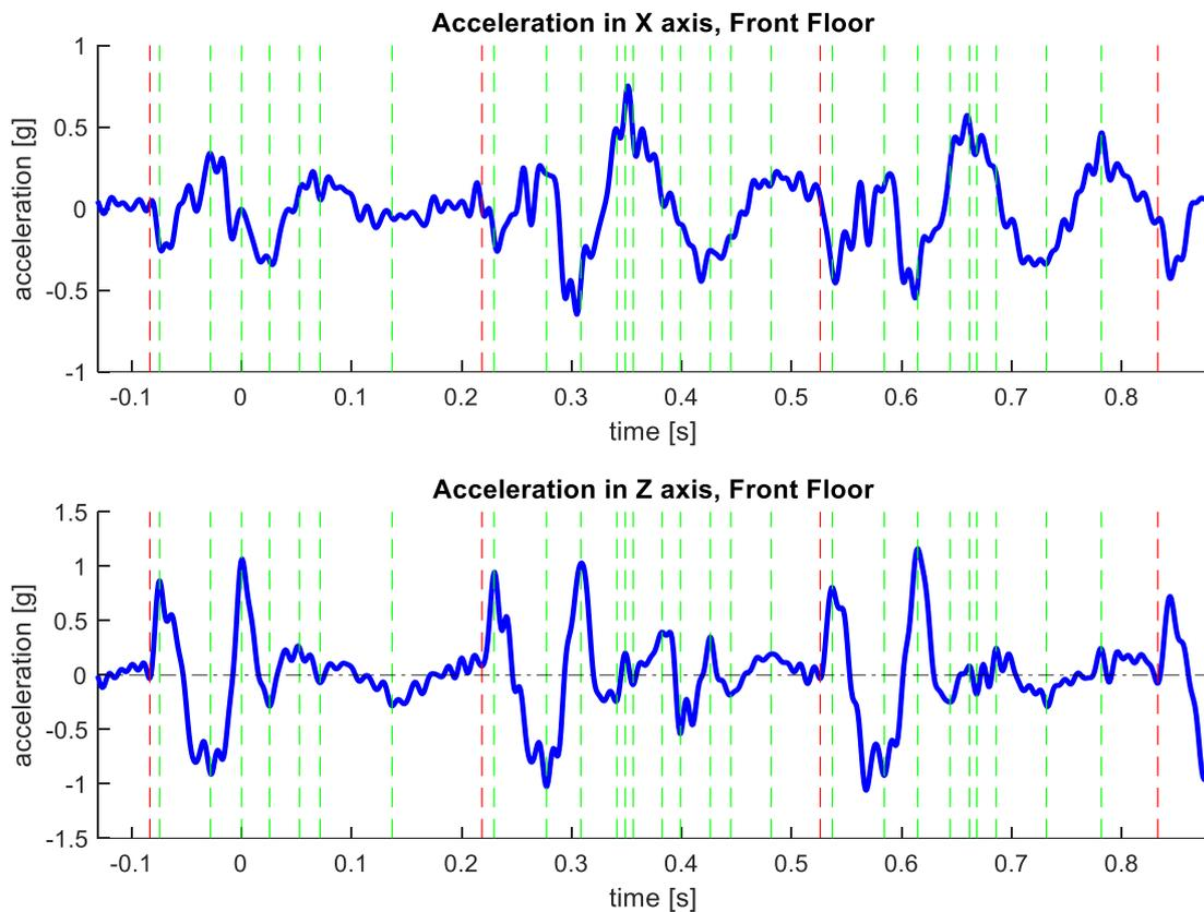
Figure 5.1.5.1: Zone of study, Front Floor Accelerometer, X and Z axes accelerations
