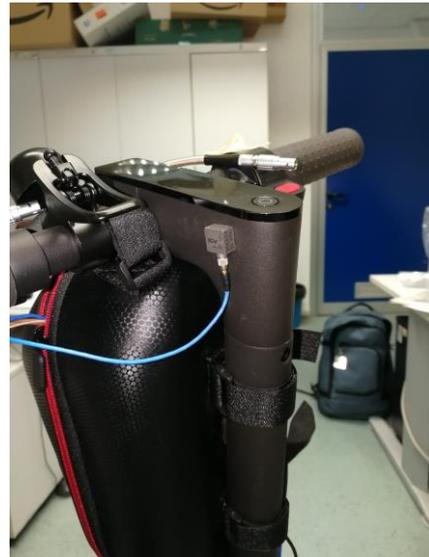
Figure 3.1.3. GPS and Front Floor Accelerometer (left) Steering Accelerometer (right)
