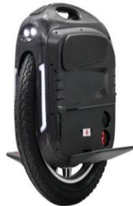
Figure 1.4.4: Self-balancing unicycle
