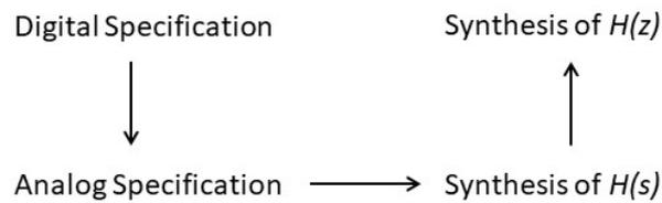
*Figure D. 5 Design of digital filters using analogue prototypes. Adaptation from (Wanhammar & Saramäki, 2020)*
