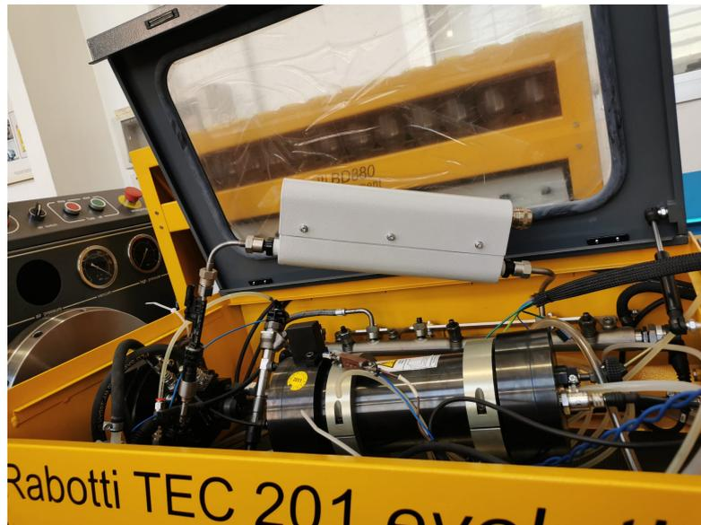
**Figure A.4:** Flow-meter connected to the circuit for diesel injection
