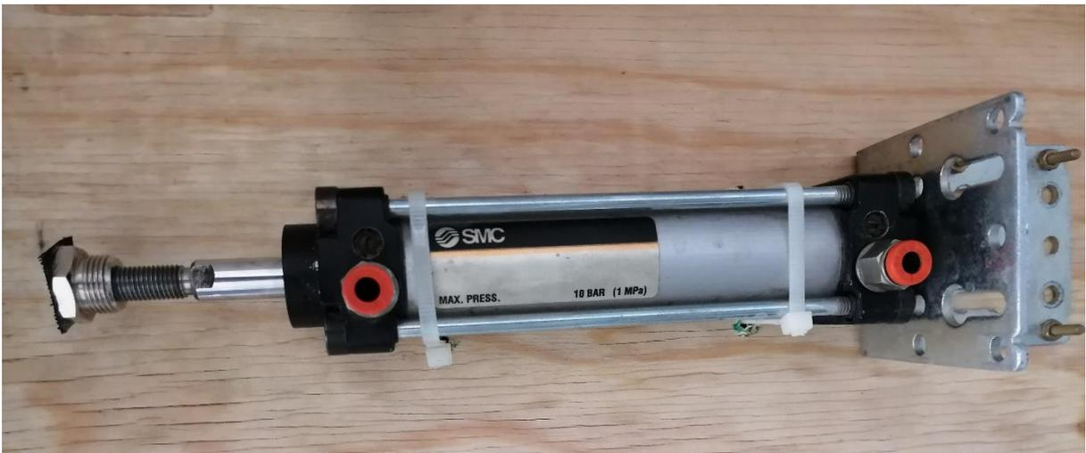
*Figure 4.1* SMC double-acting pneumatic cylinder.
