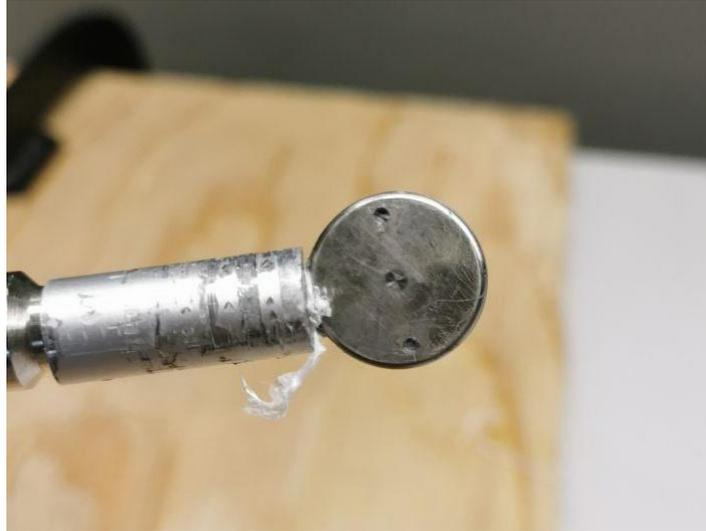
**Figure 5.5** Machined titanium alloy sample connected to the hand-made fitting.
