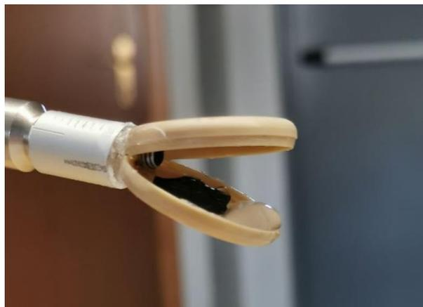
**Figure 5.6** PA molded sample, pressure test.
