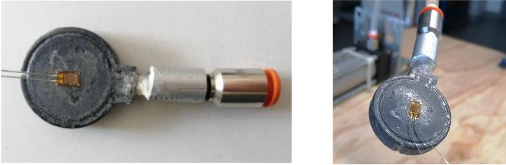
**Figure 6.3** Result of the installation of the linear strain gauge on the AM PA 12 sample.
