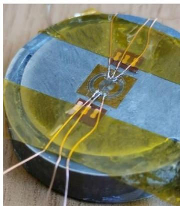
**Figure 6.18** Diaphragm strain gauge bonded on AM titanium capsule.
