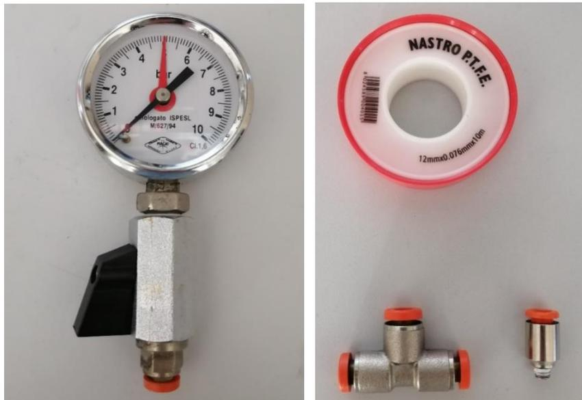
*Figure 4.5* Close-up view of the barometer, PTFE tape and push-in fittings.
