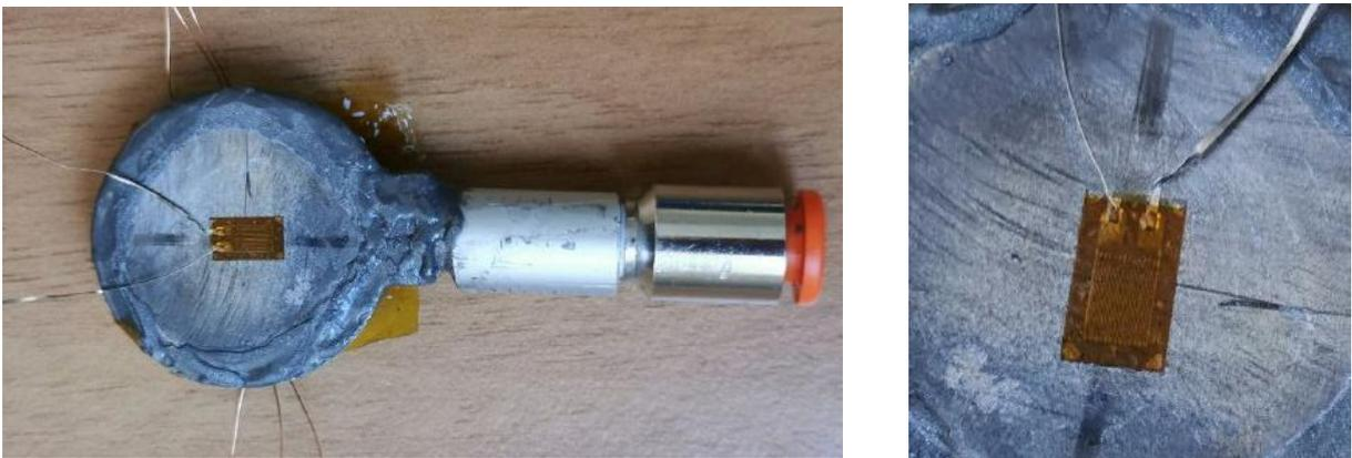
**Figure 6.2** Result of the installation of the linear strain gauge on the AM Ti6Al4V sample.
