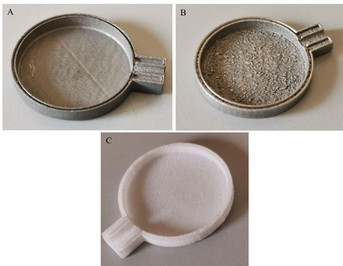
**Figure 5.2** 3D printed samples: A) Ti6Al4V; B) AlSi10Mg; C) PA 12.
