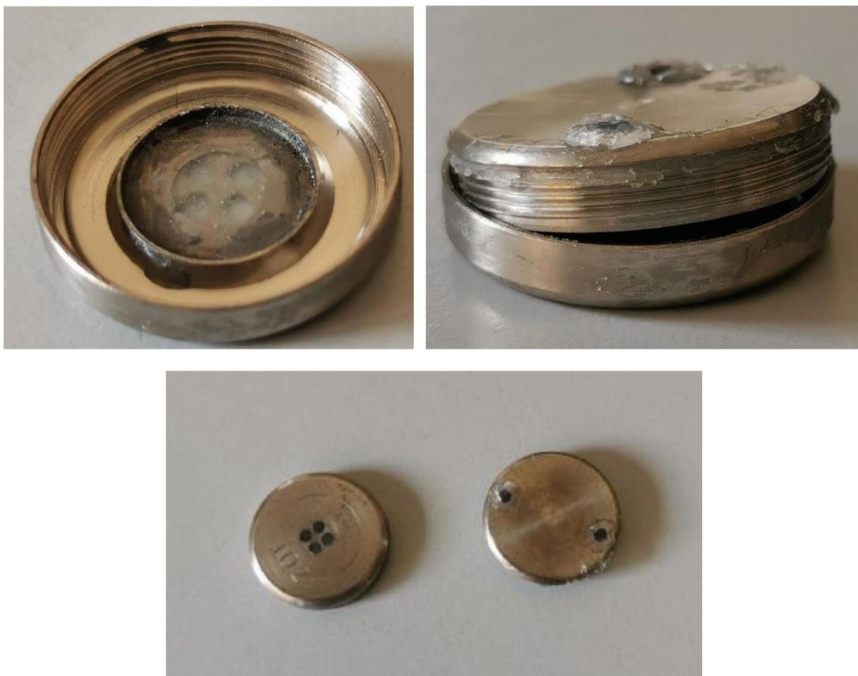
**Figure 5.4** Machined titanium alloy capsule sent by the Houston Methodist Research Institute.
