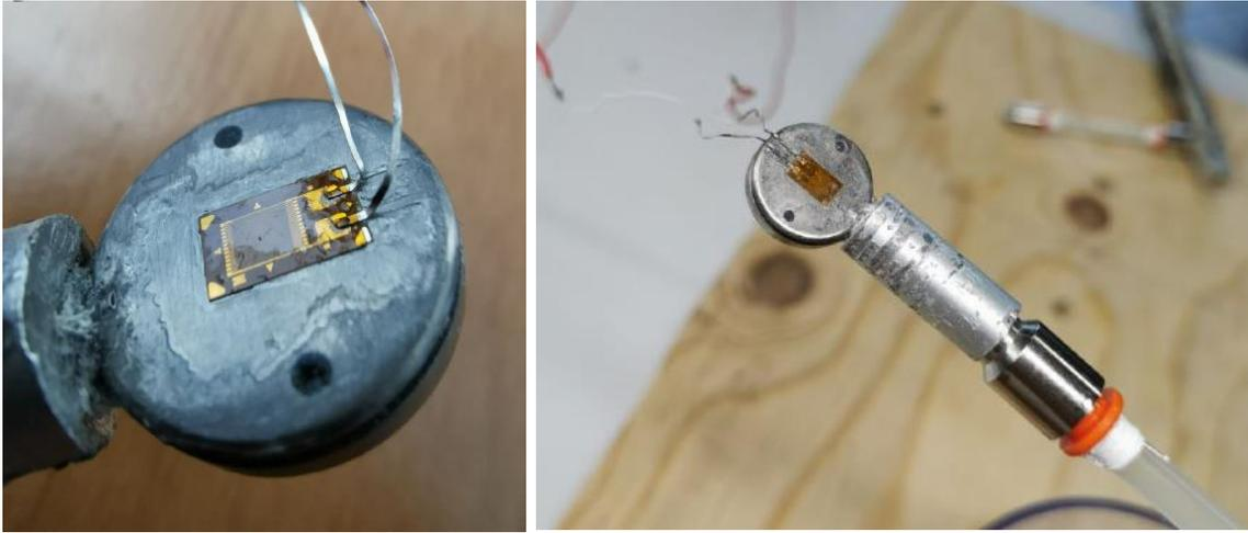
**Figure 6.1** Result of the installation of the linear strain gauge on the machined Ti6Al4V sample.
