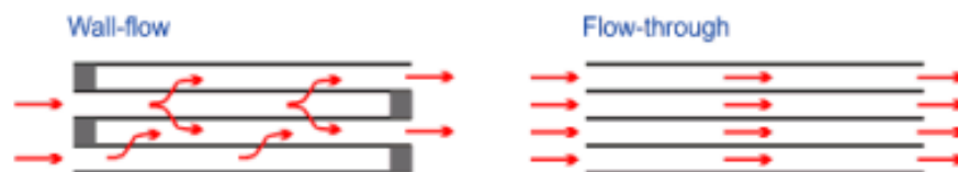
Figure 16 - DPF structure Wall-flow and Flow-through (1)
