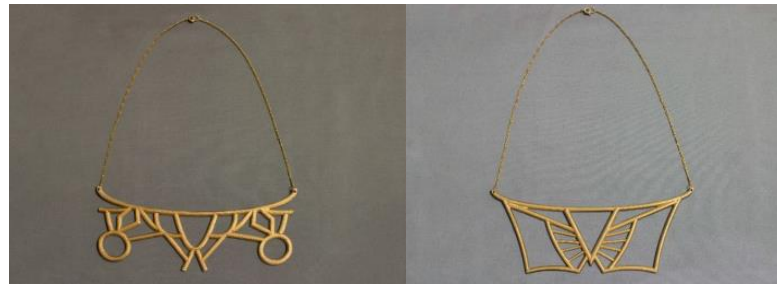
Figure 76: Design of jewellery pendants 4 (on the left) and 5 (on the right) made of white PLA filament and respectively brush and spray painted with gold paint source: Pasricha & Greeninger (2018)
