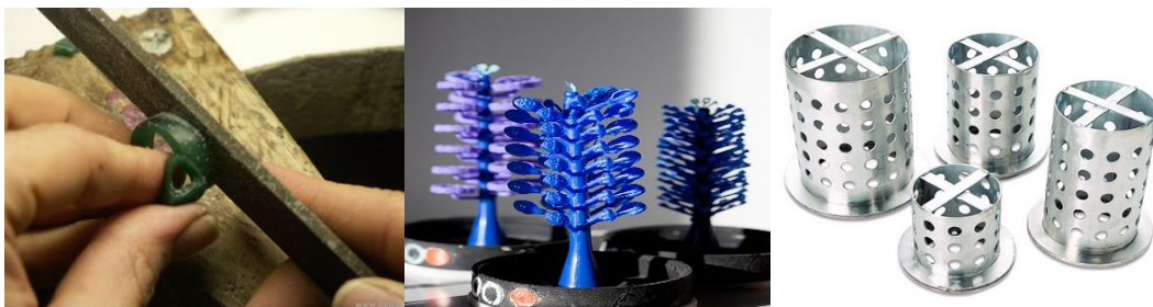
Figure 44: Steps: model creation - wax trees – flasks
