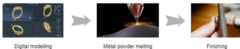
Figure 46: Selective Laser Melting common steps
