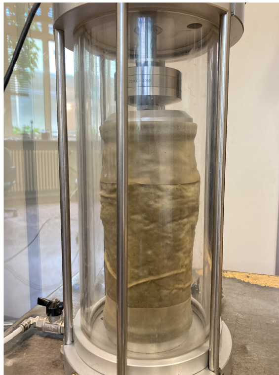
Figure 4.10: Specimen After Quick Shear Test
