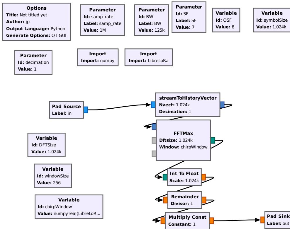
Figure A.1: Flowgraph of the DFTPeak block in GNU Radio companion.
