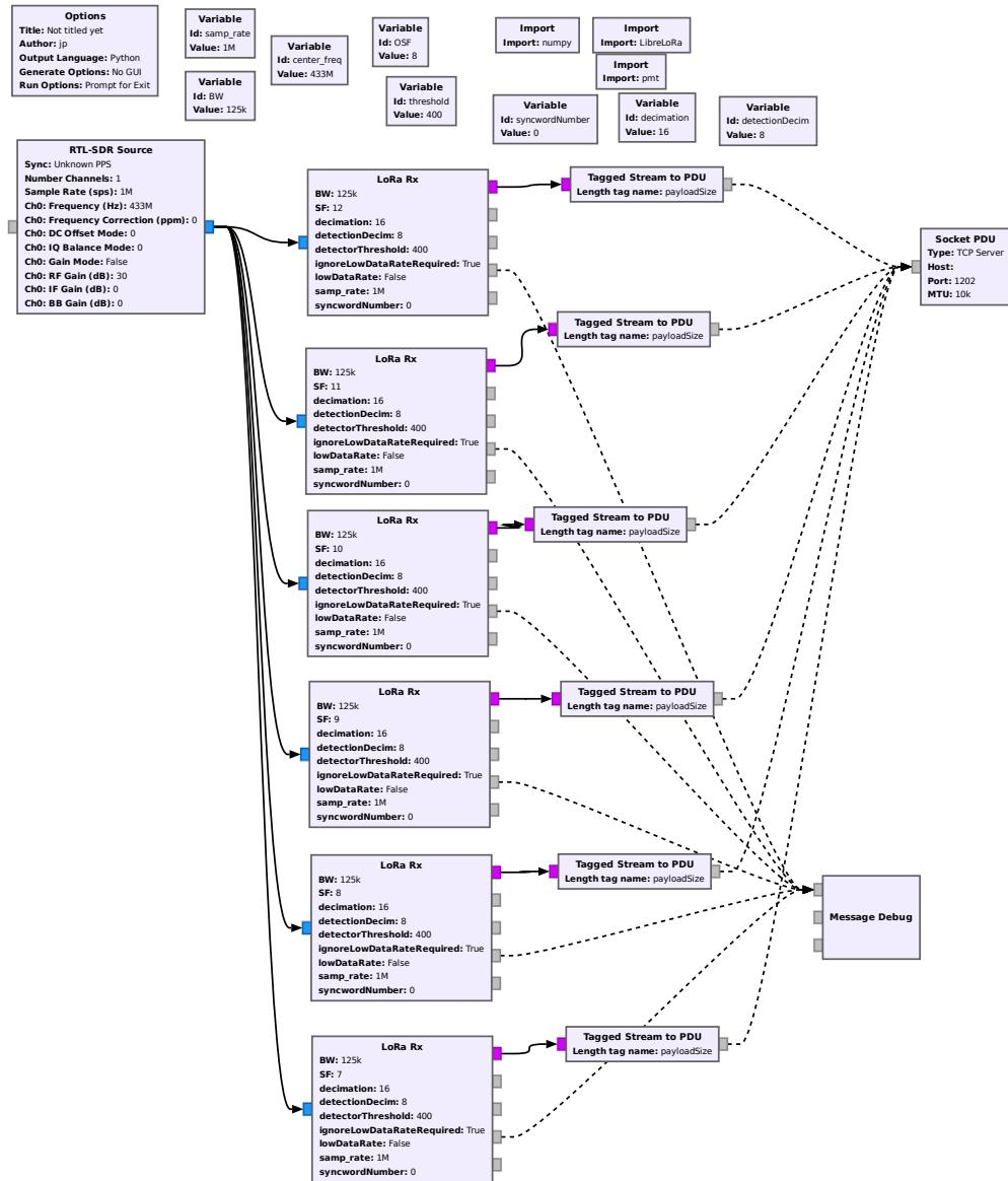
Figure 6.3: Flowgraph of the Multi-Parameter, Multi-Channel Receiver.
