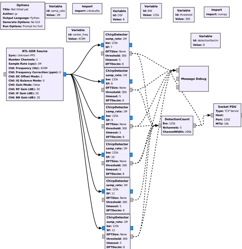
Figure 6.2: Flowgraph of the LoRa multi-channel multi-SF detector.
