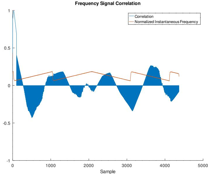
Figure 4.4: Output signals of the correlator when receiving the end of the preamble a LoRa frame with SF = 7, CRC on, and payload of a single byte containing a power of 2 (1, 2, ..., 128).
