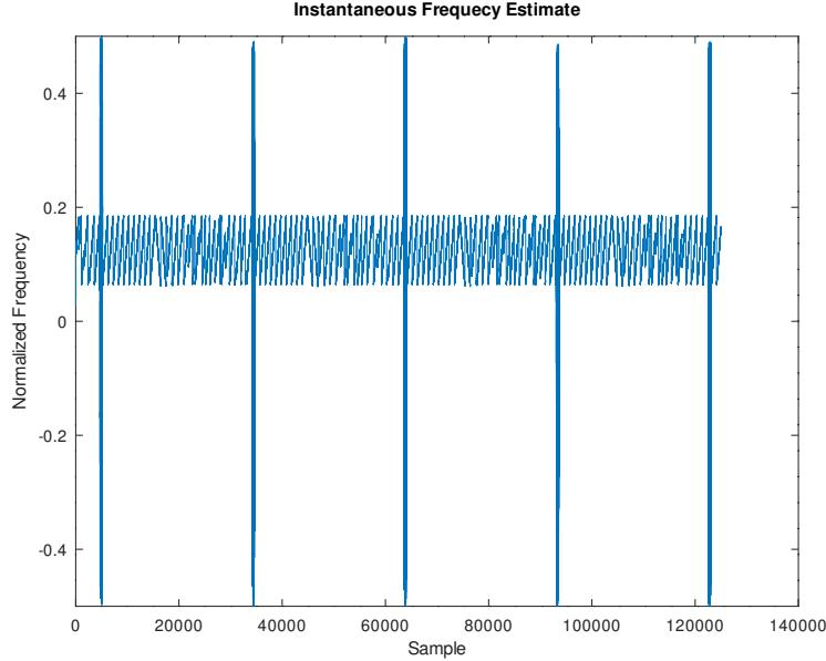
Figure 4.2: Output signal of the stochastic gradient descent frequency tracker given the described test signal at its input.
