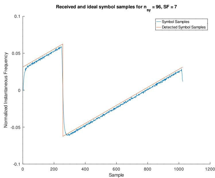
Figure 4.7: Synchronized frequency samples of a received LoRa symbol together with the samples of the symbol detected by the minimum squares decider block when given the former as an input.
