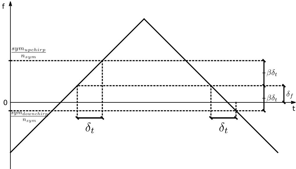
Figure 4.6: Illustration of the offset estimation procedure with a single upchirp (as sync word) and downchirp.
