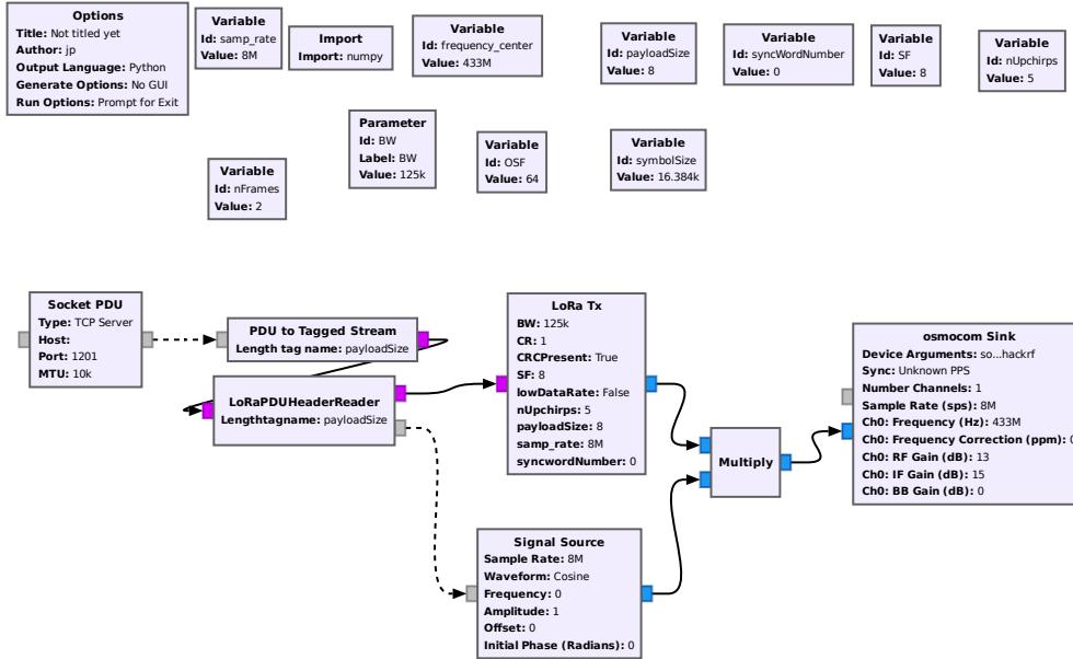
Figure 6.4: Flowgraph of the Variable Parameter Transmitter.
