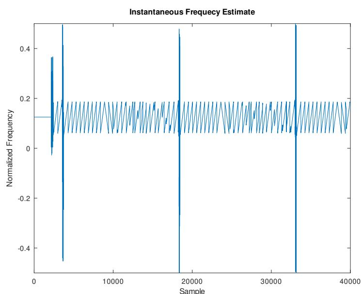
Figure 4.3: Output signal of the DFT peak frequency tracker given the described test signal at its input.
