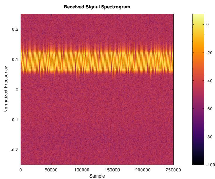
Figure 4.1: Spectrogram of the input signal composed of a sequence of LoRa frames with SF = 7, CRC on, and payloads of a single byte containing powers of 2 (1, 2, ..., 128).
