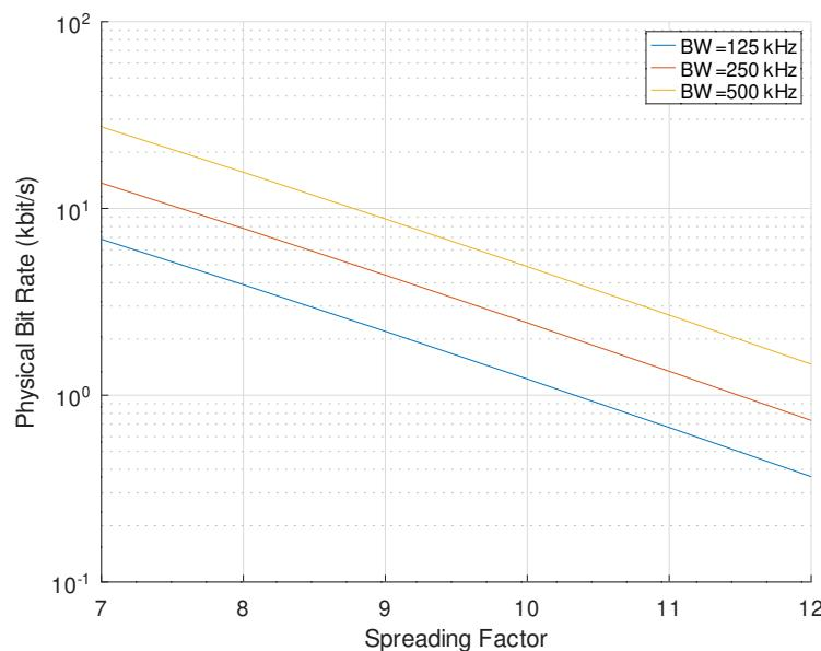
Figure 2.1: Physical bit rate in function of spreading factor (SF) and bandwidth (BW) for some of the possible values.
