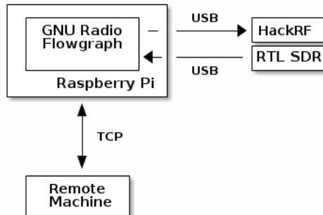
Figure 6.1: Block diagram of employed hardware setup.
