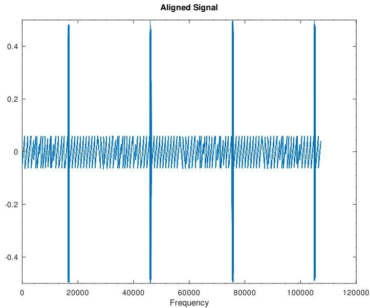
Figure 4.5: Synchronized signal, as generated by the synchronizer when its input is the previously shown test signal.
