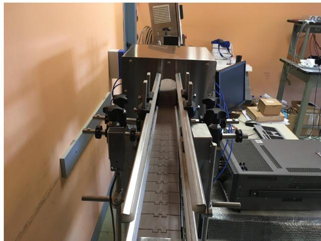
(b) The insulating box positioned around the antennas.
