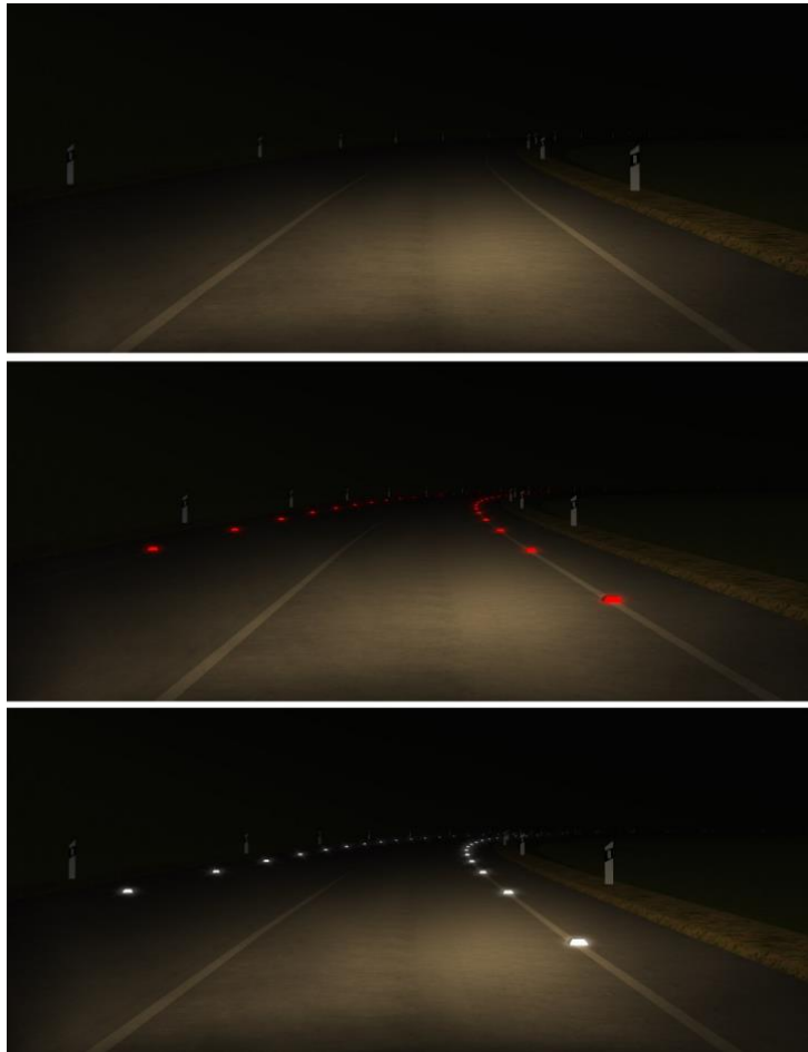
Figure 3: A curve screenshot of the three scenarios: the unlit road configuration without LED (upper); the red LED road stud configuration (middle), and the white LED configuration (bottom).
