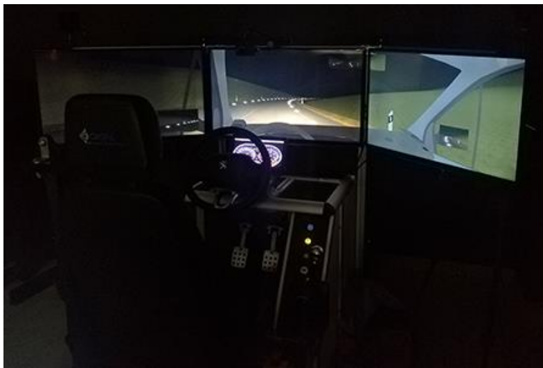
Figure 7: Driving simulator set-up
