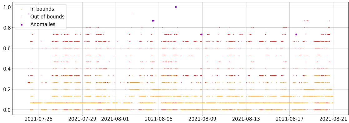
**Figura 5.21:** ISOLATION FOREST anomaly detection sulla metrica *ExitThreadIdleCount*
