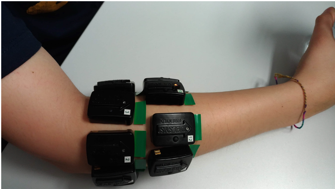
Figure 2.9: Example of final sensor placement on a subject involved in the acquisition of NinaPro DB6 [38]
