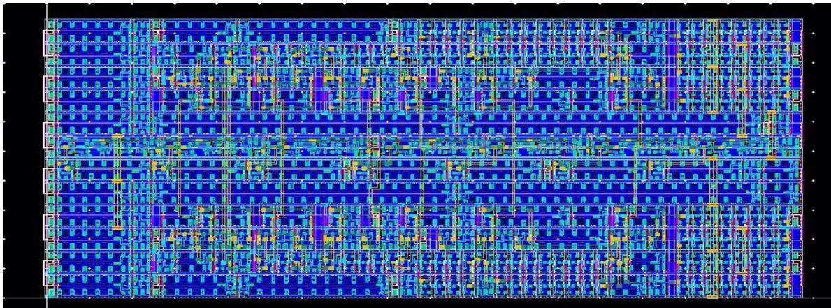
Figure 4-7 Layout of Programmable non-overlapping clock generator
