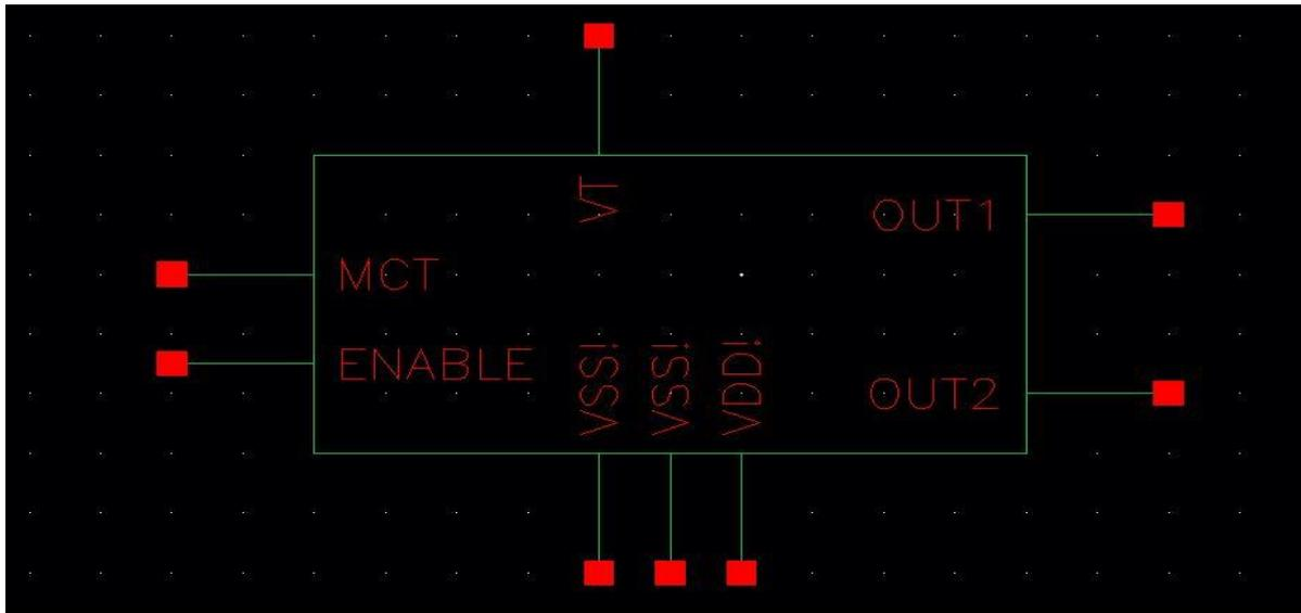
Figure 4-17 Symbol of output amplifier
