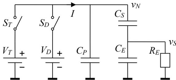
Figure 2-3 Bias conditions in phase 2 ( $t_1 < t < t_2$ )
