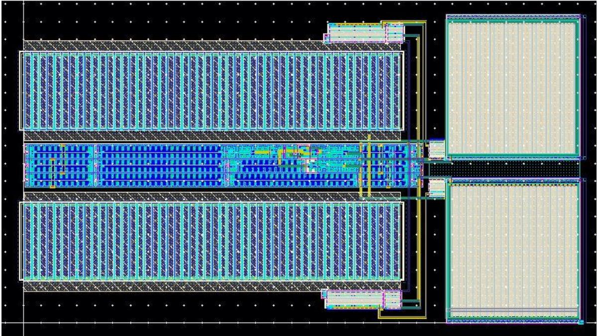
Figure 4-18 Layout of Output Stage Amplifier
