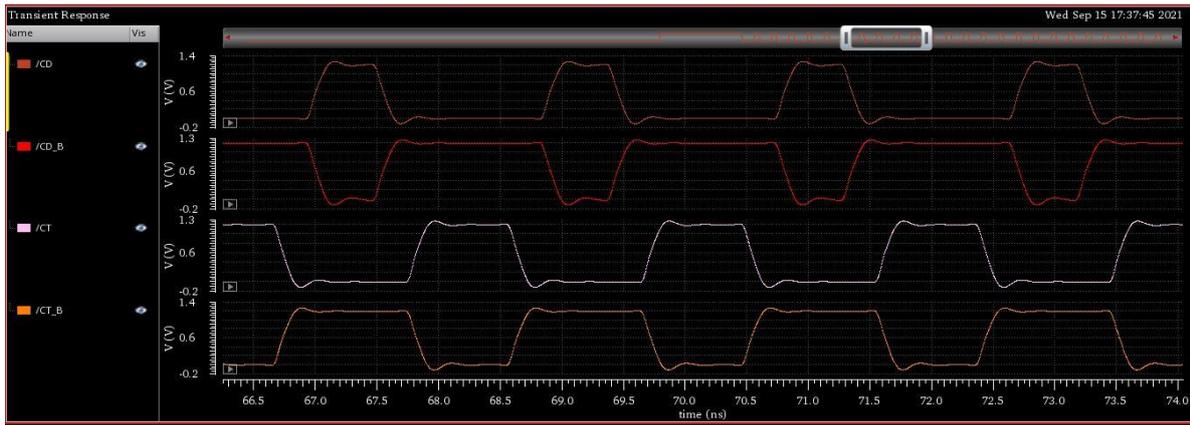
Figure 5-8 Output waveforms for 2 nH and 1 pF
