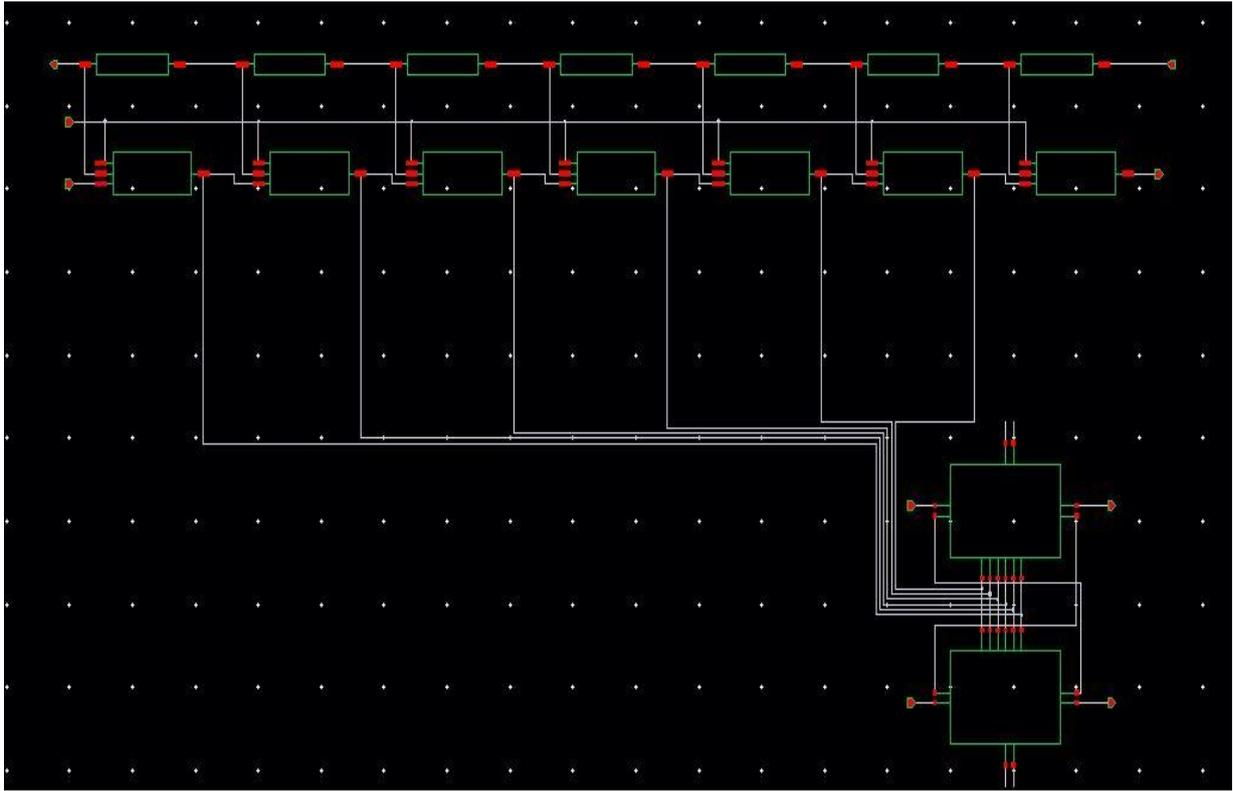
Figure 4-6 Schematic of Programmable non-overlapping clock generator
