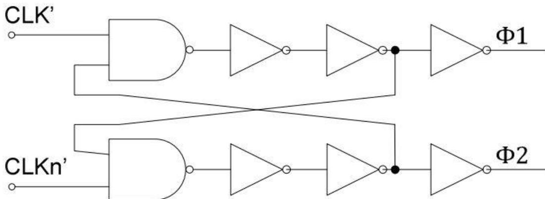
Figure 4-1 Conventional two-phase clock generator
