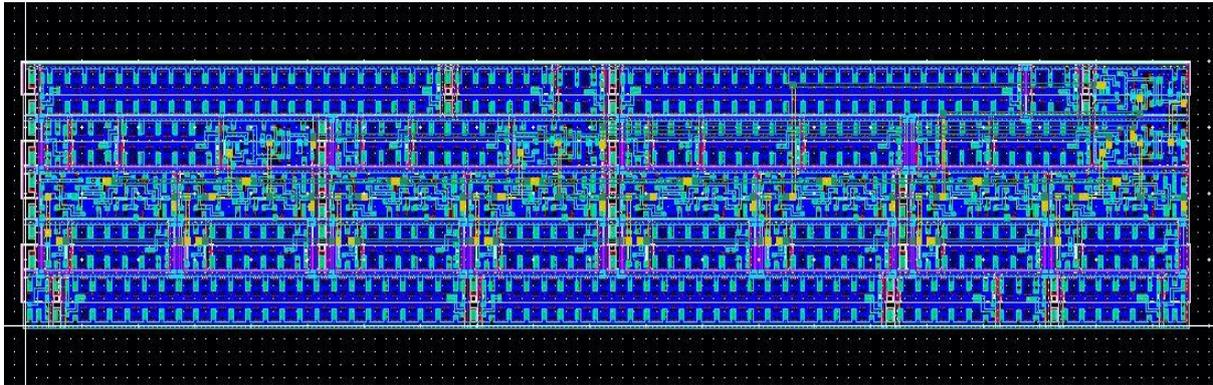
Figure 3-19 Layout of the programmable MUX
