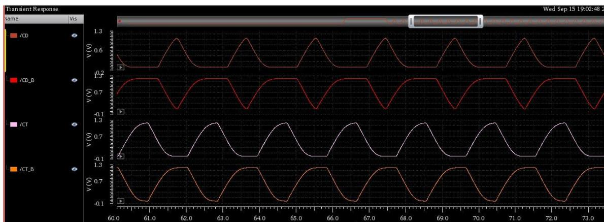
Figure 5-10 Output waveforms for 2 nH and 4 pF
