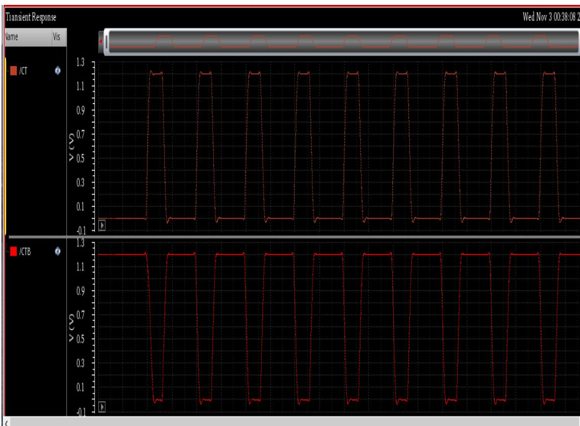
Figure 4-16 Spectre Simulation of Output Stage
