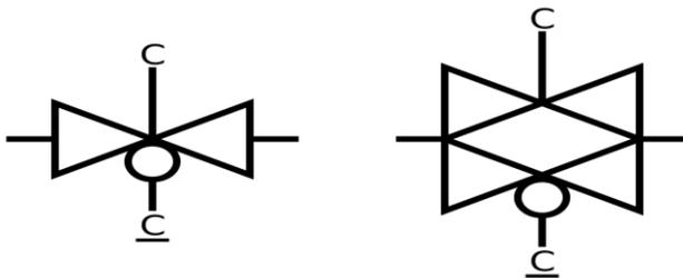
Figure 4-10 Symbol of transmission gate
