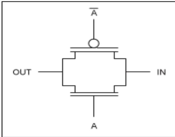
Figure 4-11 Circuit of transmission gate
