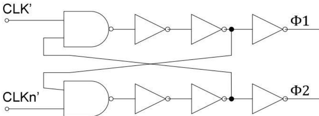
Figure 4-1 Conventional two-phase clock generator
