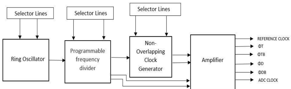
Figure 2-6 Block diagram of the clock generator
