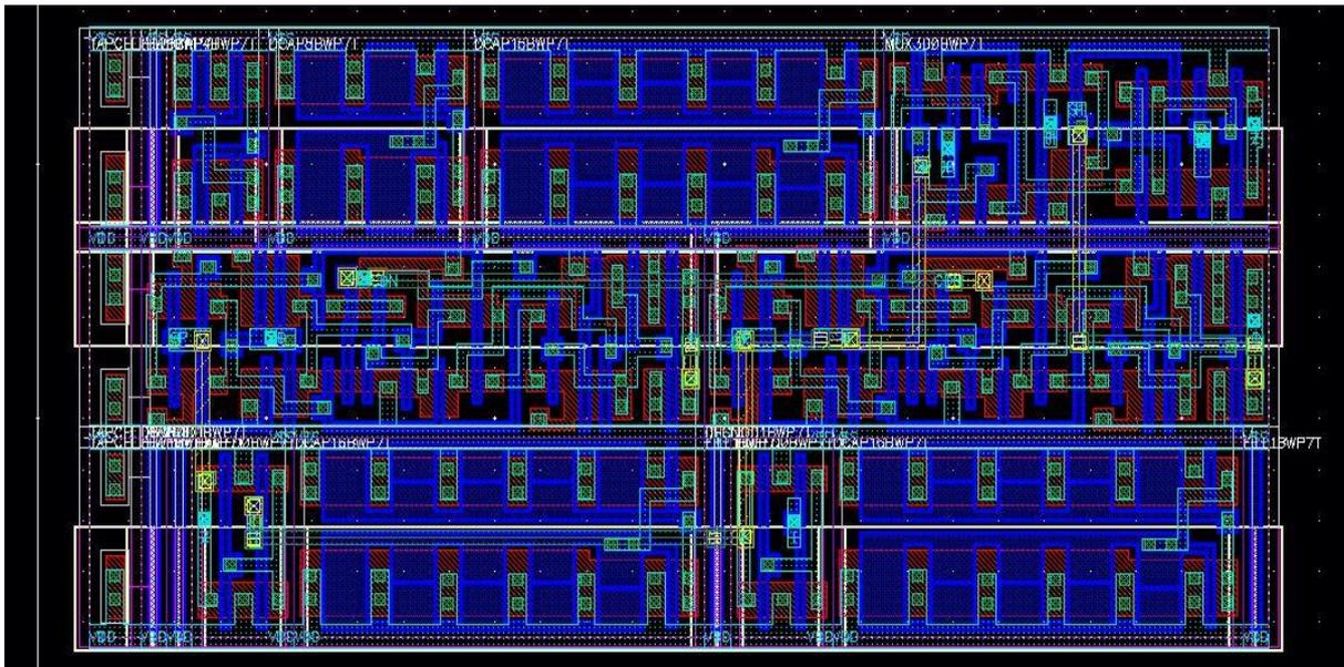
Figure 3-21 ADC MUX layout
