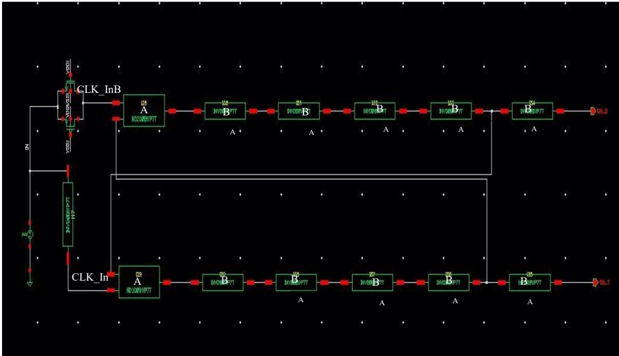
Figure 4-2 Non overlapping clock generator. A: NAND, B: Inverter.
