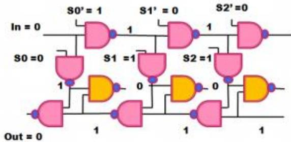
Figure 3-3 Glitching when Delay Path is one
