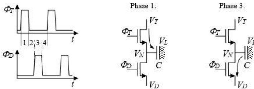
Figure 2-1 The 4 phases of the non-overlapping clock for charging (1) and discharging (3) of the nanoelectrode capacitor  $C$
