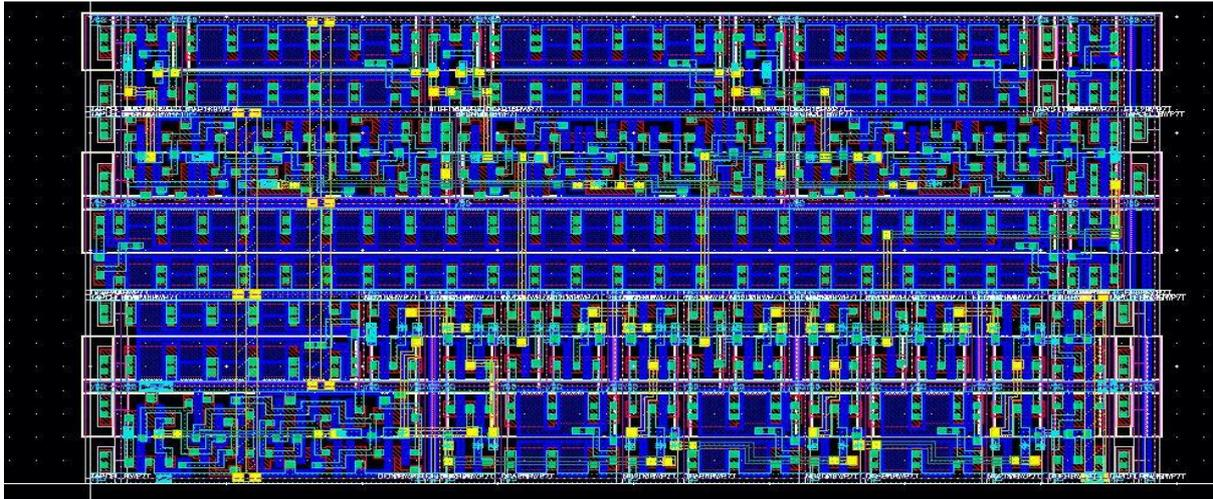
Figure 3-10 Layout of Programmable Ring Oscillator
