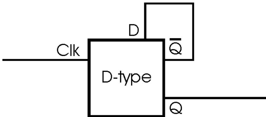
Figure 3-13 D-type frequency divide by two circuit
