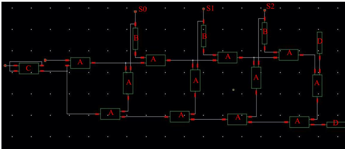
Figure 3-5 Ring Oscillator with selectable path. A: NAND gate, B: inverter, C: D Flip Flop and D: GTIE Cell
