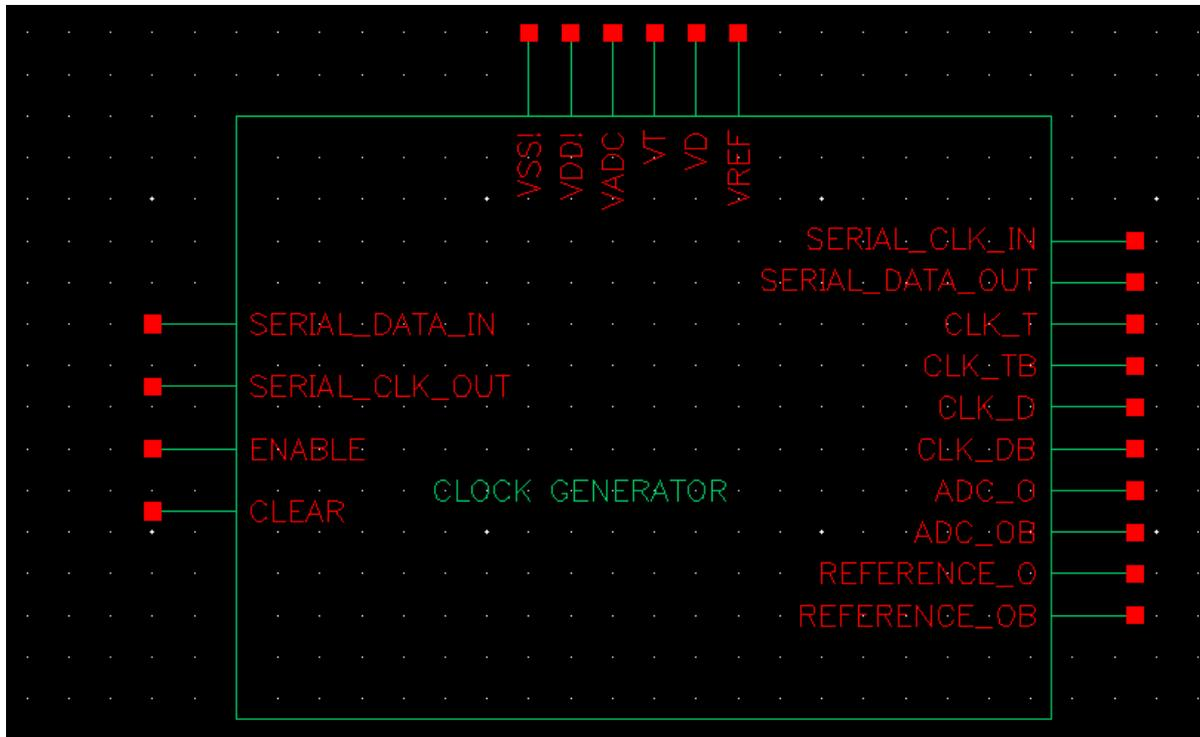
Figure 5-2 Symbol of the clock generator
