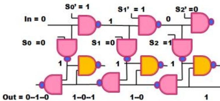
Figure 3-4 Glitching when Delay Path increases by one
