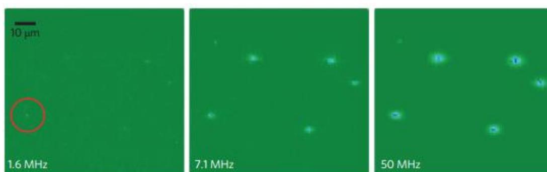
Figure 1-7 Two-dimensional maps of the measured response  $\Delta C_{exp}$  at different modulation frequencies
