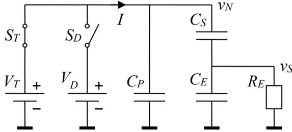
Figure 2-2 Bias conditions in phase 1 ( $0 < t < t_1$ )
