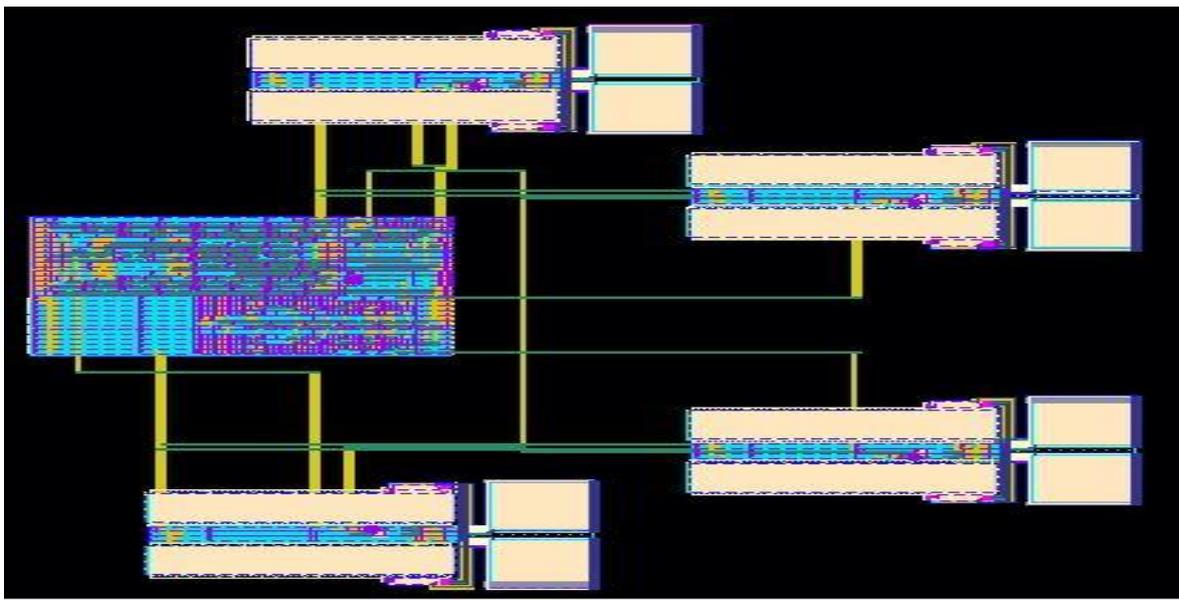
Figure 5-3 Layout of the clock generator
