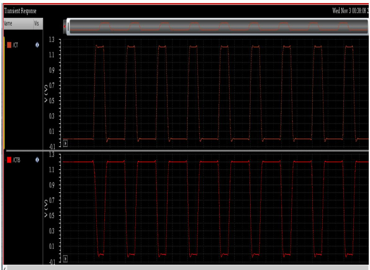
Figure 4-16 Spectre Simulation of Output Stage
