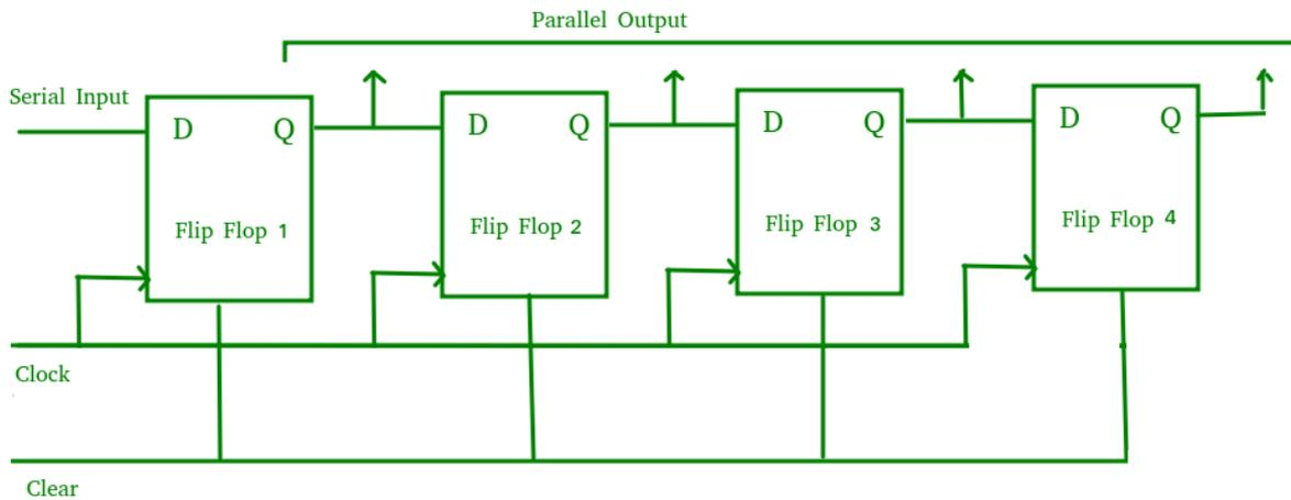
Figure 3-6 Serial In Parallel Out Shift Register
