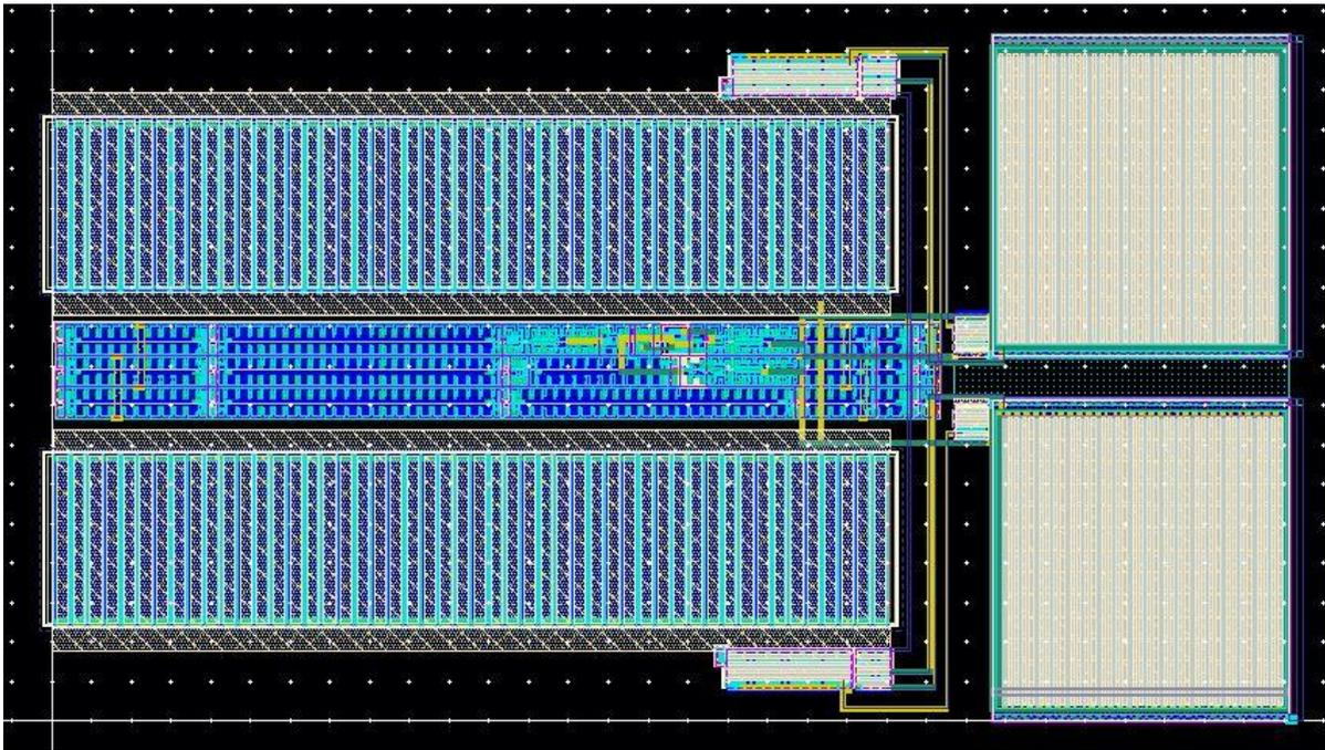
Figure 4-18 Layout of Output Stage Amplifier
