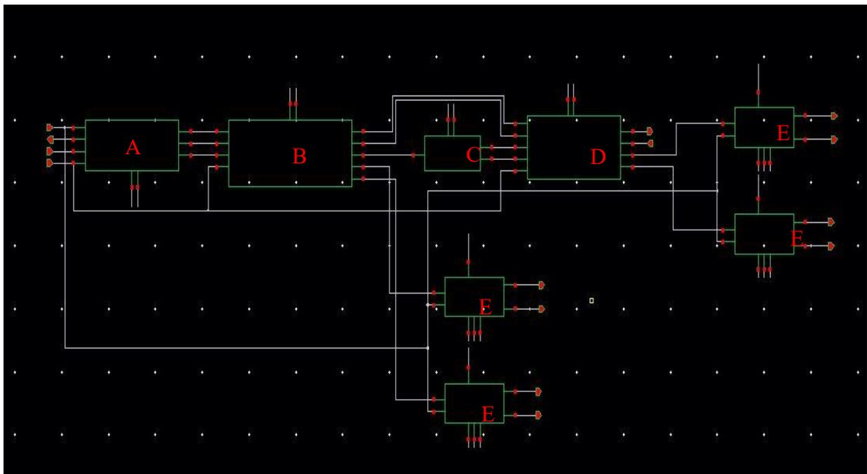
Figure 5-1 Schematic diagram of clock generator. A: Ring Oscillator, B: Programmable Frequency Divider, C: Transmission Gate, D: Non-overlapping Clock Generator, E: Output stage Amplifier
