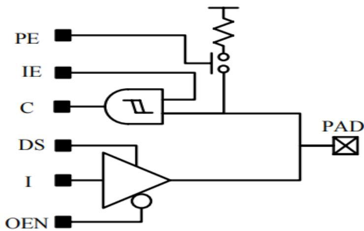
Figure 5-13 Digital Pin PDDW1216SCDG
