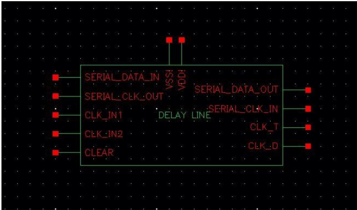
Figure 4-8 Symbol of Programmable non-overlapping delay line
