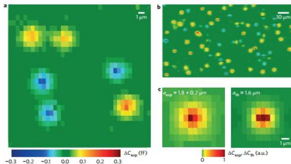
Figure 1-8 a and b: Response to conducting (yellow/orange) and dielectric spheres (cyan/blue). c: comparison of measured (left) and simulated (right) apparent particle sizes.
