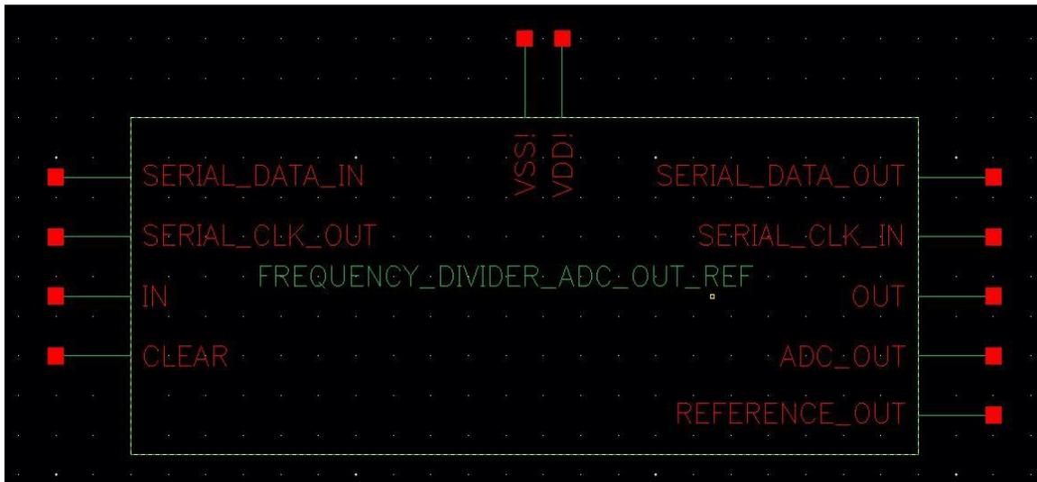
Figure 3-24 Symbol of the programmable frequency divider
