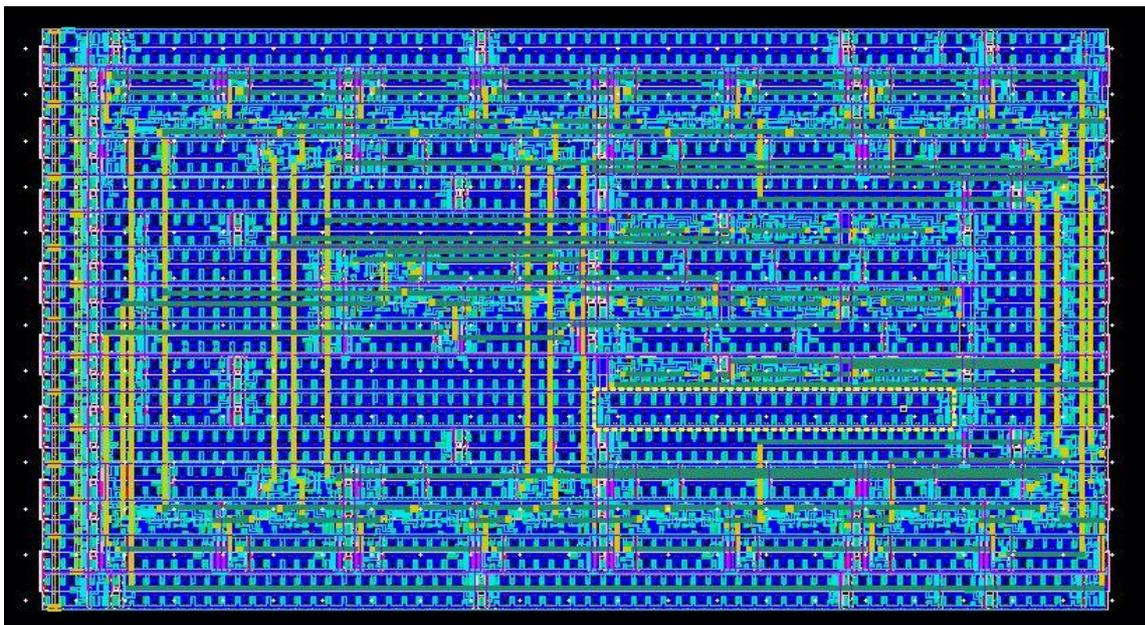
Figure 3-23 Layout of the programmable frequency divider
