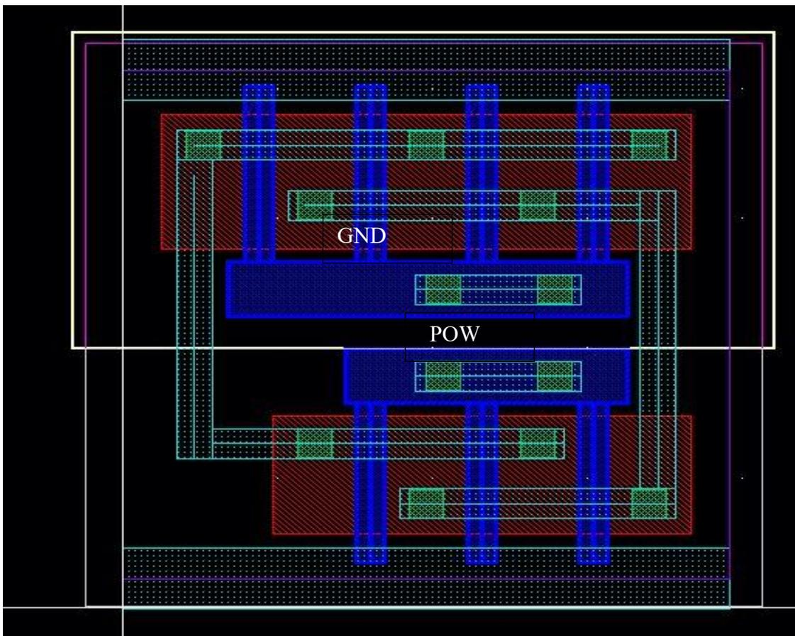
Figure 4-13 Circuit of transmission gate for the delay line
