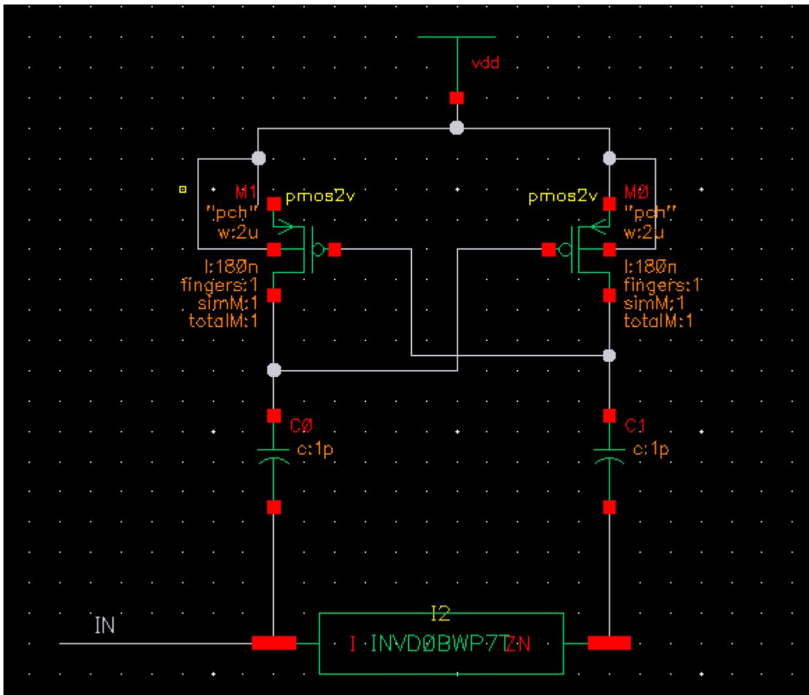
Figure 4-14 Cross-coupled rectifier circuits
