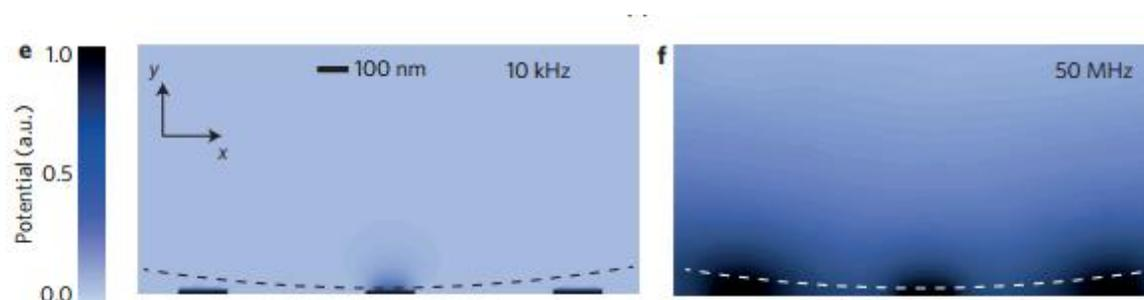
Figure 1-6 Maps of the AC potential amplitude generated by three electrodes at 150 mM salt concentration at zero DC bias and 10 kHz and 50 MHz modulation frequencies
