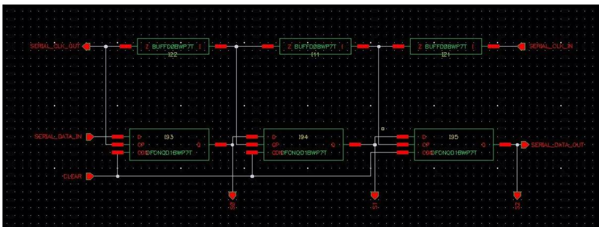
Figure 3-7 SIPO used for Ring Oscillator
