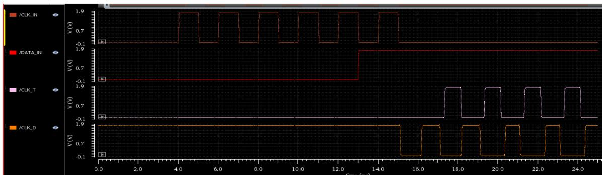
Figure 4-9 Spectre Simulation for the Delay Line
