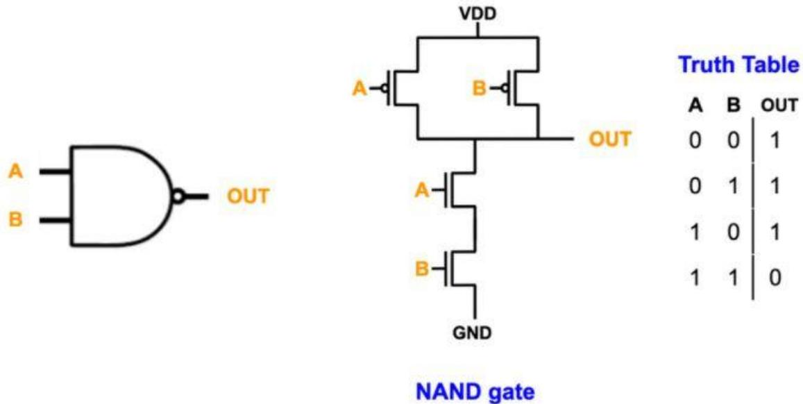
Figure 3-2 Gate-level and transistor-level representation of NAND2 and its truth table.
