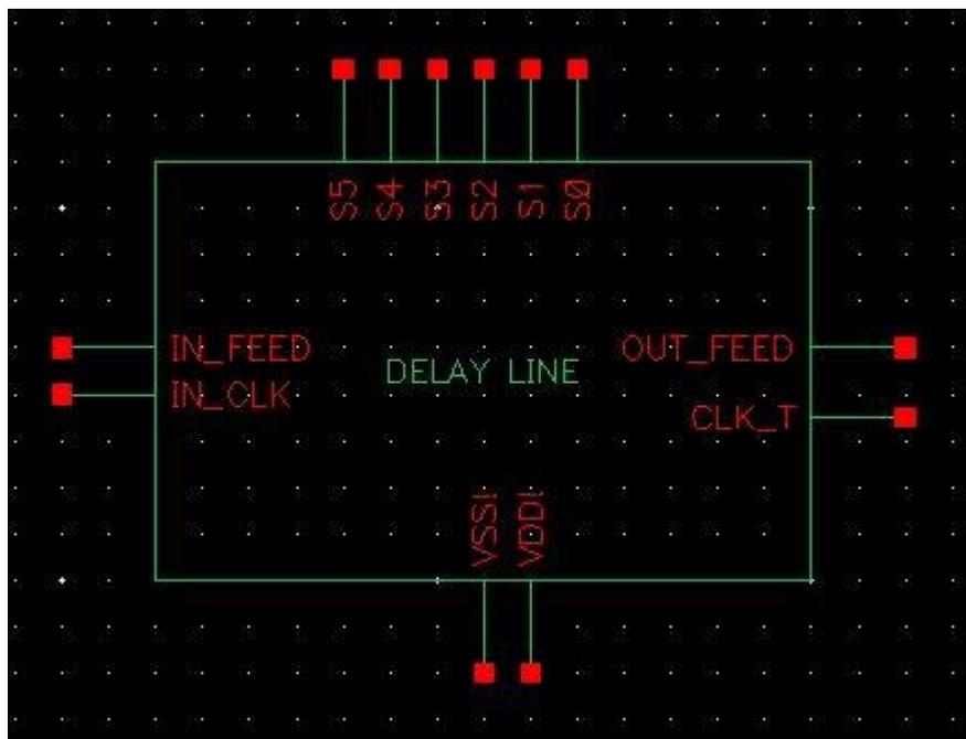
Figure 4-5 Symbol of the programmable delay path of figure 4.4
