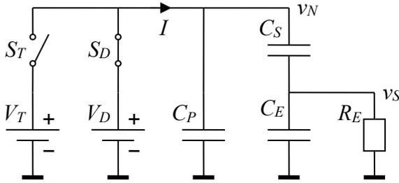
Figure 2-4 Bias conditions in phase 3 ( $t_2 < t < t_3$ )
