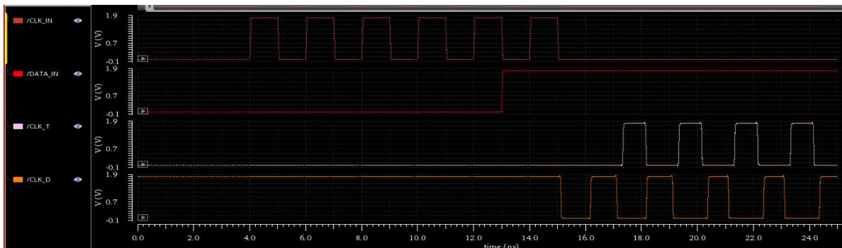
Figure 4-9 Spectre Simulation for the Delay Line
