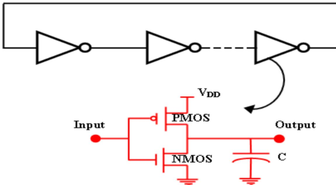
Figure 3-1 Hardware structure of single-ended inverter-based ring oscillator
