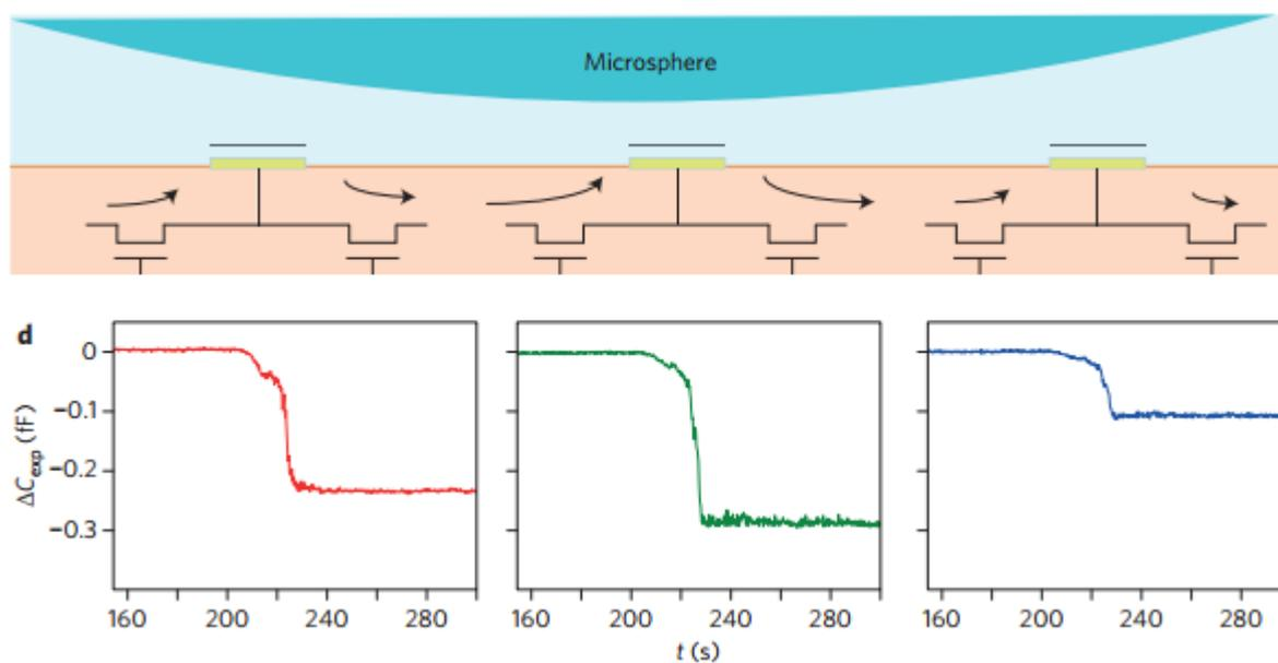
Figure 1-5 Time traces recorded from three contiguous nanoelectrodes during sedimentation
