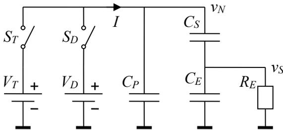
Figure 2-5 Bias conditions in phase 4 ( $t_2 < t < t_4$ )
