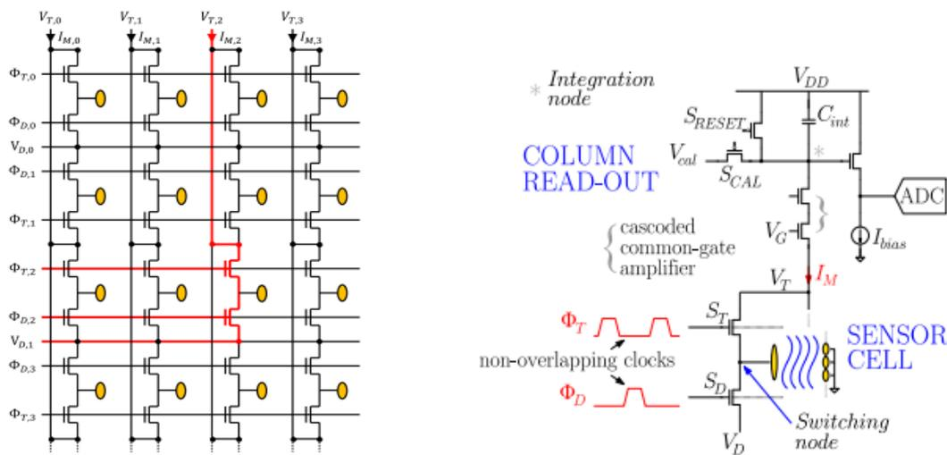
Figure 1-4 Left: Biosensor  $256 \times 256$  nanoelectrode array with column-wise selectable and row-wise readable sensor cells. The golden ellipses are the sense electrodes. A sensor cell and its selection and read paths are highlighted in red. Right: Sensor cell and column read-out circuit.
