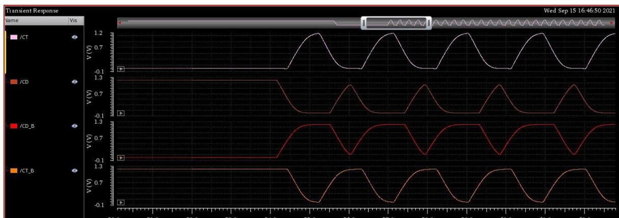
Figure 5-7 Output waveforms for 1 nH and 4 pF
