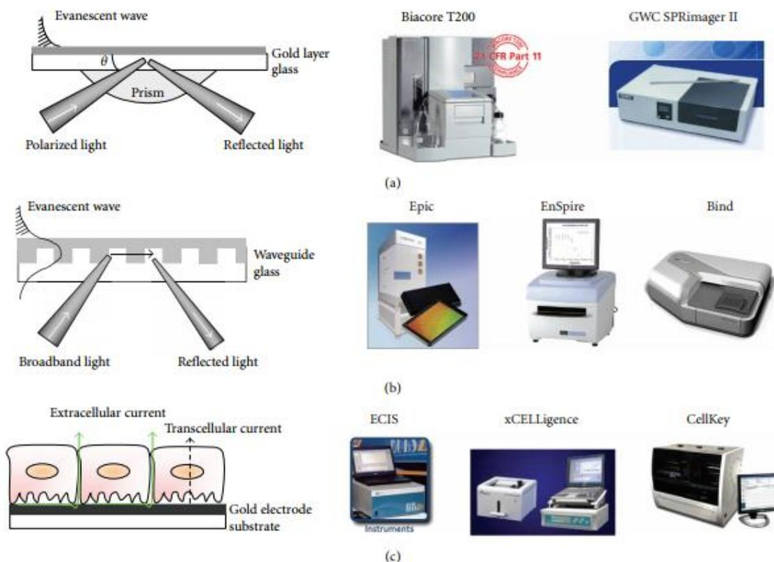
Figure 1-2 Standards and commercial instruments of three particular kinds of label-free biosensors
