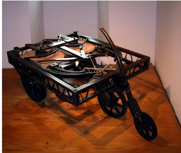
Figure 1.2: A self-propelled cart replica at museum Clos Lucé [5]
