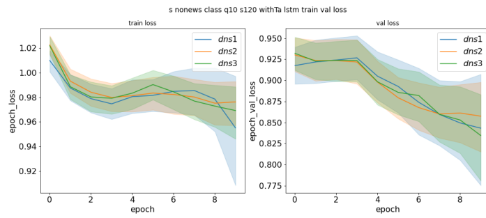
Figure 6.69: Loss plot for neural network trained with Nasdaq 100 dataset in classification single-task learning mode, without news feature , lstm cells, with technical analysis features.
