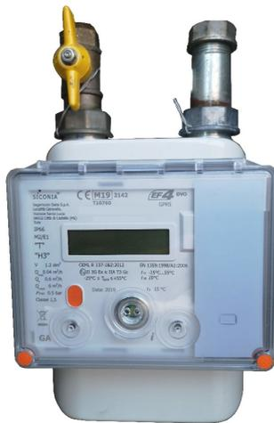
Figure 1.2: Electronic GAS consumption meter.
