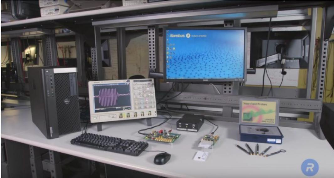
Figure 2.4: Side channel analysis instrument bench [18].
