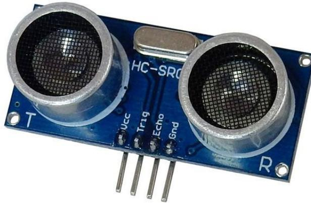
Figure 2.2. Ultrasonic sensor.
