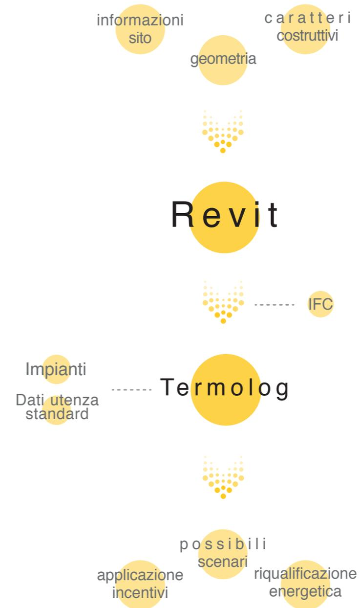
Fig.10\_Schema del workflow
