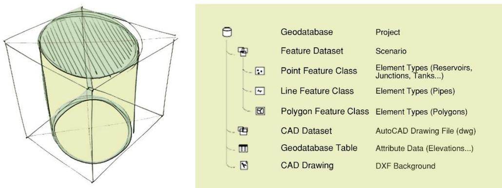
Figure 22. Internal structure of a File Geodatabase.
