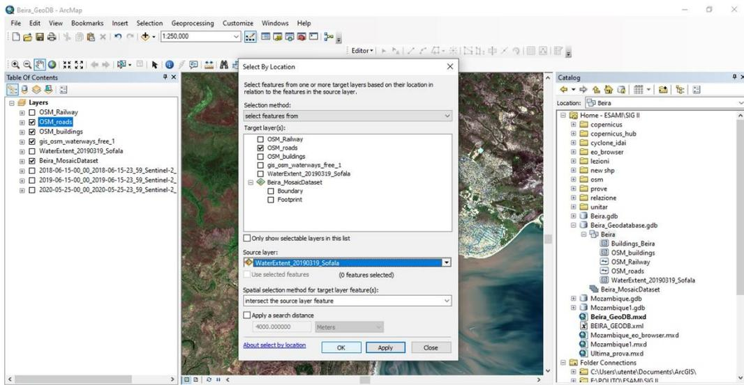
Figure 31. Select by Location tool intersecting the system of infrastructures with the water extent layer.
