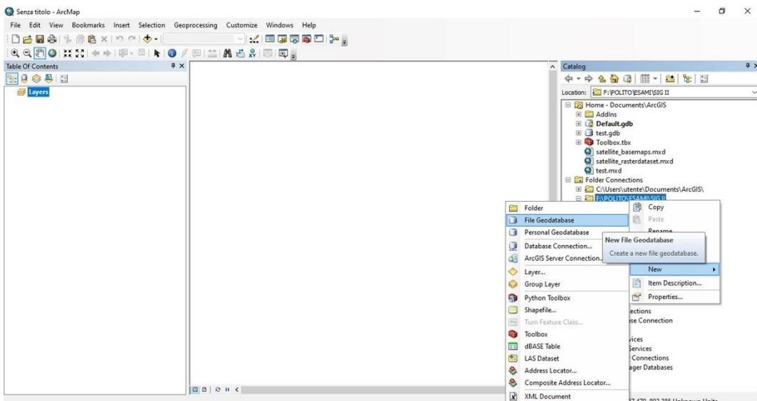
Figure 25. Creation of a new File Geodatabase using ArcGIS software.
