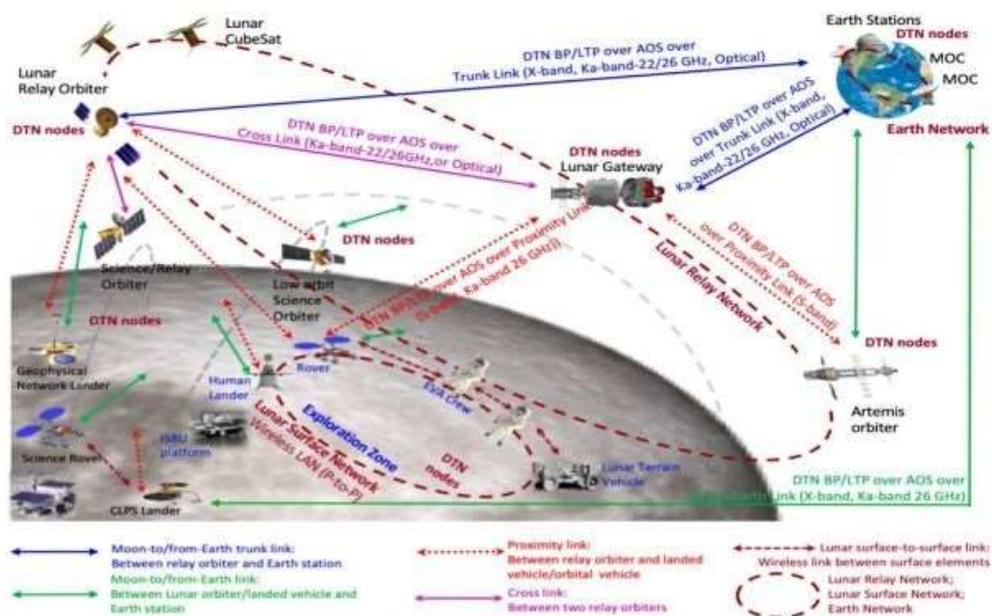
Fig 2.3.4 Communication Architecture by NASA (Credit: NASA)
