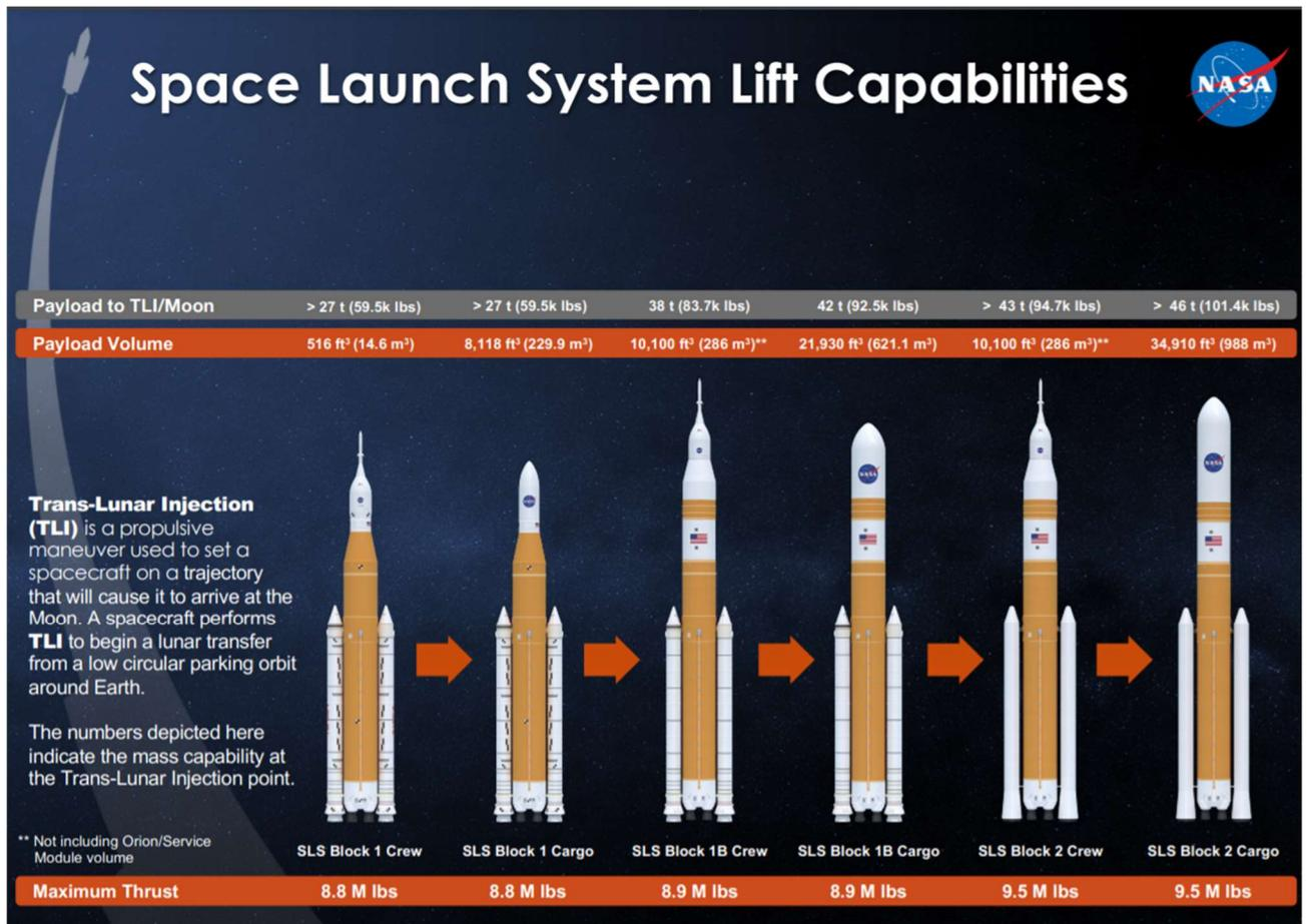
Fig 2.3.3-2 Resume of rockets capabilities (mass and volume) for each SLS version and configuration [14]
