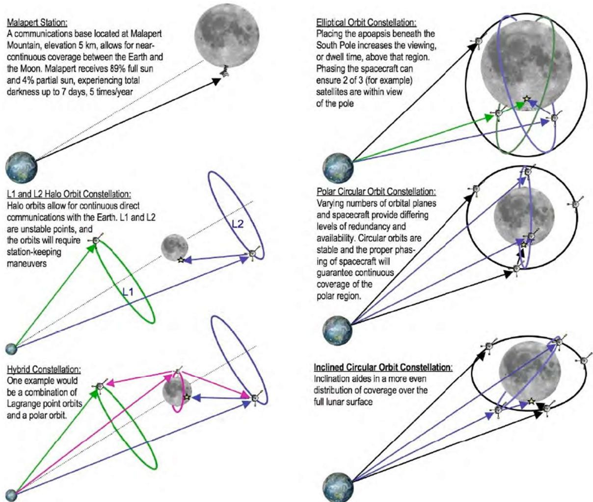
Fig. 7.1-1 Different satellite configuration studied by Kul B. Bhasin et al. [44]
