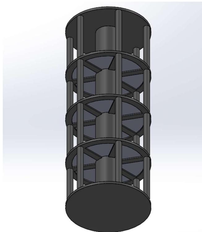
**Fig 4.4.1-1 Secondary Structure of habitable module**
