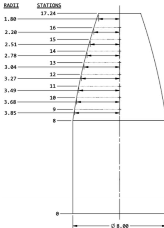
Fig. 2.3.3-6 Spaceship fairing envelope and dimensions [15]
