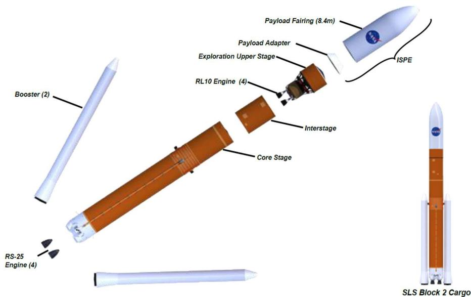
Fig 2.3.3-2 Reference configuration of Block 2 cargo version of rocket [13]
