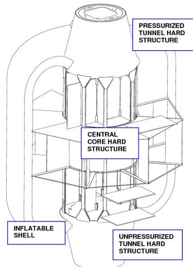
**Fig. 4.4-1 Detail of TransHab structural elements [27]**
