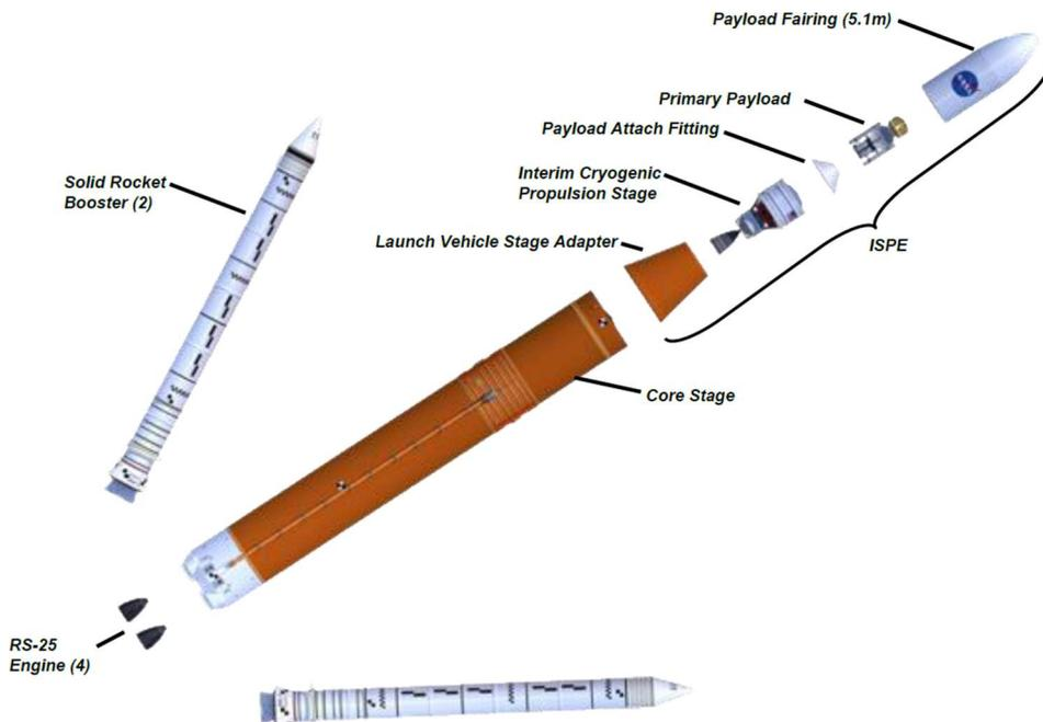
Fig. 2.3.3-1 Reference configuration of Block 1 rocket [13]
