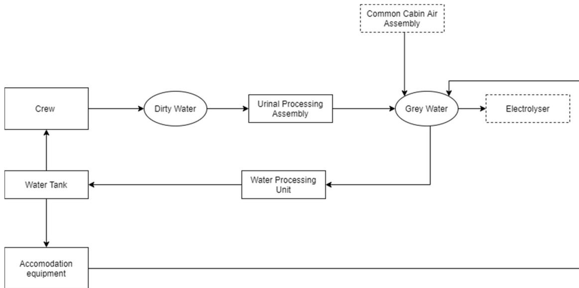
**Fig. 8.1.2-1 Water and wet waste sub-systems architecture**
