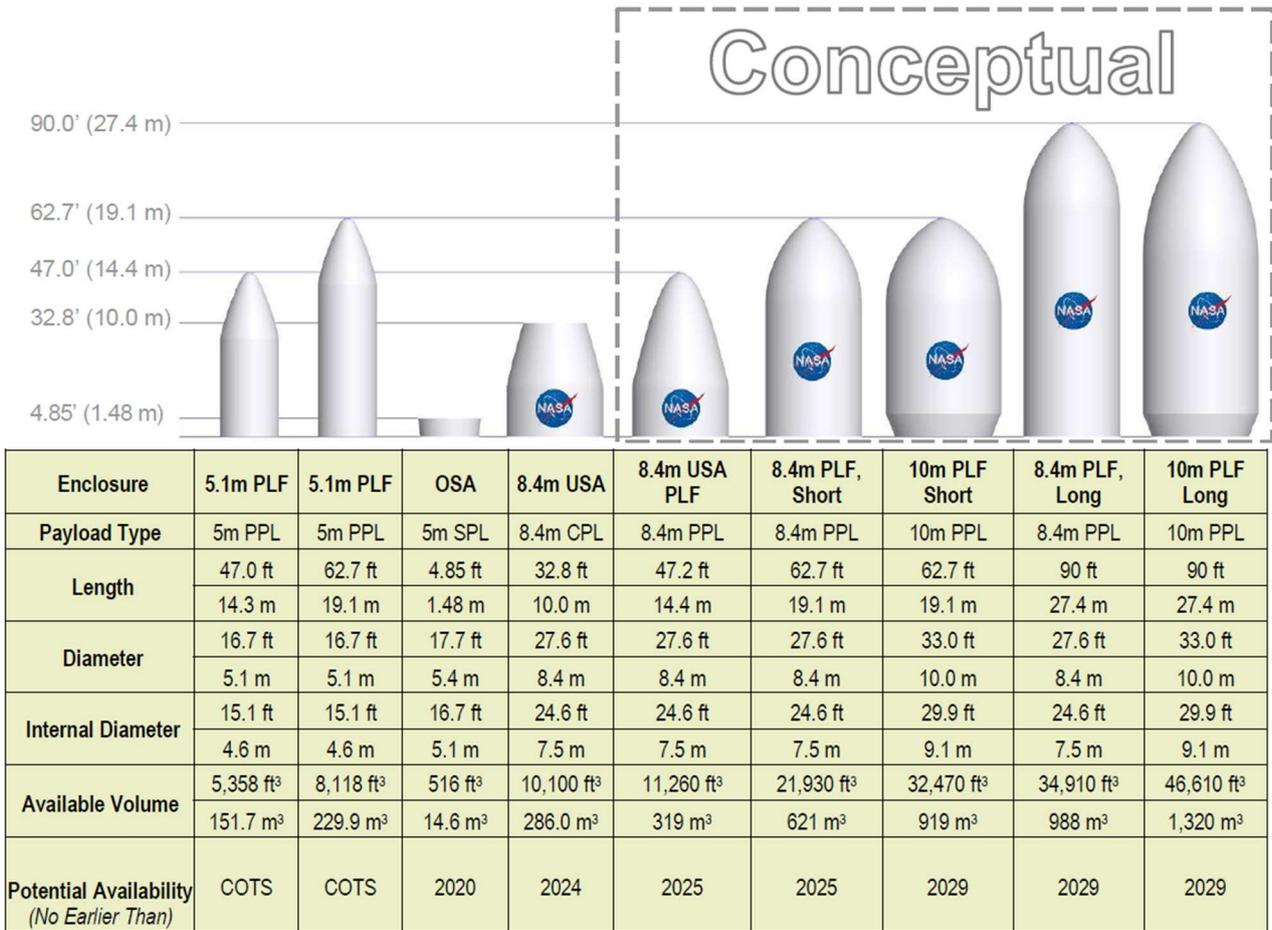
Fig. 2.3.3-3 Resume of possible fairing configurations for SLS [13]
