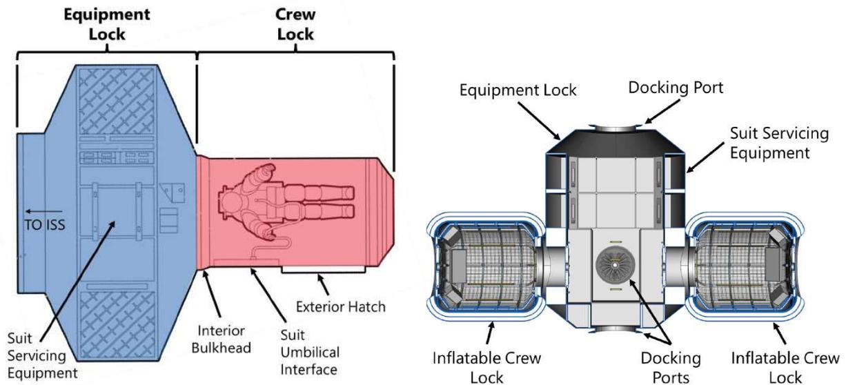
*ISS Joint Quest Airlock module diagram showing the dual-chamber design*
