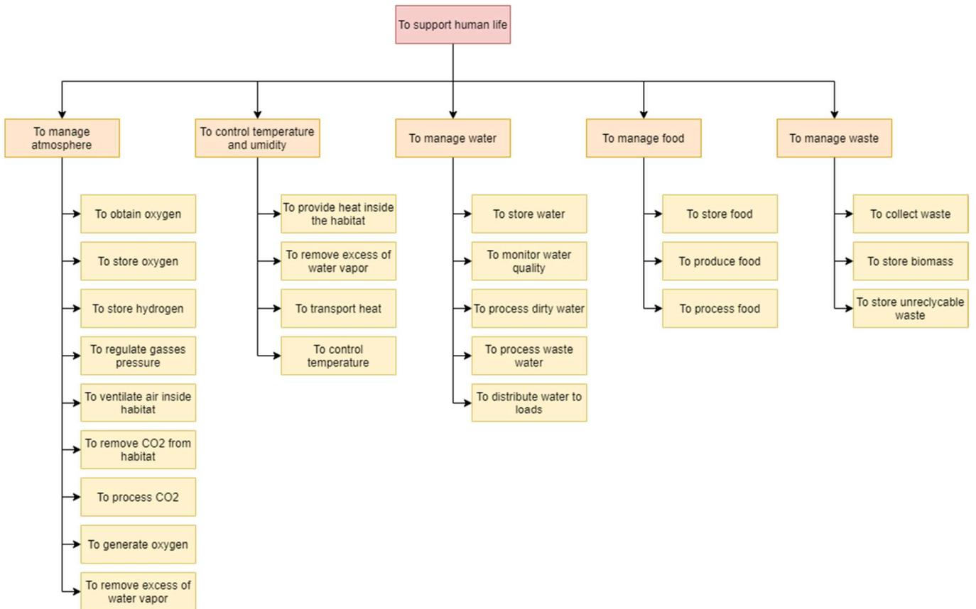
**Fig. 8.1-1 Functional Analysis of ECLS System**
