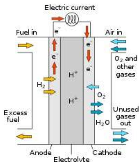
Fig. D.1-1 Detail of single fuel cell functioning (credit Wikipedia.org)
