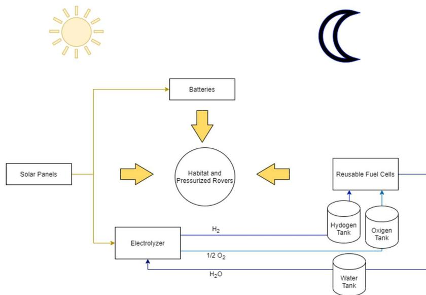
Fig. 6.2.1-1 Hybrid Power generation subsystem scheme
