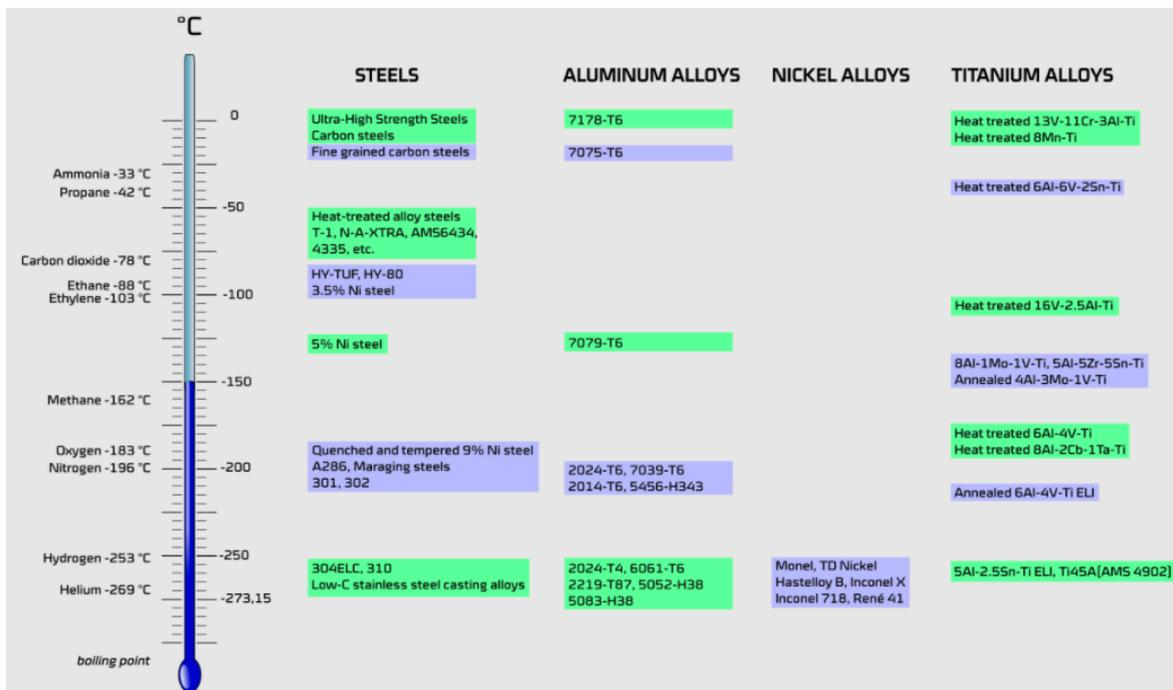
Figure 32 Materials resistant to extremely low temperatures. (Gasparini, 2019)
