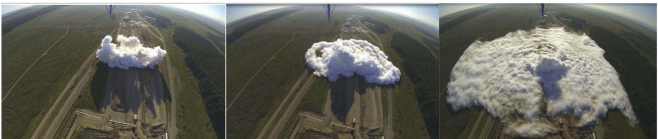
Figure 18. Images of the visible cloud resulting from the rupture of the pipeline, respectively at 10, 30 and 120 s from break [41].
