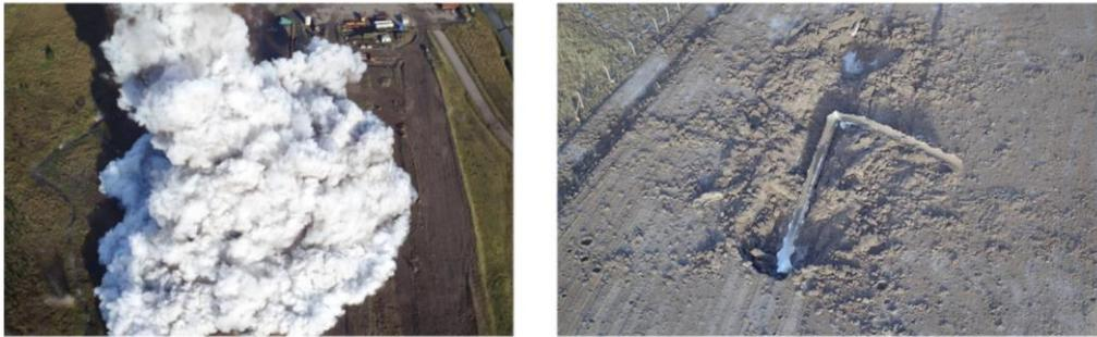
Figure 21. Spreading CO<sub>2</sub> cloud and crater and the fractured test section.
