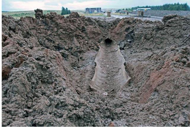
Figure 17. View of the crater formed during the instrumented burst.
