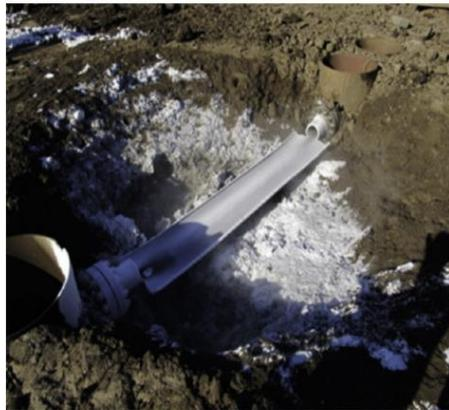
*Figure 25. Photo of the crater and a broken pipe in the COSHER [5].*
