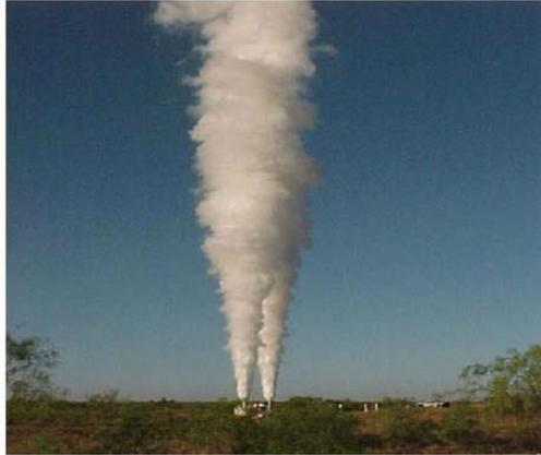
*Figure 23. Upward loss of  $\text{CO}_2$  from a pressurized vessel.*
