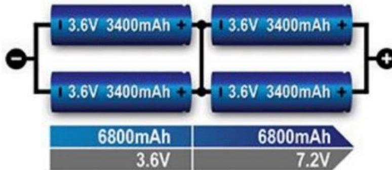
Figure 12: Example of connection of two cells in parallel and subsequently in series.
