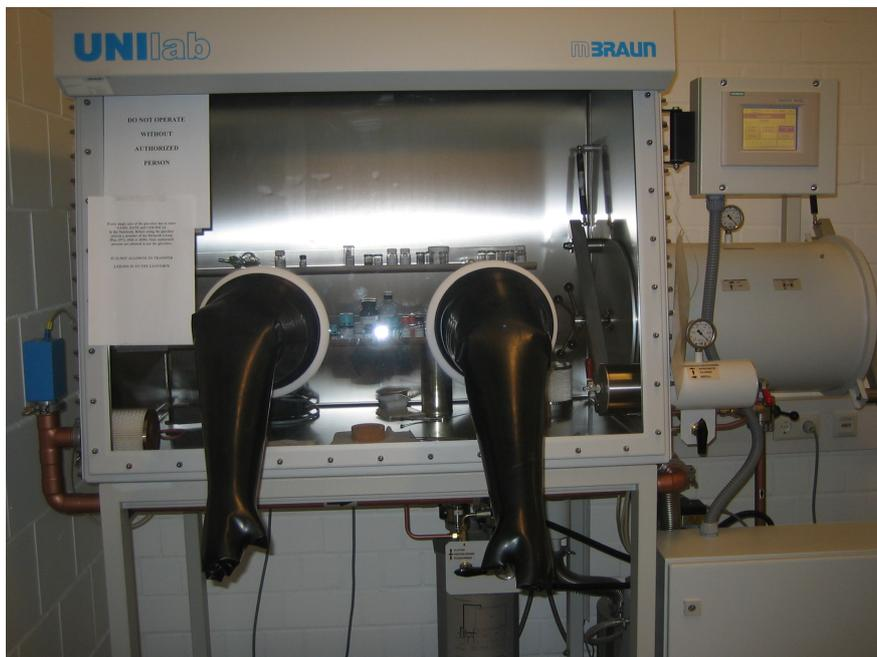
Figure 15: Example of a glovebox.
