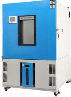
Figure 20: Example of a climatic chamber used for the controlled temperature tests.
