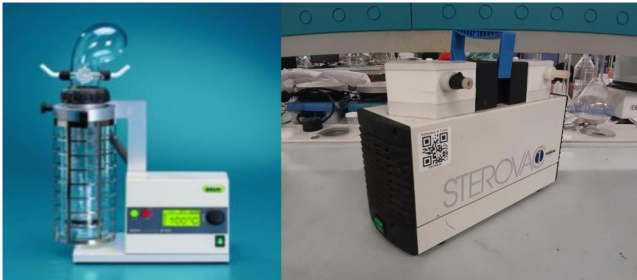
**Figure 2.1.2:** Büchi drying oven and vacuum pump.
