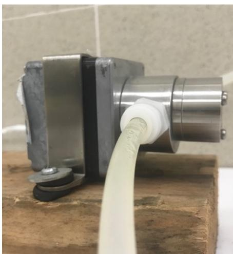
**Figura 4.4.** Pompe ad ingranaggi Fluid-o-tech (Magnet drive gear pump-motor units FG200/FG300 series).
