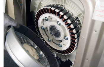
Figure 1.9: Direct Drive of a washing machine. [19]
