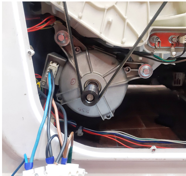
Figure 5.3: MUT3 Interior Permanent Magnet (IPM) motor used.
