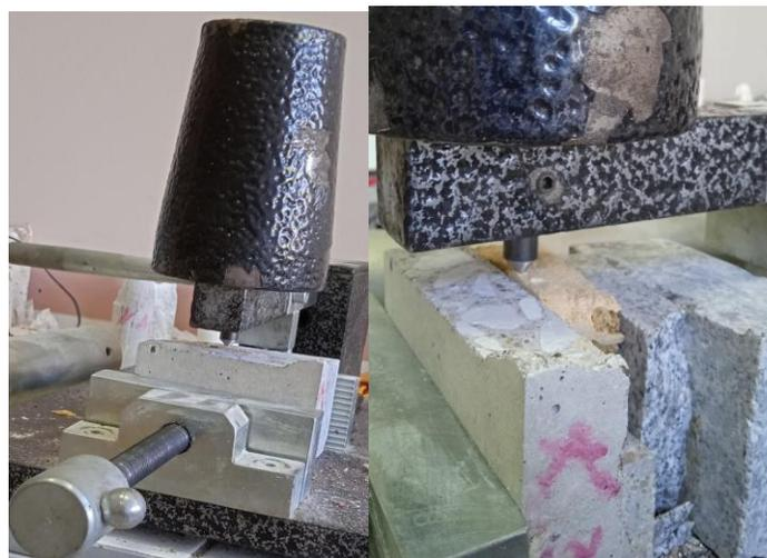
Figure 4.7. Cerchar abrasivity test equipment.
