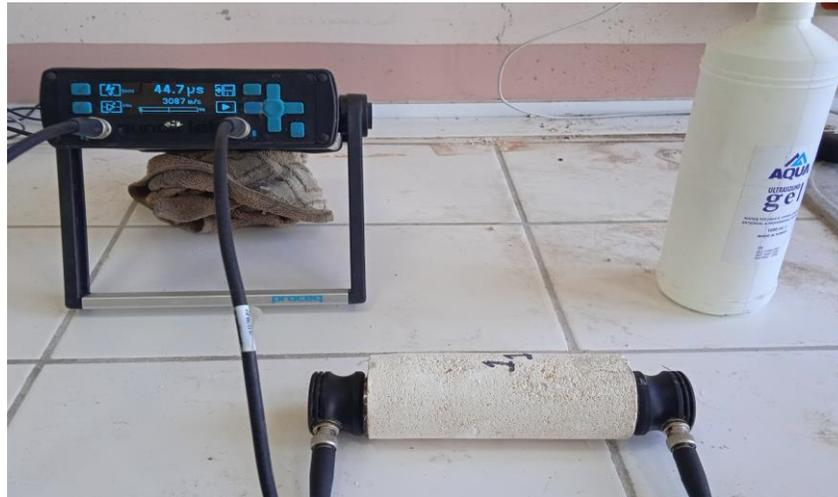
Figure 4.6. Determination of the ultrasonic velocity of the rocks by Pundit Lab (+).
