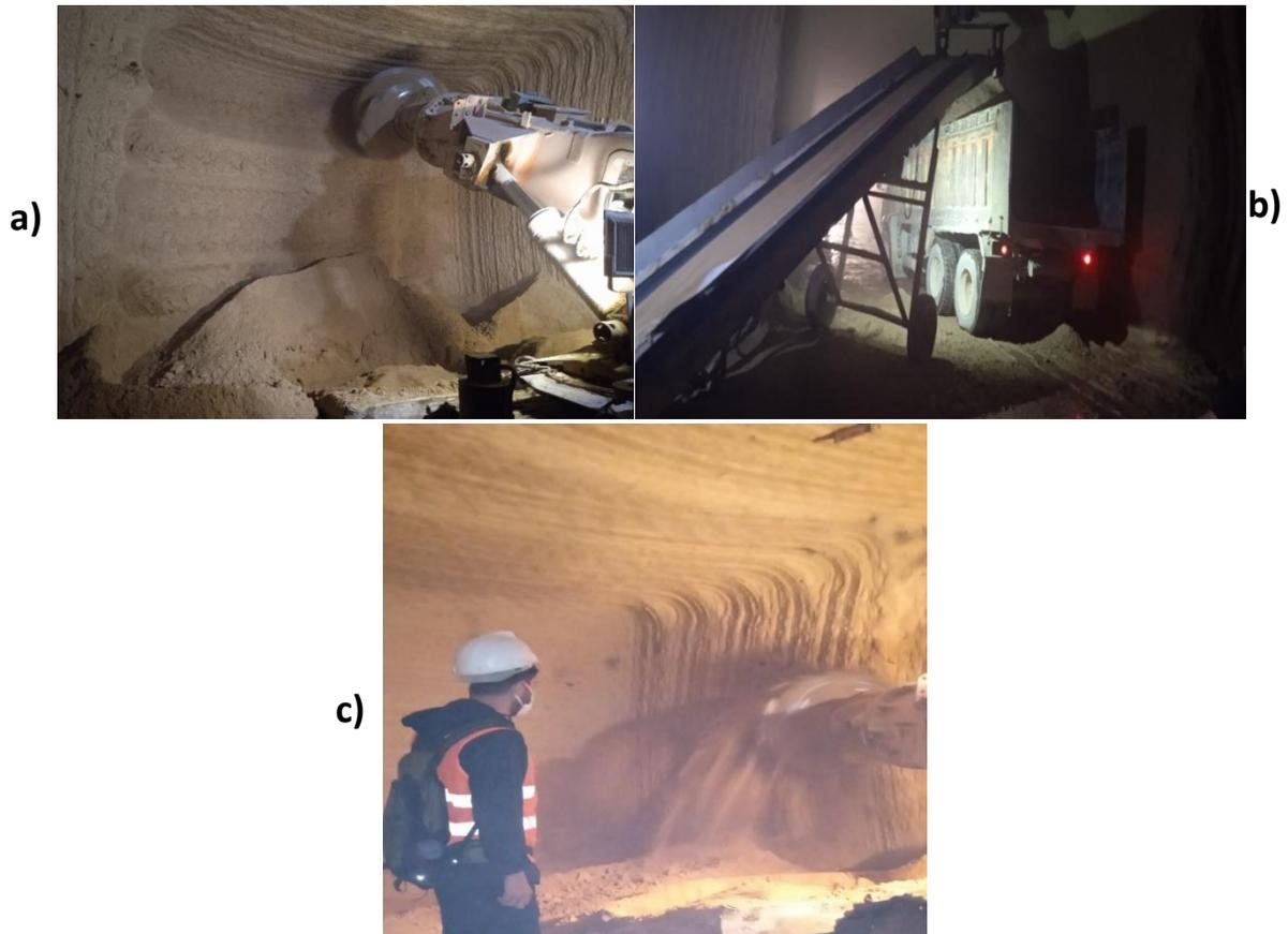
**Figure 5.9. a) Excavating b) Mucking c) Trimming.**
