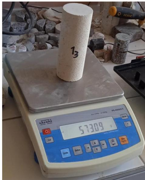
Figure 4.3. Evaluating the weight of specimens by electronic precision balance.
