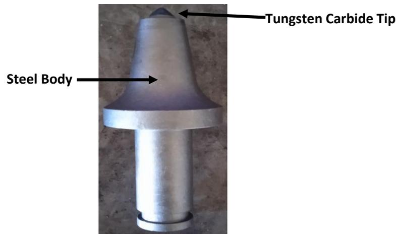
**Figure 5.10.** Conical cutter.
