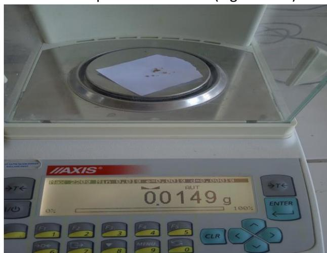
**Figure 4.13.** Electronic precision balance.
