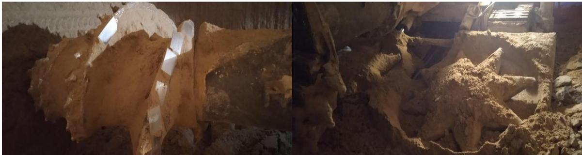
**Figure 5.7.** The adhesion of formation on the cutterhead and gathering arm.
