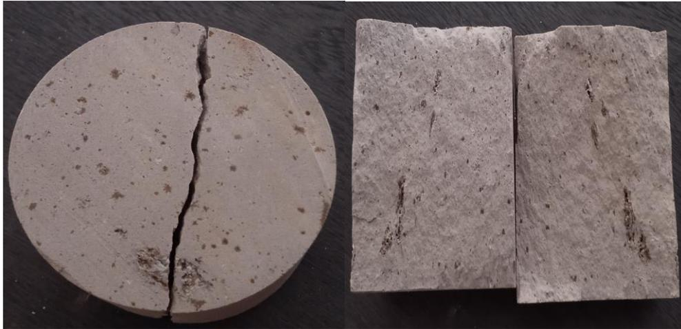
**Figure 4.8.** Rock specimens used for Cerchar abrasivity test.
