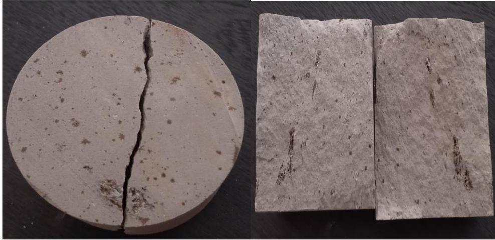
**Figure 4.8.** Rock specimens used for Cerchar abrasivity test.
