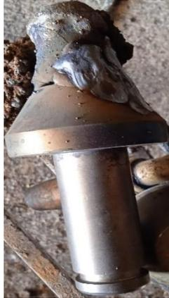
**Figure 5.12.** Welded steel body.
