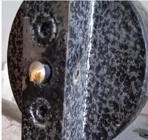
**Figure 4.12.** The adhered material on the tip of the pin.
