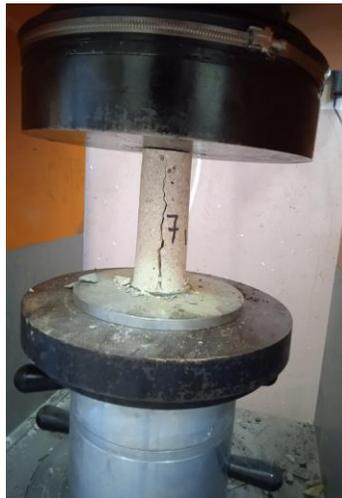
**Figure 4.4.** Hydraulic Press and specimen under analysis during the execution of the uniaxial compression test.
