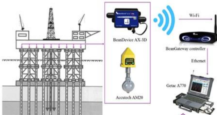
**Figure 32 : Robust noise monitoring system (combination of vibration and acoustic sensors) [82]**
