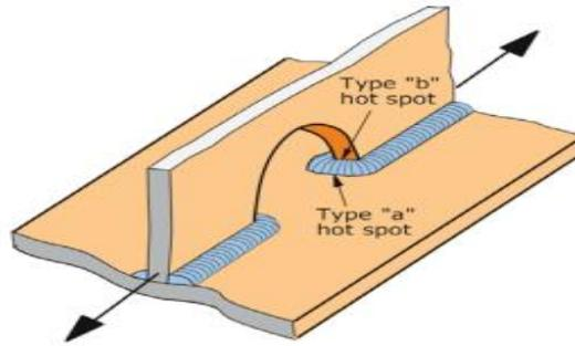
**Figure 10: Examples of two types of hot spots in the weld [41]**
