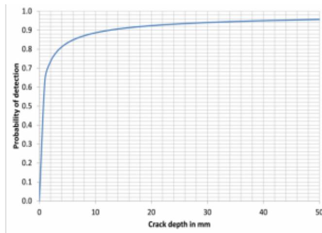
*Figure 18 : PoD for ultrasonic testing [54]*
