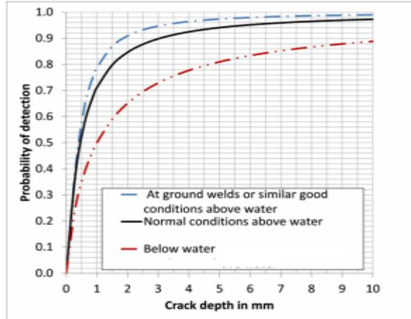
**Figure 20 : PoD Curves for MPI [54]**
