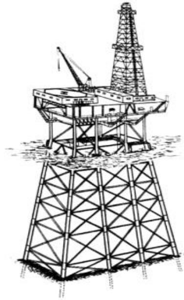
**Figure 3: Offshore jacket platform [24]**
