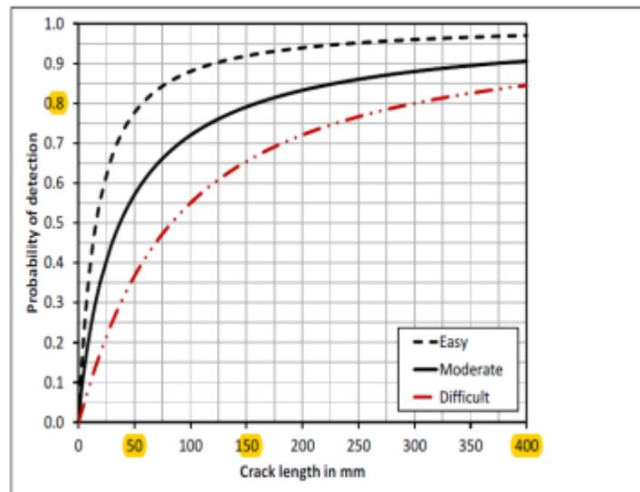
*Figure 15: PoD for Visual testing [54]*
