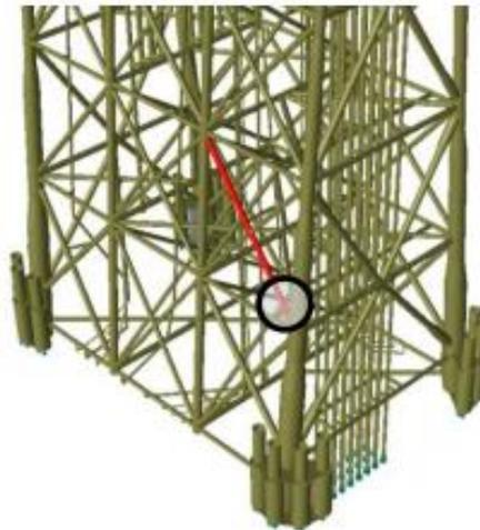
**Figure 28: Location of AE sensors in severed member [77]**
