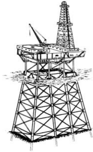
**Figure 3: Offshore jacket platform [24]**
