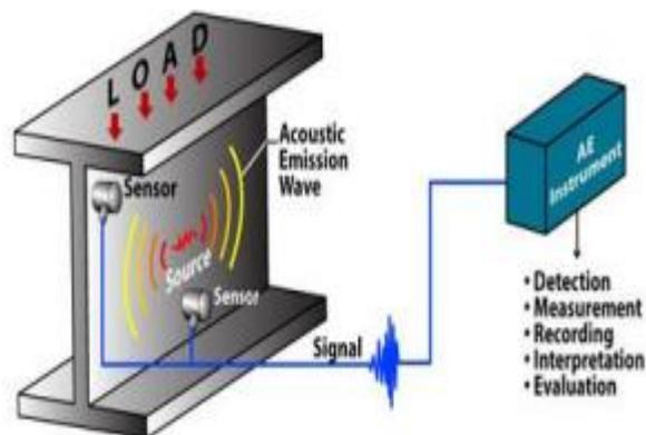
*Figure 23: Acoustic Emission technique [59]*
