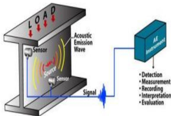
*Figure 23: Acoustic Emission technique [59]*
