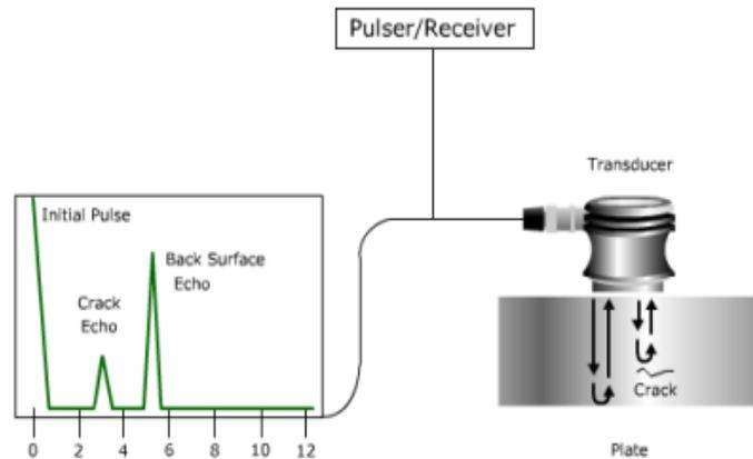
**Figure 16: Ultrasonic non-destructive technique [56]**
