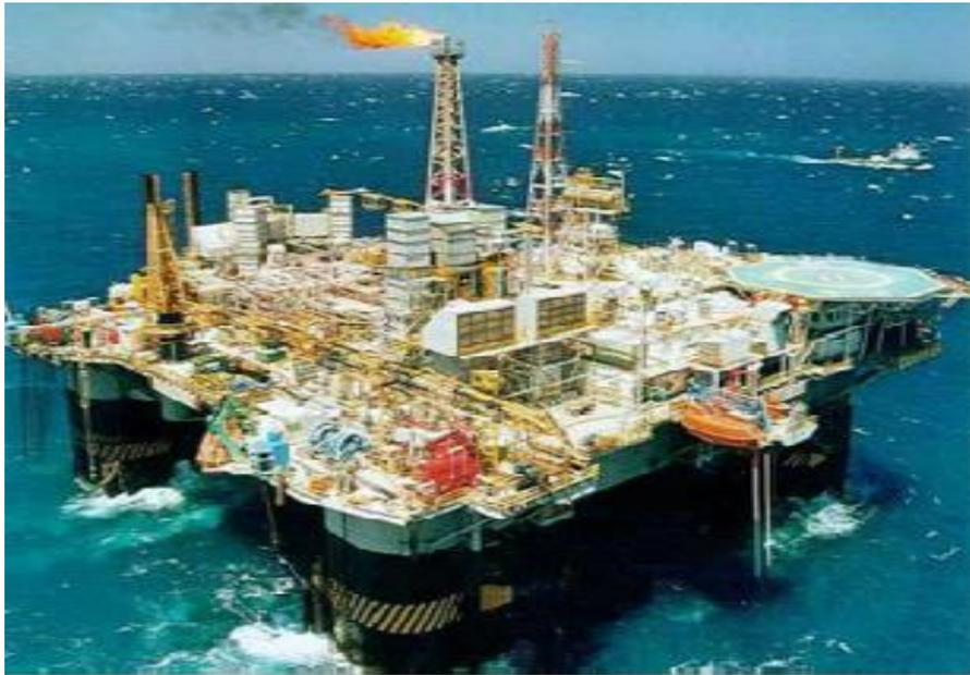
**Figure 5: semi-submersible platform [30]**
