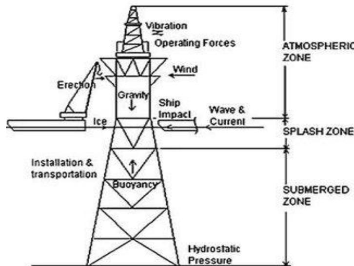
**Figure 7: Overview of loads on fixed offshore platform [34]**
