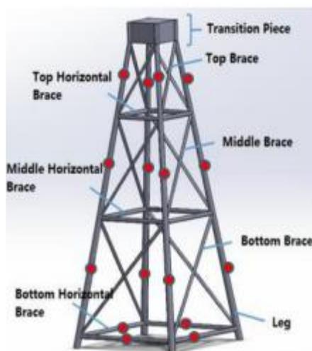
**Figure 30: Proposed installment of AE sensors inside legs members of the jacket J structure [80]**
