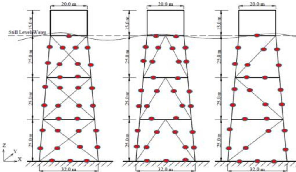
**Figure 29: Proposed installment of AE sensors on Jacket structure's surface [79]**
