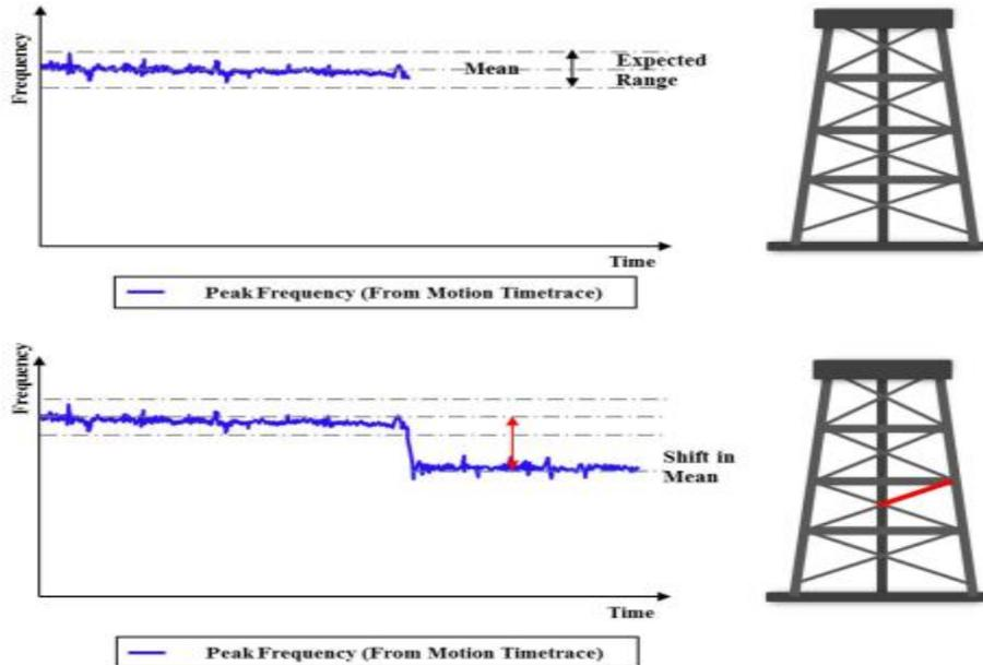
*Figure 27: Detection of loss of integrity using NFRM [71]*
