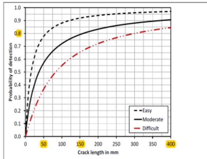
*Figure 15: PoD for Visual testing [54]*
