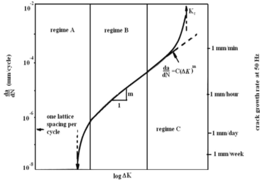
**Figure 9 : Different regimes of stable fatigue crack propagation [39]**
