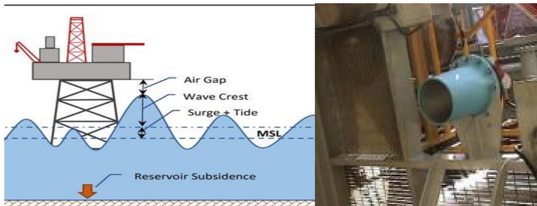
**Figure 24: Air Gap and air Gap sensor [65]**
