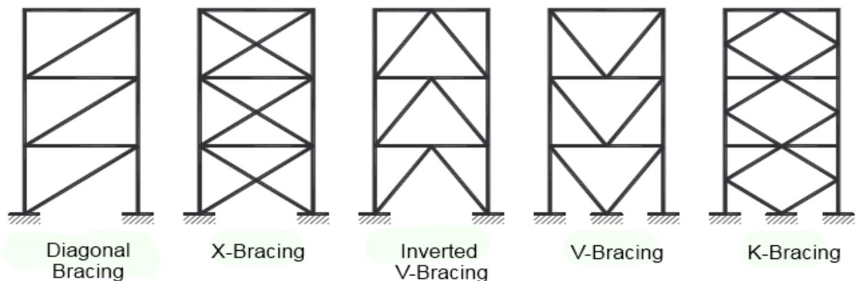
**Figure 4 : Bracing geometry for jacket structure [28]**
