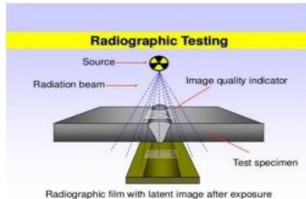
**Figure 22: Radiographic Testing [56]**
