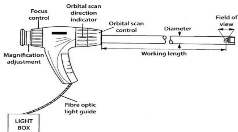
*Figure 13 :A typical 0° direct view borescope [51]*
