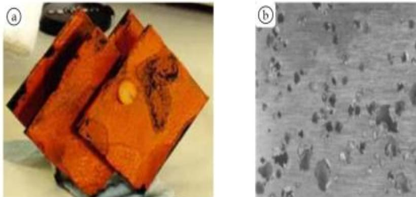
**Figure 12: a. uniform corrosion b. pitting corrosion [44]**
