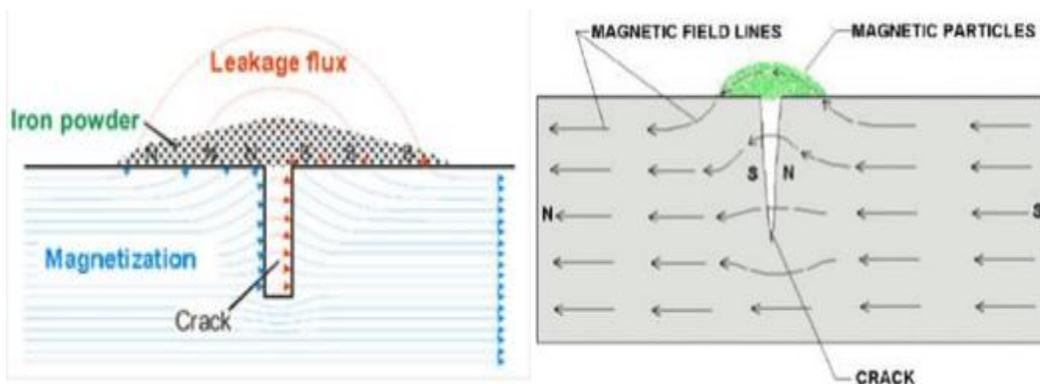
**Figure 19: Magnetic particle inspection [56]**
