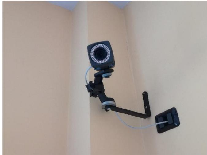
*Figure 5.3 – Telecamere ad infrarossi VICON*
