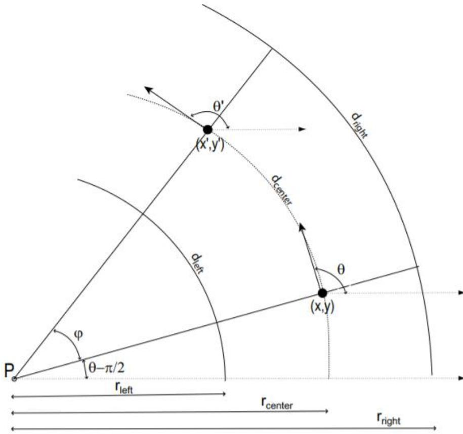
Figure 2: Detailed odometry geometry. We compute the center of the circle  $P$  by forcing  $d_{left}$  and  $d_{right}$  to be two arcs with the same inner angle  $\varphi$ . From this, we can compute the new robot position  $(x', y', \theta')$ .
