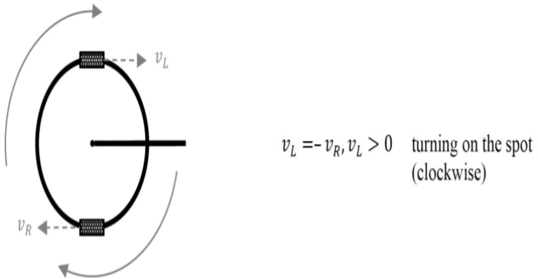
Figure 8: Rotation of differential drive
