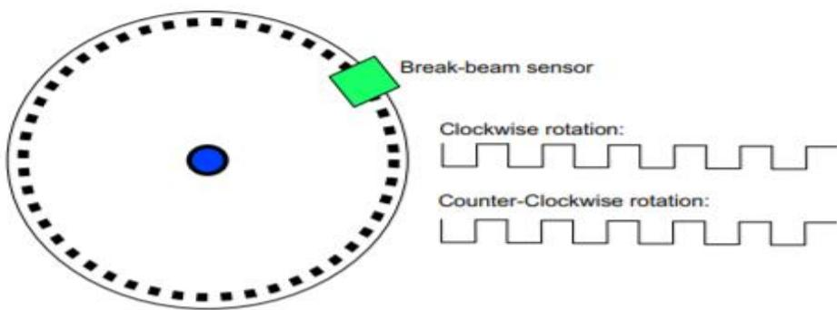
Figure 3: Simple Encoder. As a perforated disk rotates, a break beam sensor alternates between 1 and 0. The direction of motion is ambiguous.
