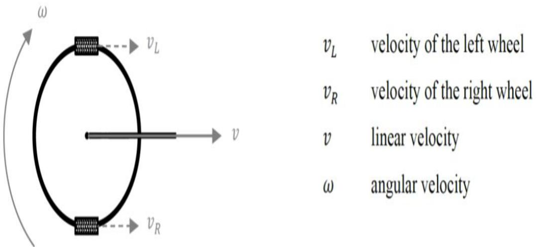
Figure 9: Linear Velocity, Angular velocity, and Driven Wheel Velocities
