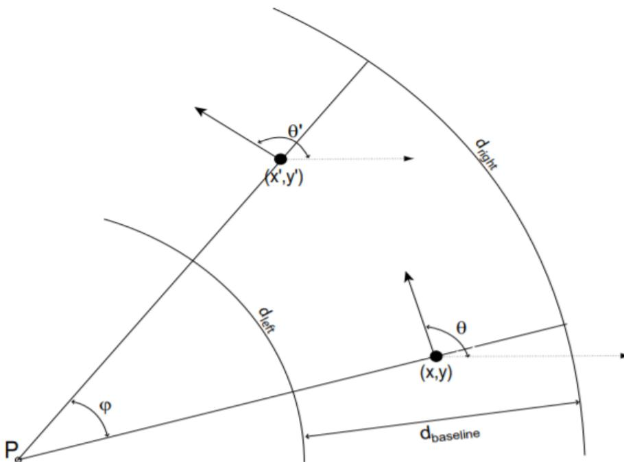
Figure 1: Odometry geometry. Over a small time period, the robot's motion can be approximated by an arc. The odometry problem is to solve for  $(x', y', \theta')$  given  $(x, y, \theta)$  and  $d_{baseline}$ . In the figure, the robot is moving counterclockwise.
