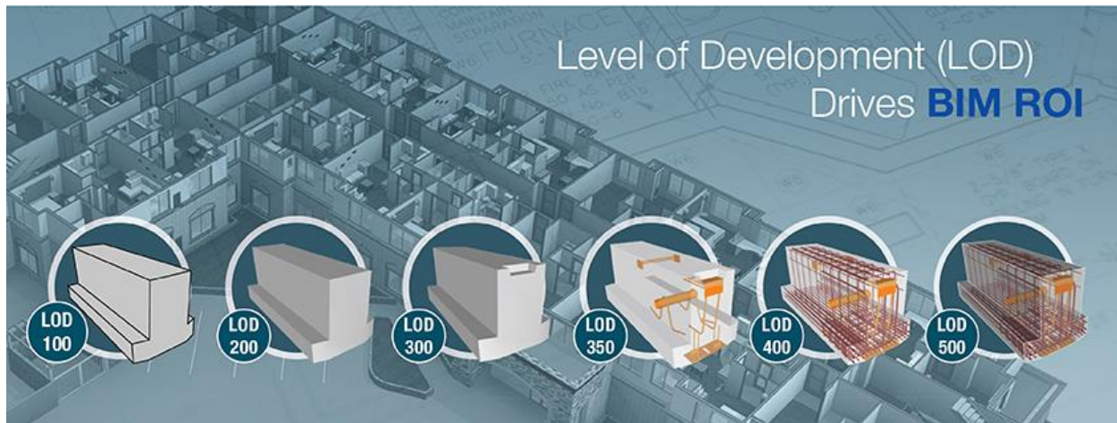
Figure 3: Level of Development LOD [Source: https://www.hitechcaddservices.com/bim/support/level-of-development-lod/ ]
