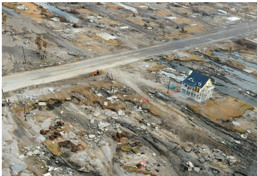
Figure 1-1, A home in Gilchrist, Texas, designed to resist flood waters survived Hurricane Ike in
