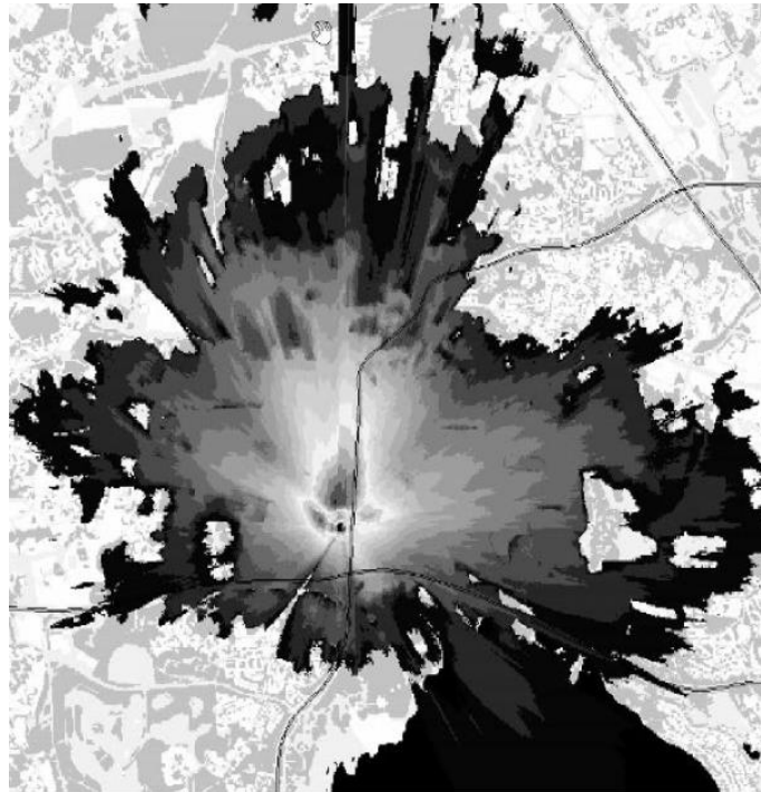
Figure 3-30, example of a coverage area of a real cell
