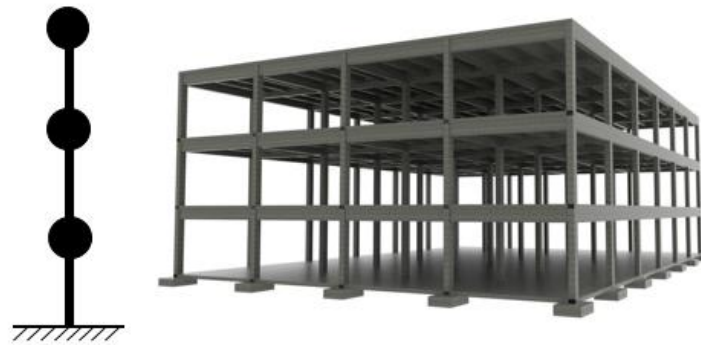
Figure 6-1, MDOF model for RC buildings used to define the Physical properties
