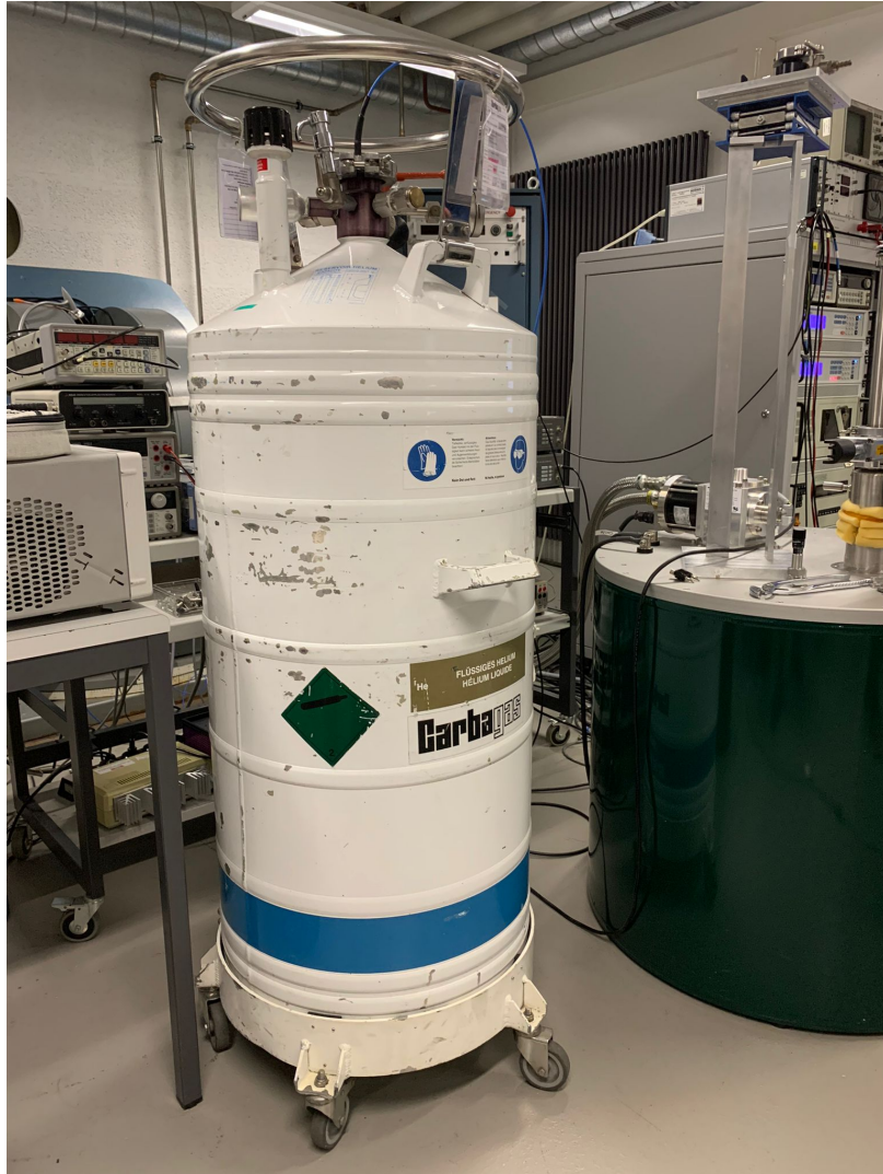
Figure 28: Photo of the cryogenic system. In the center : the Dewar with on top an RF cable exiting from the flange.
