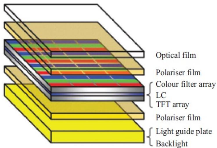
Source : Shoichi Ishihara et al., (2019), “High Quality Liquid Crystal Displays and Smart Devices”, volume 1: Development, display applications and components.
