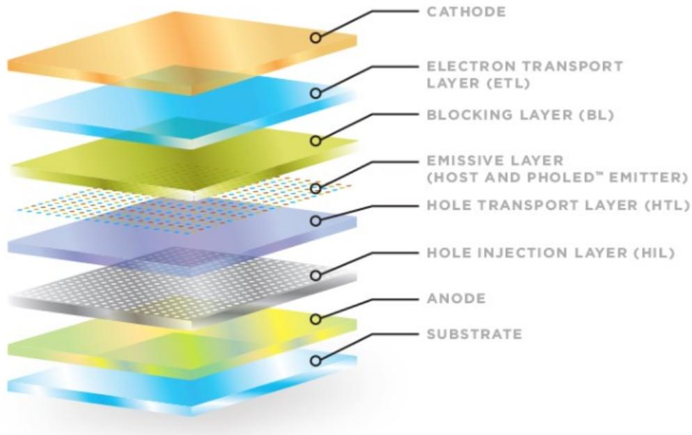
Source: Organic Light Emitting Diodes (OLEDs), Available at: <https://oled.com/oleds/>
