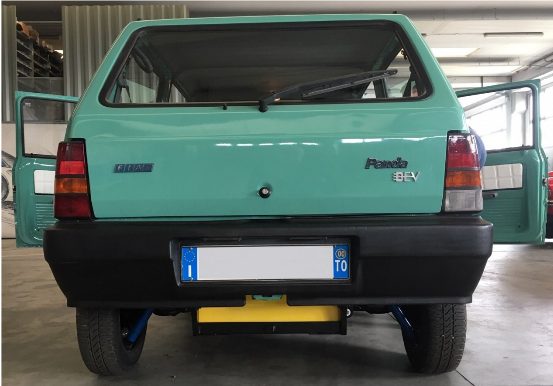
Figure 16 : HV Battery placement under rear underbody (battery coloured in yellow)
