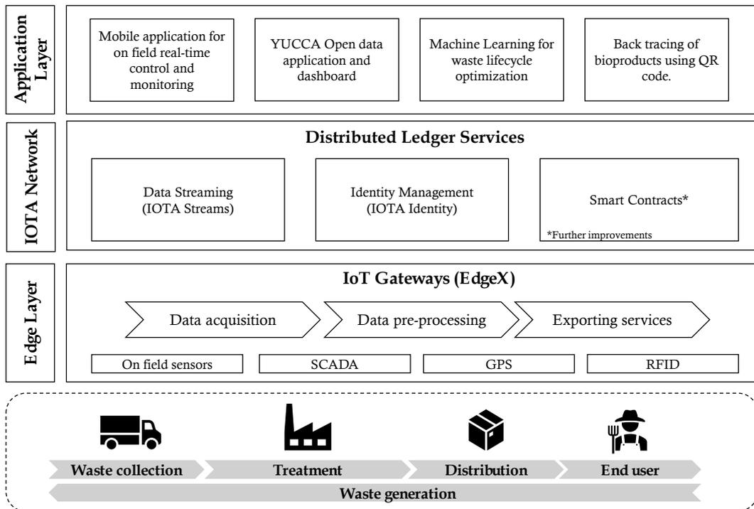
**Figure 6.1:** BioEnPro4To Architecture.
