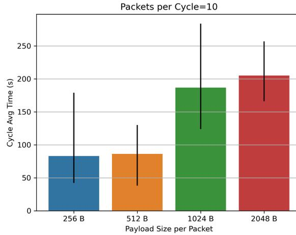
**Figure 7.2:** Minimum, Maximum and Average value of cycles publishing time for each payload size.
