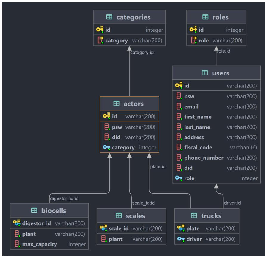
Figure 6.12: UML diagram of the entity relationships.
