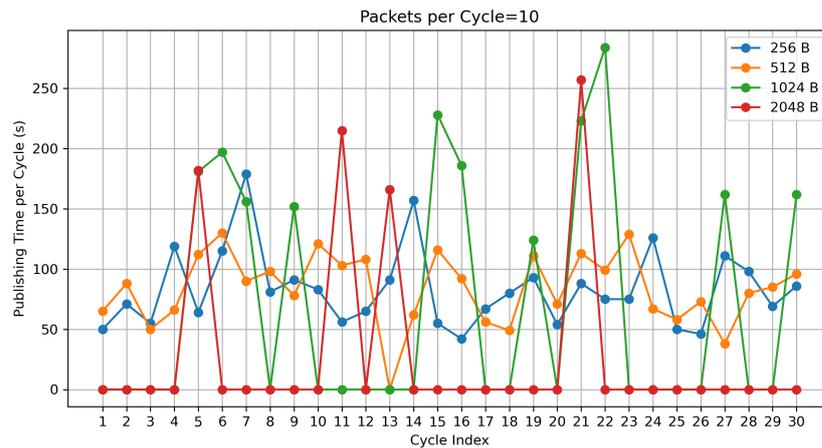
**Figure 7.3:** Cycles publishing times trend for each payload size. The zero values refer to cycles that have been interrupted due to timeout expiration.
