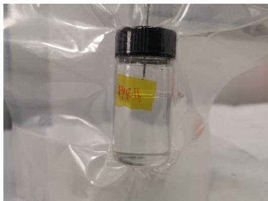
Figure 4.4 Vacuum packaged [PYR14][TFSI]
