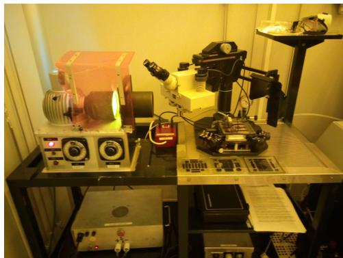
**Figure 6.2:** Set-up of the photolithographic process with the UV source, into a class 100 clean-room.
