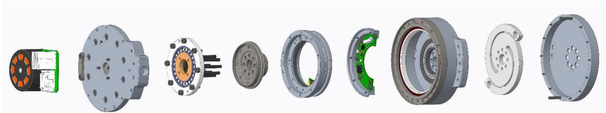
Figure 33: SEA configuration: EC45 motor with SPT1P compliant element, focus on each SEA component disassembled, BLDC motor, Harmoni Drive, mirrored Encoders, and compliant element
