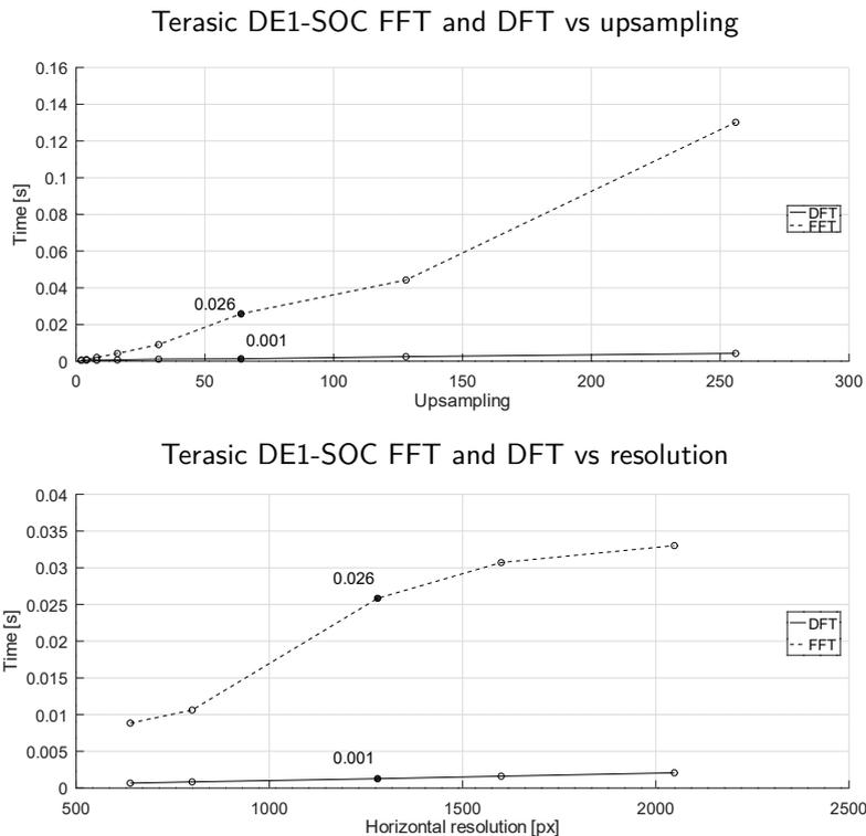
Figure 5.2: Terasic DE1-SoC displacement computation time using FFT and DFT implementation. The marked points have resolution  $1280 \times 960$  and upsampling factor 64.
