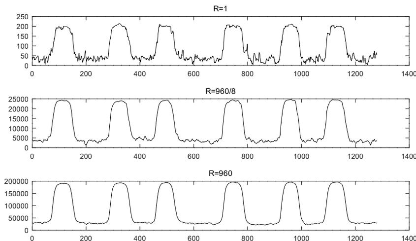
Figure 2.6: Frame vector computed with different  $R$  values. Resolution  $1280 \times 960$ .
