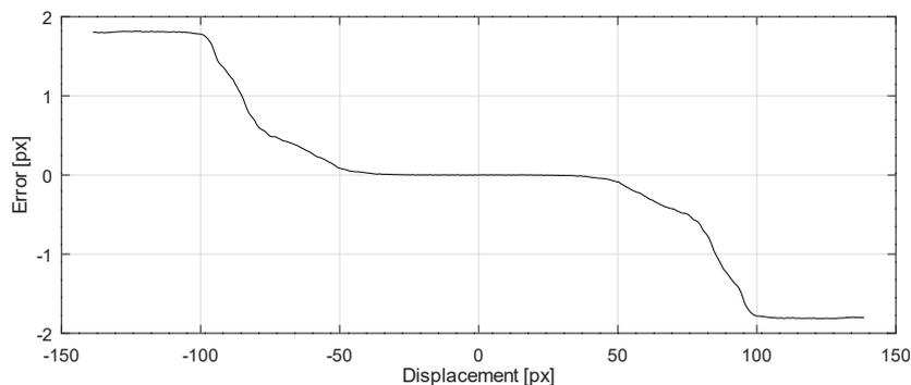
Figure 2.13: Difference between the computed displacement and the shift of the image. Frames with 640 horizontal resolution.
