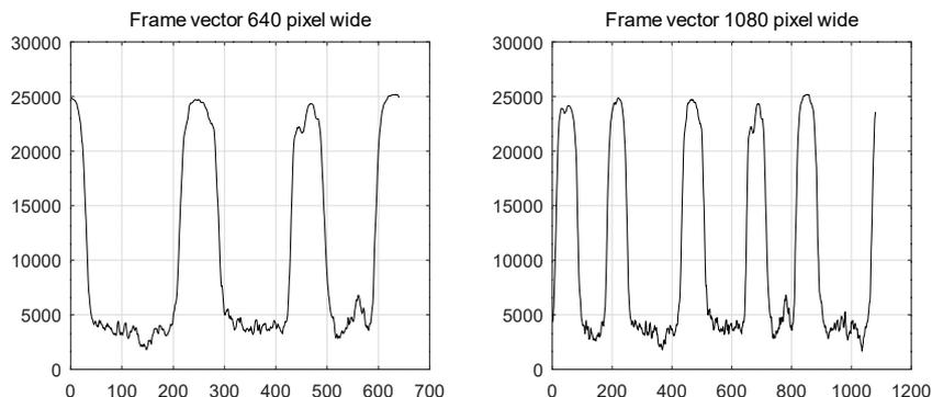
Figure 2.10: On the left the vector of the frame with the same width of a set of bands. On the right the vector with width larger different from an integer set of bands.
