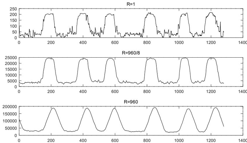
Figure 2.8: Frame vector of the tilted frame computed with different  $R$  values. Resolution  $1280 \times 960$ .
