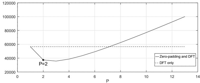
Figure 2.21: Comparison of the complexity of the zero-padding & DFT method and of the DFT approach. Resolution  $800 \times 600$  and upsampling 32
