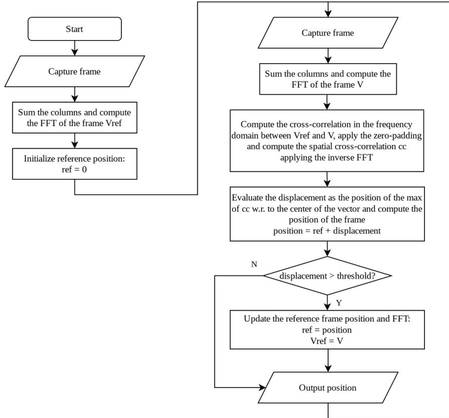
Figure 2.1: Flow chart FFT and zero-padding method.
