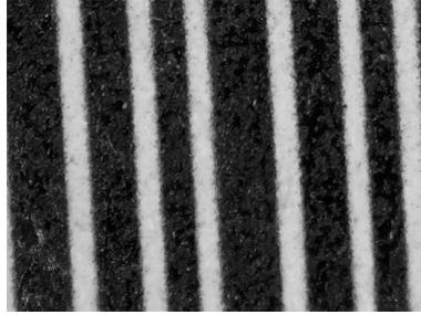
Figure 2.7: Frame with tilted bands due to the object moving and rolling shutter sensor
