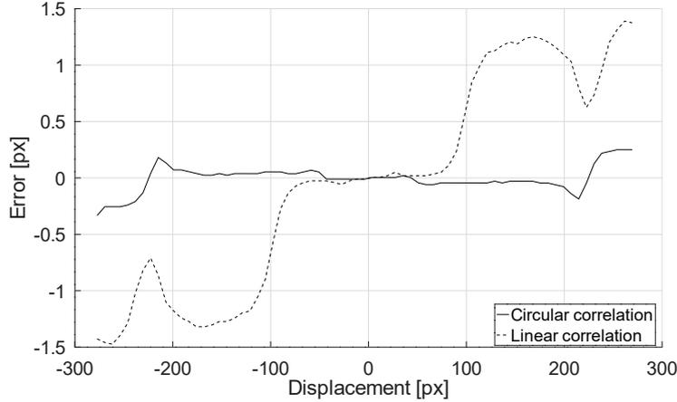
Figure 2.9: Error of the displacement computed with correlation with respect to the expected displacement. Resolution  $1280 \times 960$  and upsampling 64.
