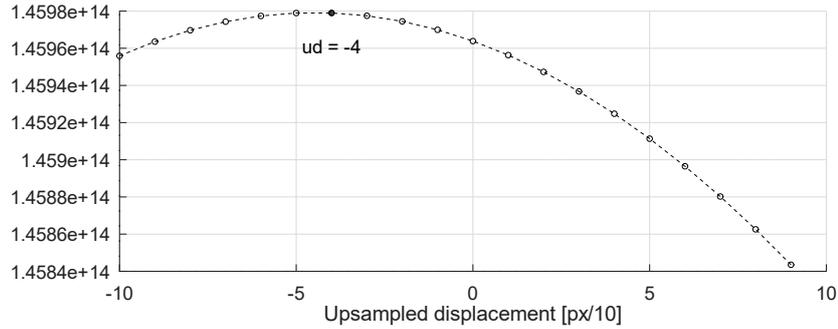
Figure 2.20: Upsampled spatial cross-correlation around the peak with upsampling factor 10. The additional upsampled displacement is  $-4/10$  pixels.
