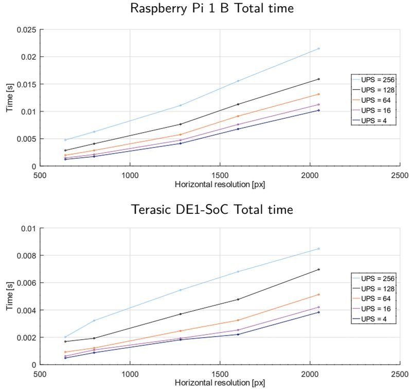
Figure 5.7: Total time (sum of the columns time plus displacement time) against the resolution for different upsampling factors UPS. The sum of the columns is computed using 1/8 of the rows.
