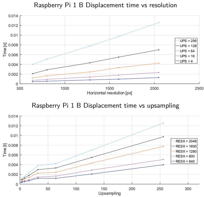
Figure 5.4: Raspberry Pi 1 B displacement computation time using different resolutions RESX and upsampling factors UPS
