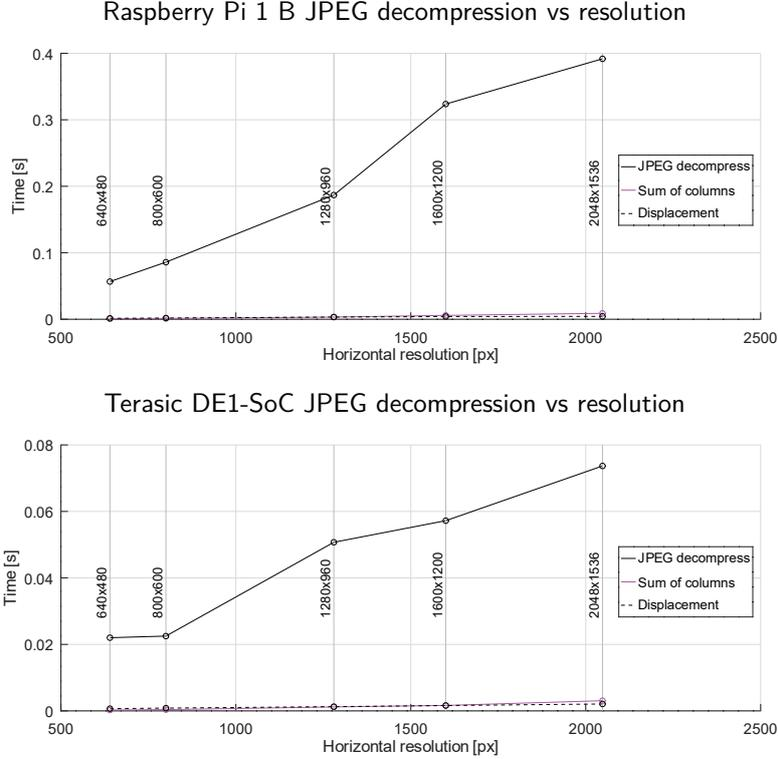
Figure 5.8: JPEG decompression time against the resolution. The sum of the columns using 1/8 of the rows and the displacement with upsampling 64 are shown for comparison.
