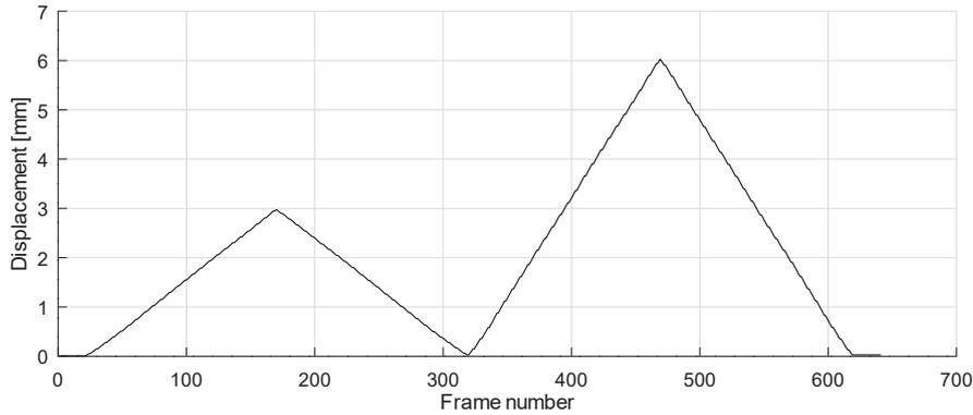
Figure 4.5: Large movements test, displacement computed in millimeters with upsampling factor 256 and resolution  $640 \times 480$
