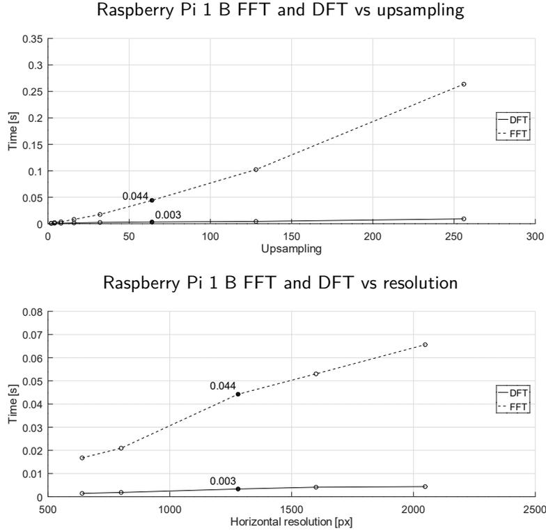
Figure 5.1: Raspberry Pi 1 B displacement computation time using FFT and DFT implementation. The marked points have resolution  $1280 \times 960$  and upsampling factor 64.
