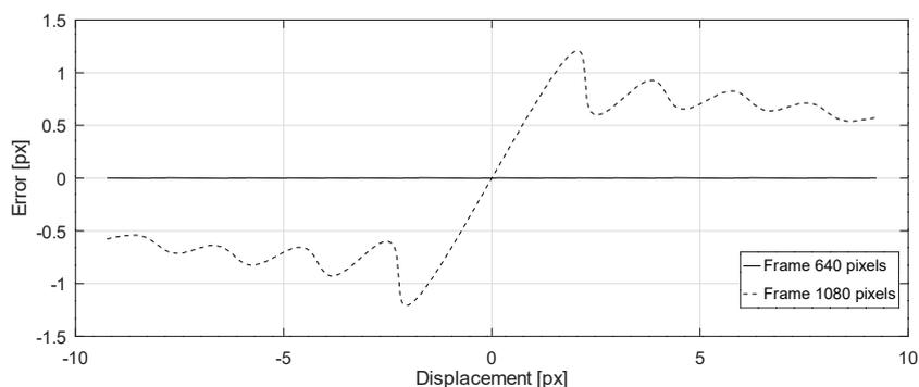
Figure 2.11: Difference between the computed displacement and the shift of the images. The continuous plot is computed using frames with the same width of a set of bands (640 pixels), while the dashed one uses frames with larger width (1080 pixels).
