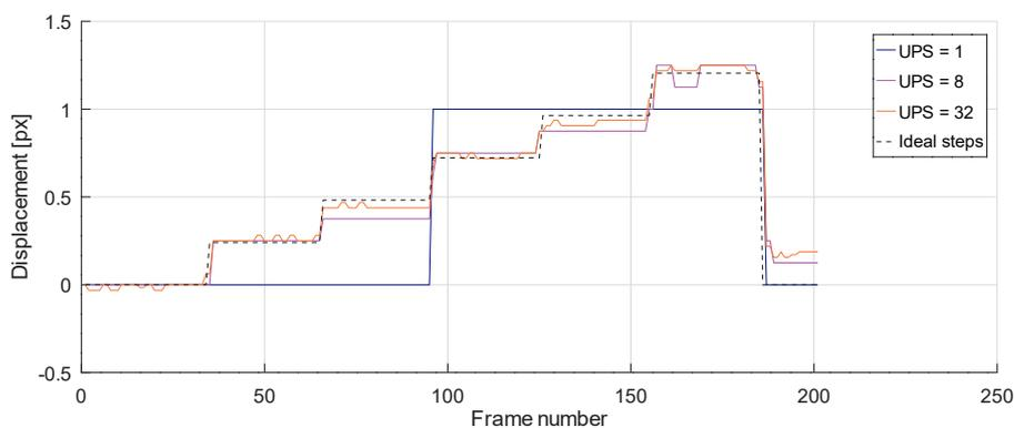
Figure 4.3: Sub-pixel test, displacement computed in pixels with resolution  $640 \times 480$  and using different upsampling factors UPS
