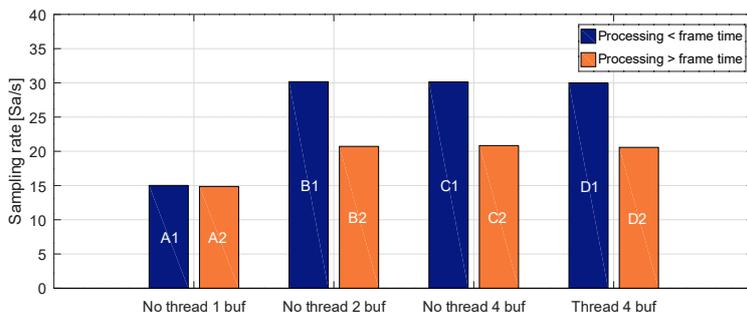
Figure 5.9: The blue columns (X1) show the sampling rate with the processing time is smaller than the frame time, the orange columns (X2) show the sampling rate with the processing time larger than the frame time.
