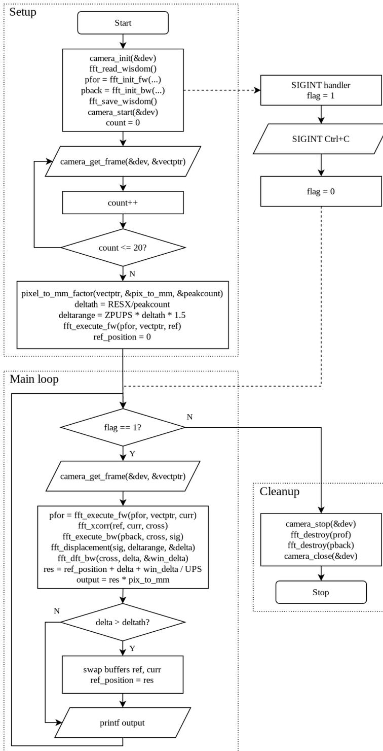
Figure 3.2: Flow chart of the main of the program and the function calls
