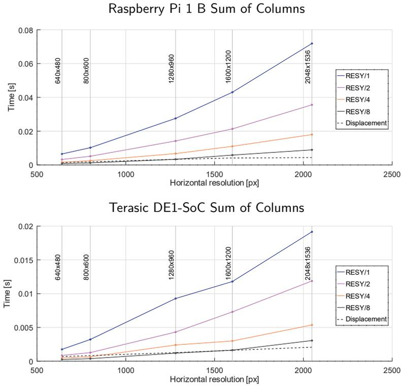
Figure 5.6: Sum of columns time against the upsampling factor using different resolutions. A variable number of rows is added, defined as fraction of the vertical resolution **RESY**. The displacement is evaluated with upsampling 64.
