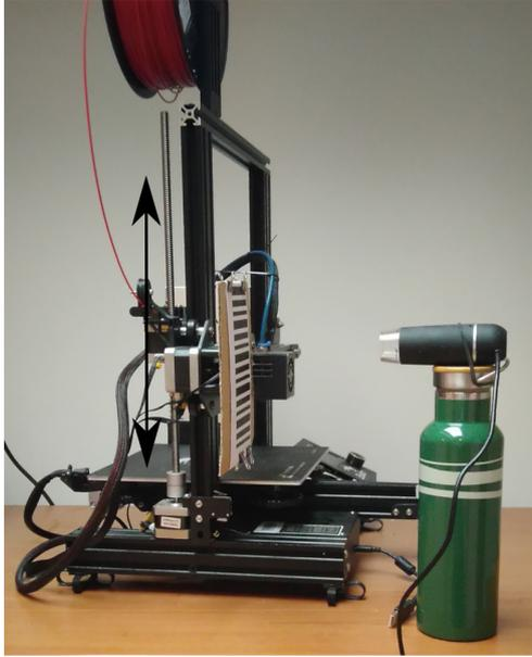
Figure 4.2: USB microscope and 3D printer setup during the sub-pixel testing
