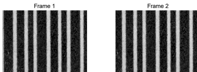
Figure 2.2: Example of captured frames with resolution  $1600 \times 1200$  and shift 81.7 pixels
