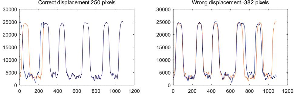
Figure 2.16: Frame vectors aligned in the expected position (left) and in the wrongly computed displacement (right)
