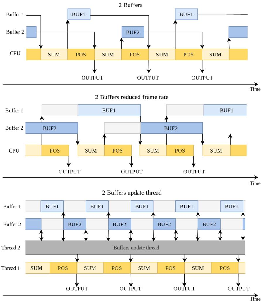
Figure 3.4: Flow diagram comparing the program behavior when the computation time is longer than the frame time using 2 frame buffer (top), 2 frame buffers and reducing the frame rate (middle) and 2 frame buffers with a thread constantly refreshing the frames (bottom).
