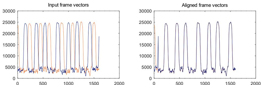
Figure 2.3: Vectors obtained as the sum of the columns of the frames. The left plot shows the original vectors, the right plot shows the vectors aligned in position corresponding to the maximum of the cross-correlation.
