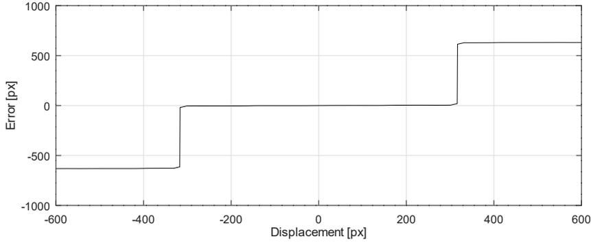
Figure 2.14: Difference between the computed displacement and the shift of the image. Frames with 1200 horizontal resolution.
