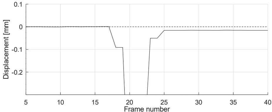
Figure 4.1: Position of the Z axis when moving down and up 1 mm. The position on the right half is  $-0.016 \text{ mm}$ .
