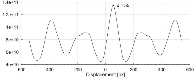
Figure 2.19: Non-upsampled spatial cross-correlation. The computed pixel displacement is 55 pixels.
