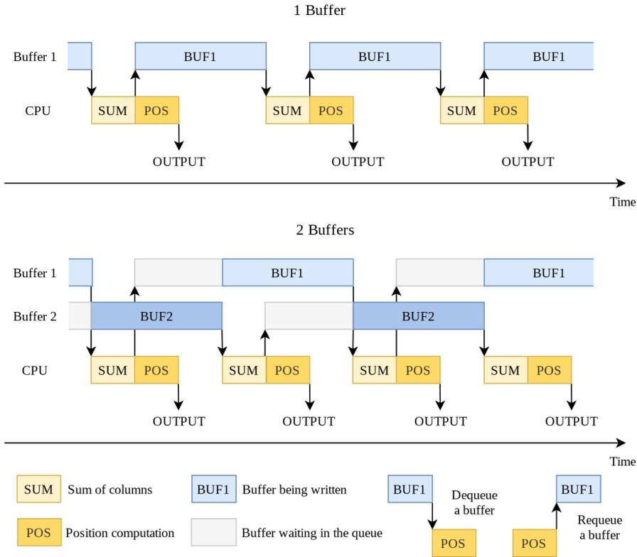
Figure 3.3: Flow diagram comparing the program behavior when using 1 frame buffer (top) or 2 frame buffers (bottom) when the computation time is shorter than the frame time
