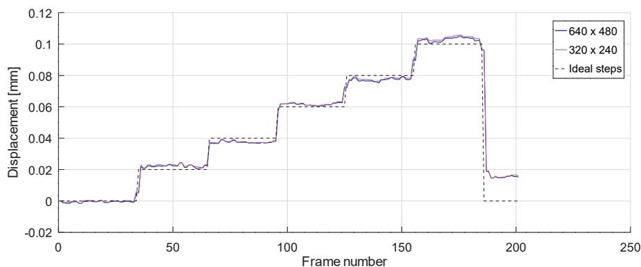
Figure 4.4: Sub-pixel test, displacement computed in millimeters with upsampling factor 256 and resolutions  $640 \times 480$  and  $320 \times 240$  (obtained downscaling  $640 \times 480$ )
