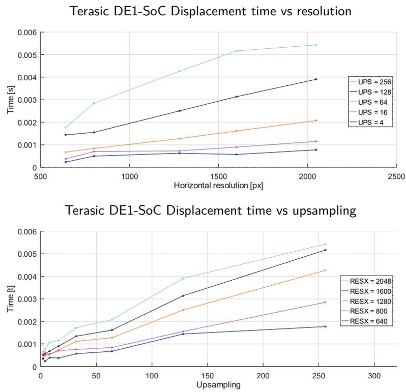
Figure 5.5: Terasic DE1-SoC displacement computation using different resolutions RESX and upsampling factors UPS
