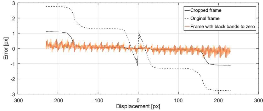
Figure 2.15: Difference between the computed displacement and the shift of the image. Frames with 1080 horizontal resolution.
