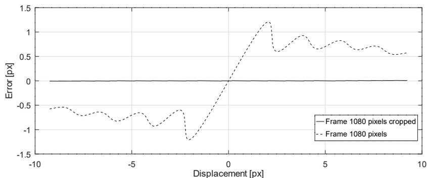
Figure 2.12: Difference between the computed displacement and the shift of the images. The continuous plot is computed using the 1080 pixel frames cropped to the same width of a set of bands, while the dashed one uses the full 1080 pixels frames.
