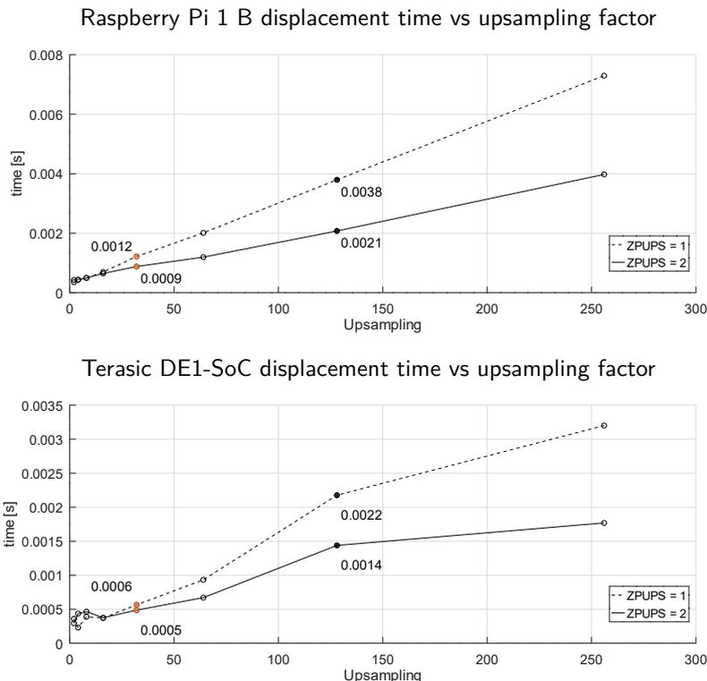
Figure 5.3: Displacement computation time with zero-padding factors ZPUPS 1 and 2. The resolution is  $640 \times 480$ , the marked points have upsampling 16 (orange) and 128 (black).
