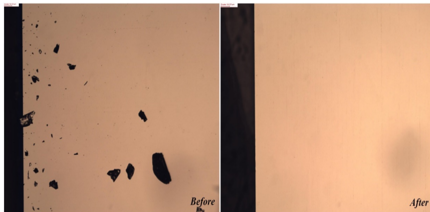
Figure 3.3.3 Results after cutting on the back side under the microscope
